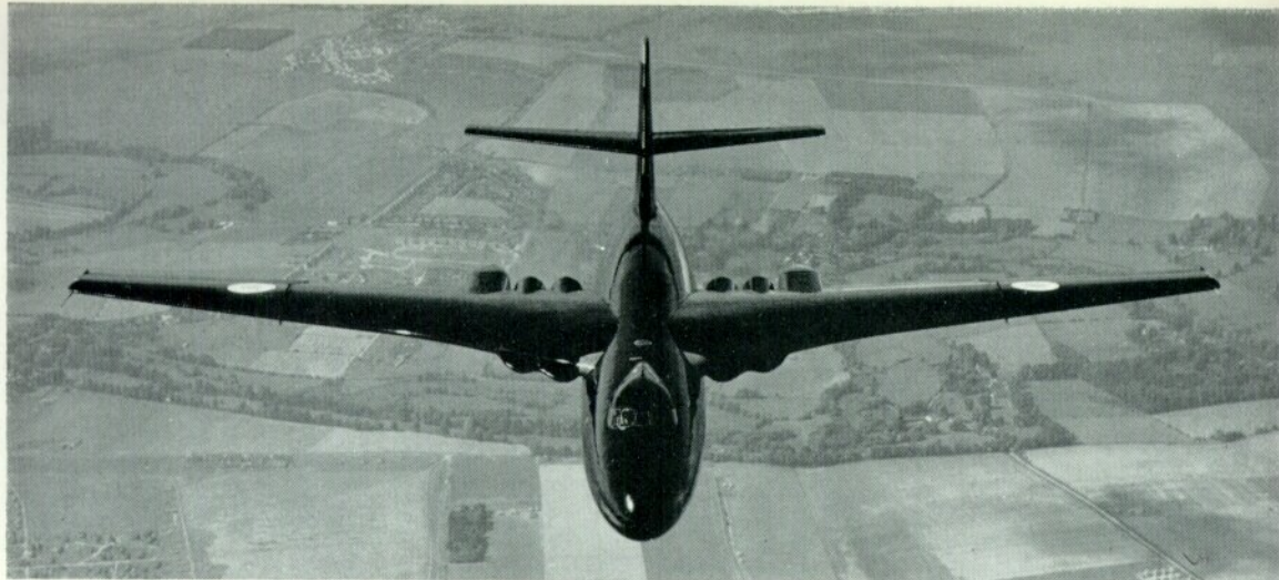
Sole example of the Valiant B.2 was WJ954. The B.2 had a lengthened nose and the main undercarriage legs retracted back into large fairings on the wing trailing edge. Overall finish was glossy black with white serial numbers.
