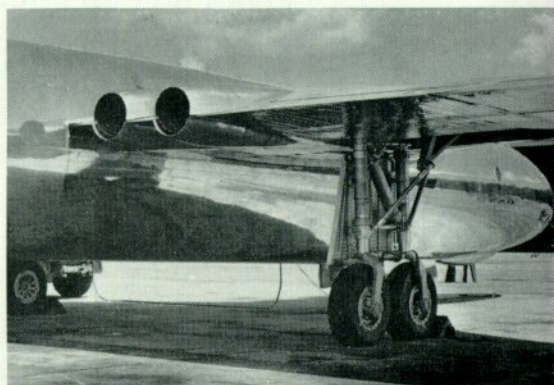
Close-up of prototype Valiant disclosing short jet pipes, later lengthened to improve the local airflow and fuel tank ventilation.
