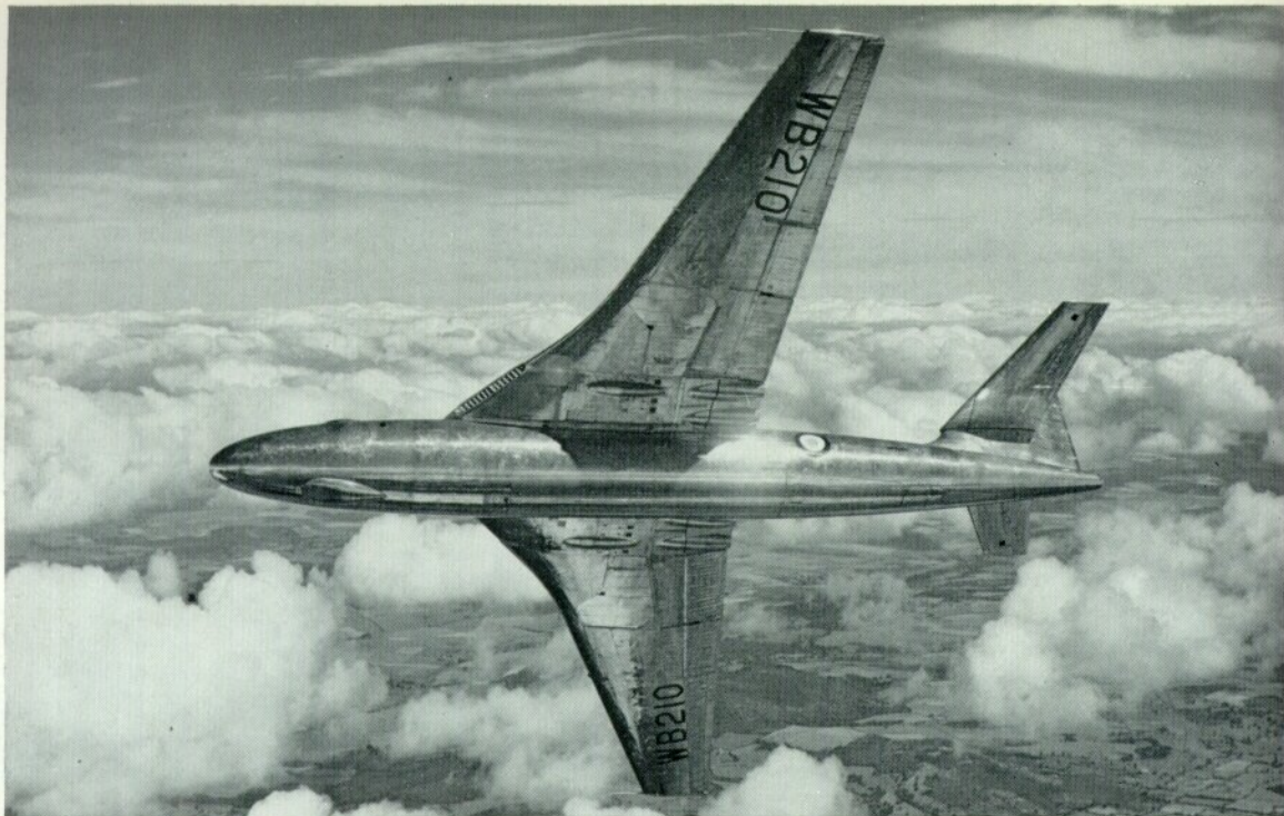
The prototype Valiant WB210 during initial test flight showing original straight slotted air intake with air flow straighteners in port leading edge wing root.
