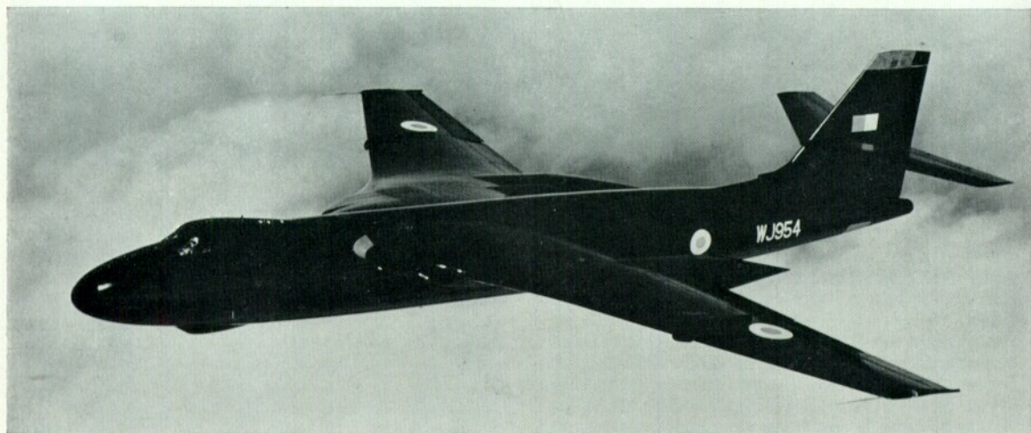
Sole example of the Valiant B.2 was WJ954. The B.2 had a lengthened nose and the main undercarriage legs retracted back into large fairings on the wing trailing edge. Overall finish was glossy black with white serial numbers.
