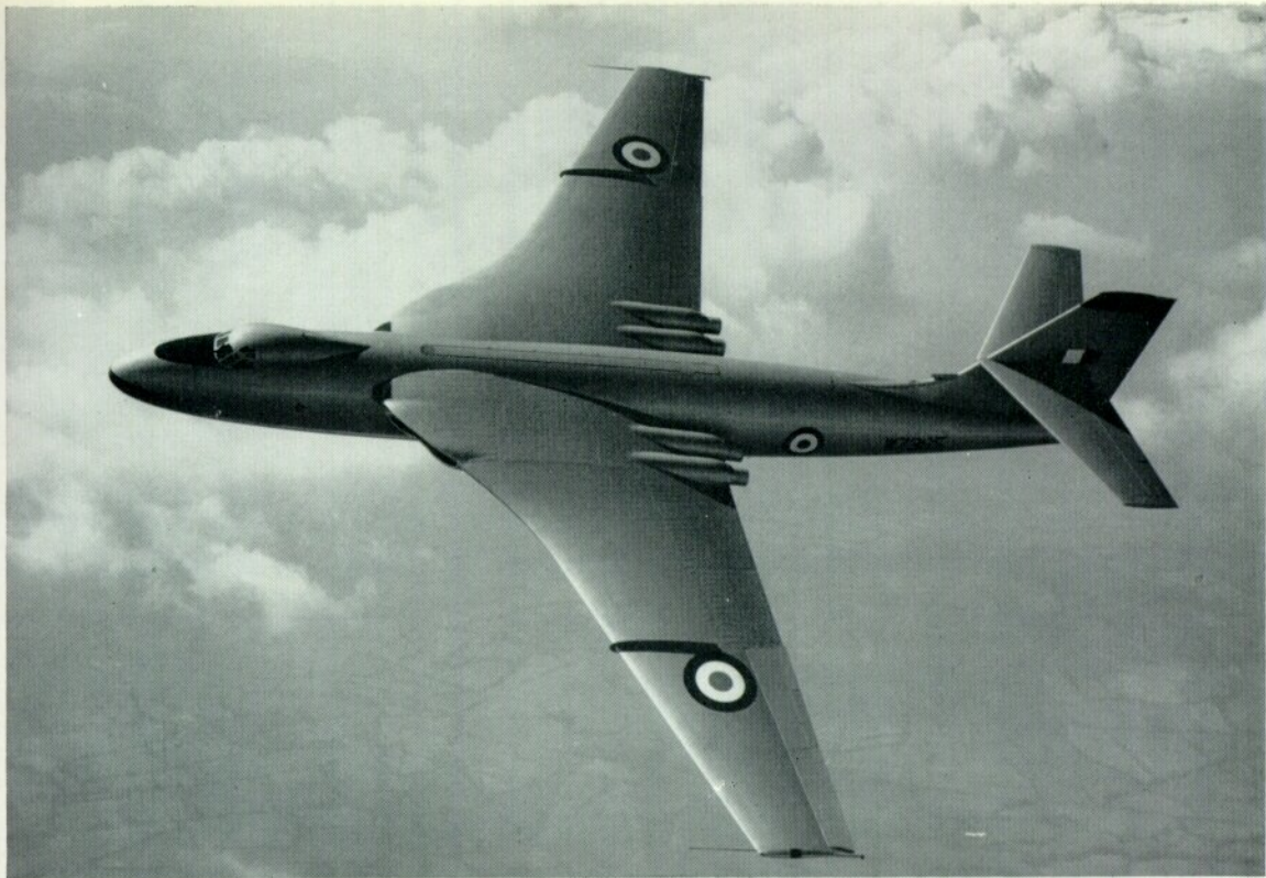
An early production Valiant (WZ365) in grey finish showing wing "fences" and protruding jet pipes.
