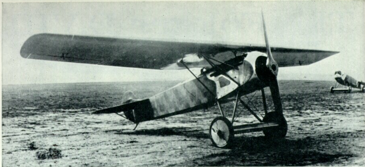
Third of the Fokker parasol monoplanes that participated in the first German fighter trials, the V.27 had a 195-h.p. Benz Bz.IIIb (Photo: via R. Ward)
