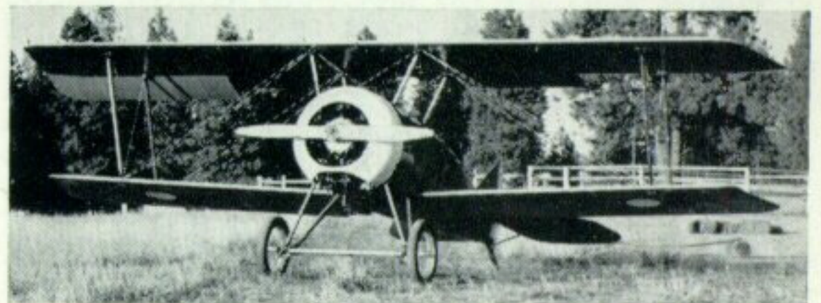
No. 38898 (now re-named Carlson S-4C) during final stages of rebuilding by Ed Carlson; rigging not complete. Powered by 120-h.p. Ken Royce radial. (Photos: Ed Carlson)
