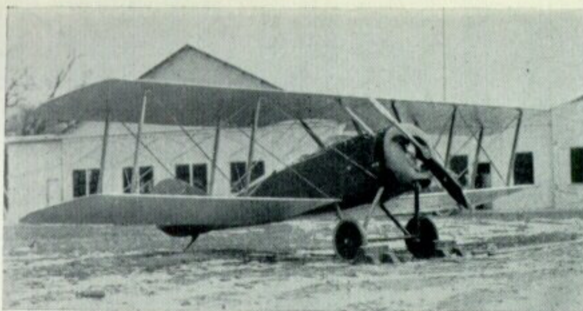
The S-7 side-by-side two-seat trainer, built and flown in twenty-nine days, January 1919. The only Thomas-Morse aircraft not designed by B. D. Thomas.
