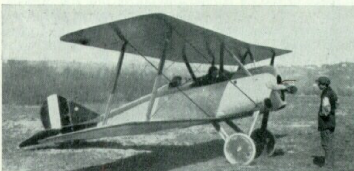
S-6, 80-h.p. Le Rhône. Only example of this tandem-seat trainer built. (Photo: G. Baumwart)
