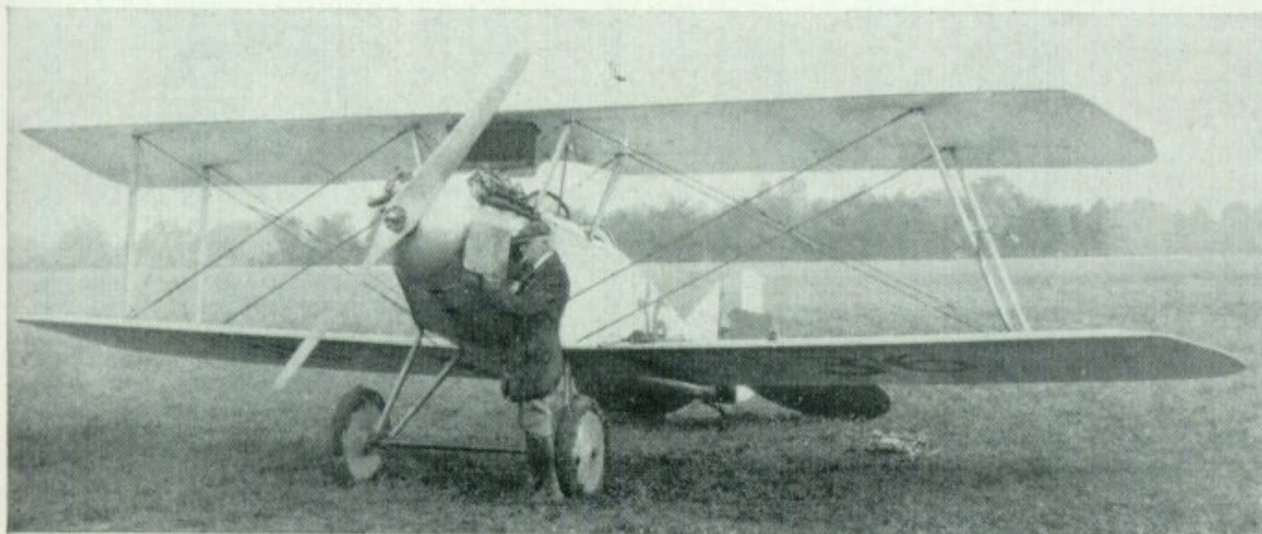
Yackey "Sport" flown by W. D. Addems (seen in photo) in 1925 Ford Reliability Tour. Basically an S-4C converted to two-seater, with 90-h.p. OX5 engine, four upper wing panels, lower ailerons sealed over. (Photo: Ford Motor Co.)
