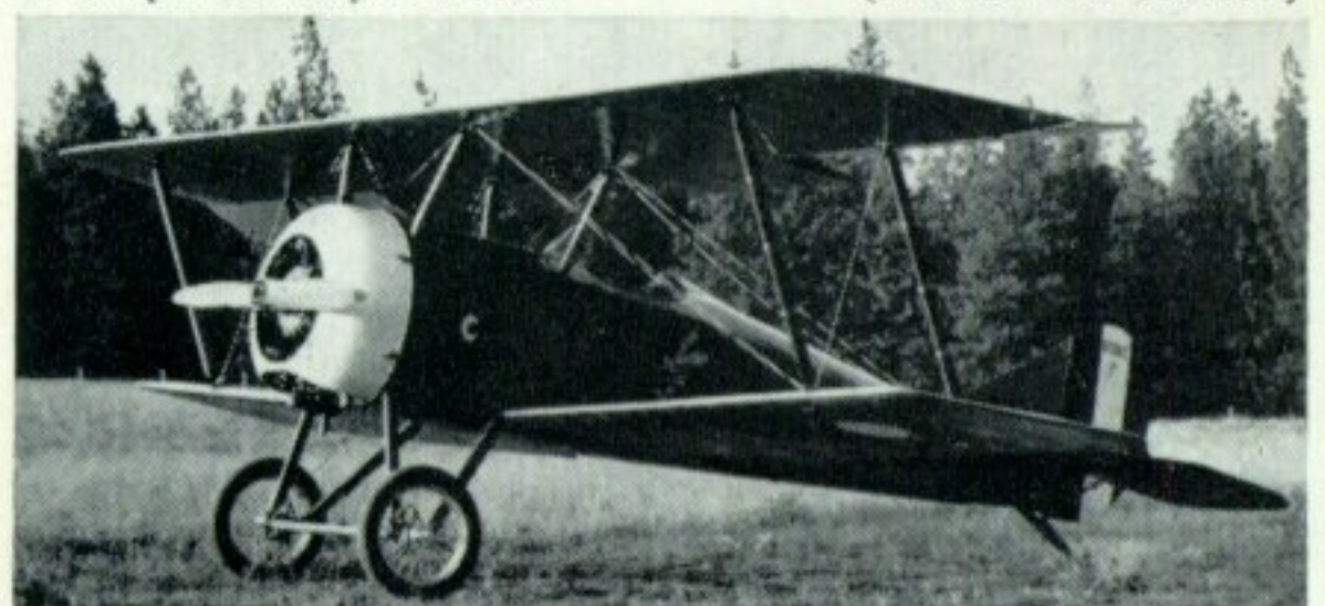
No. 38898 (now re-named Carlson S-4C) during final stages of rebuilding by Ed Carlson; rigging not complete. Powered by 120-h.p. Ken Royce radial. (Photos: Ed Carlson)
