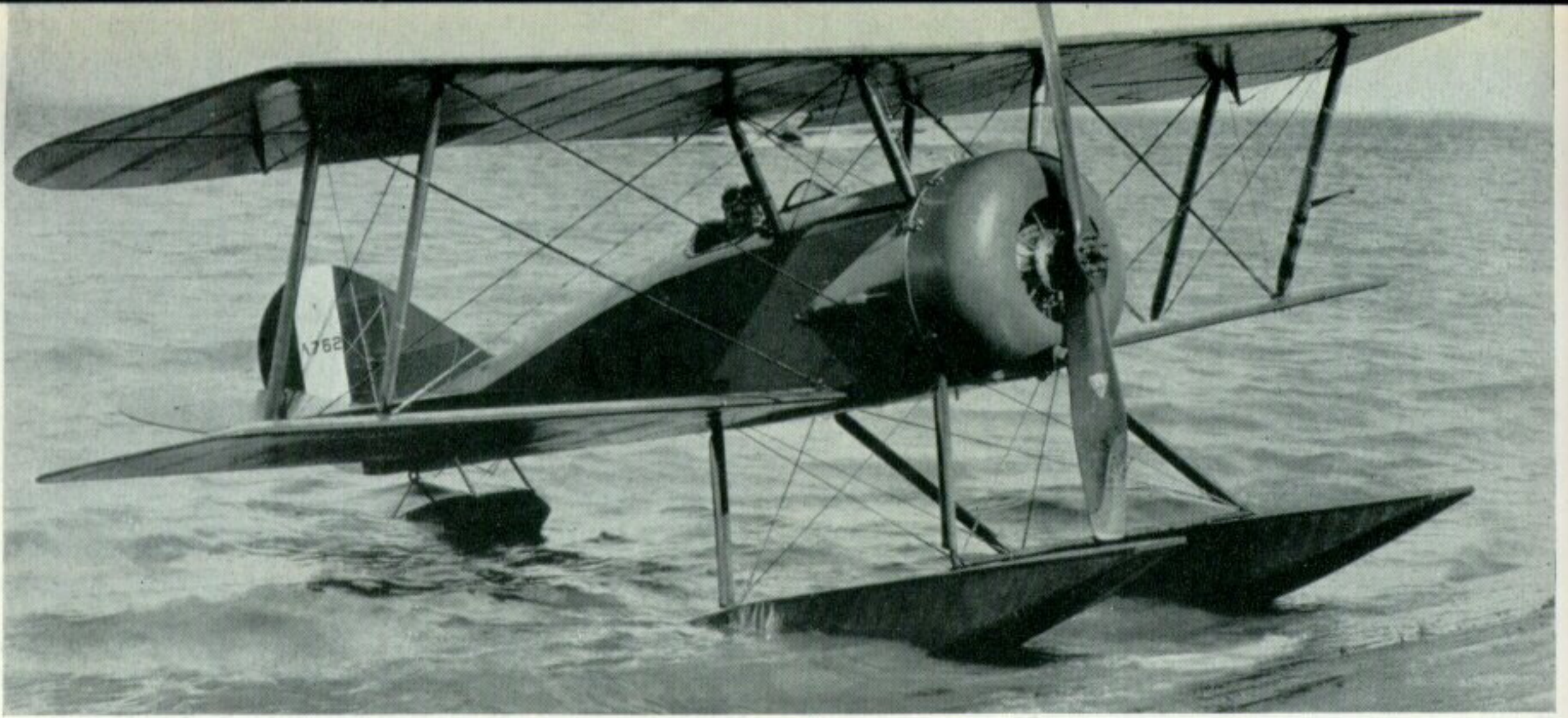
S-5 floatplane, 100-h.p. Gnome rotary, U.S.N. serial A-762, photographed June 1918 at Dinner Key N.A.S., Florida. (Photo: U.S.N. official)
