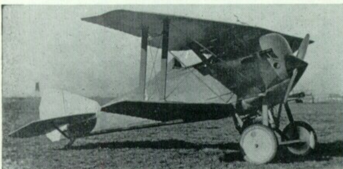
Left: S-4E racer, 135-h.p. Aeromarine engine, photographed in 1925. Carried the legend "Space Eater" below the cockpit. (Photo: U.S. Navy). Right: S-4E, 110-h.p. Le Rhône; last of the single-seat S-4 scouts. (Photo: T-M. Aircraft Corp.)
