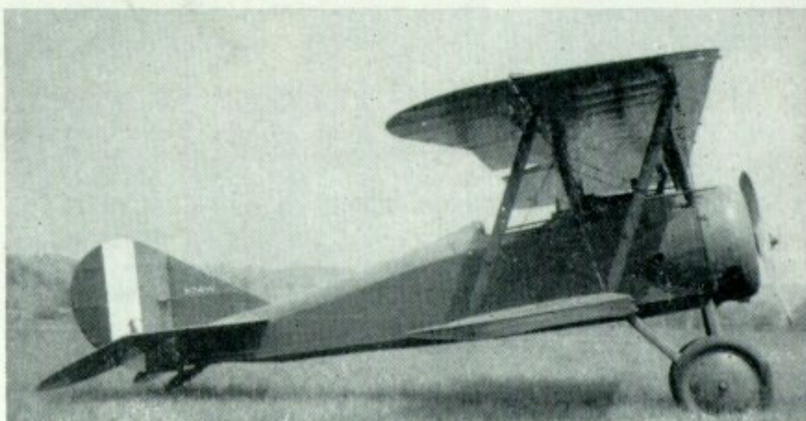
S-4B No. 153, the only surviving example, owned by the late D. B. Woodward and now on loan to the U.S.A.F. museum, Dayton, Ohio. A machine gun has been added, and original 100 h.p. Gnome has been replaced by 80 h.p. Le Rhône. (Photo: Logan Coombs)
