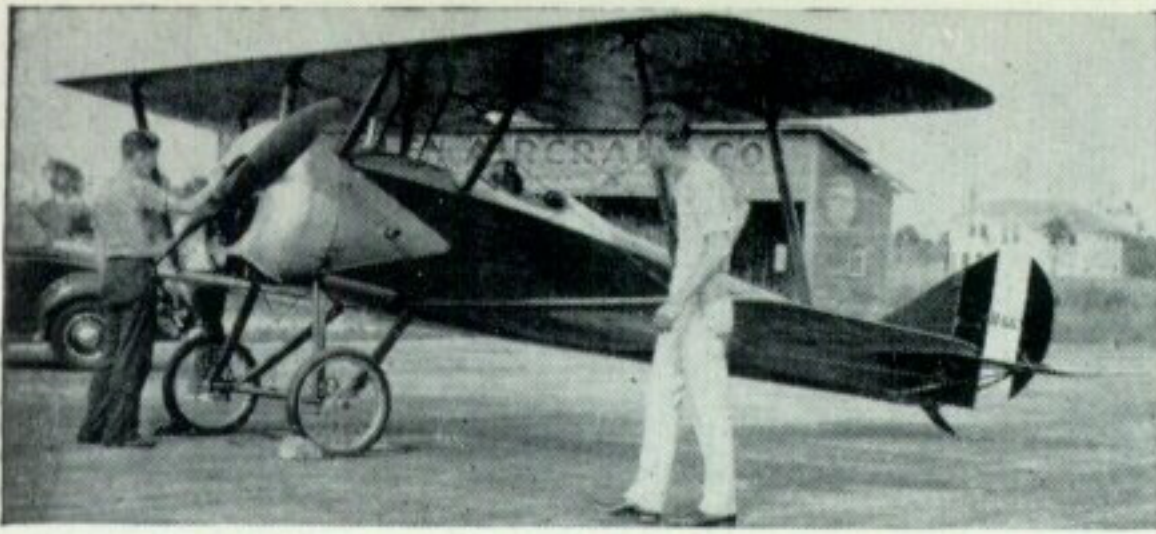
Left: S-4C formerly owned by Jack Walton of Tampa, Fla., photographed in 1937. This is probably the prototype S-4 with S-4C wings and Le Rhône engine; the fuselage is longer than the standard S-4C. (Photo: Jack Walton). Right: The first Tommy with Le Rhône engine, S-4C 38633, photographed at Taliaferro Field, Hicks, Texas. Note field modification of box for expended cartridge cases, and rudder from different aircraft, 38651. (Photo: Air Force Museum)
