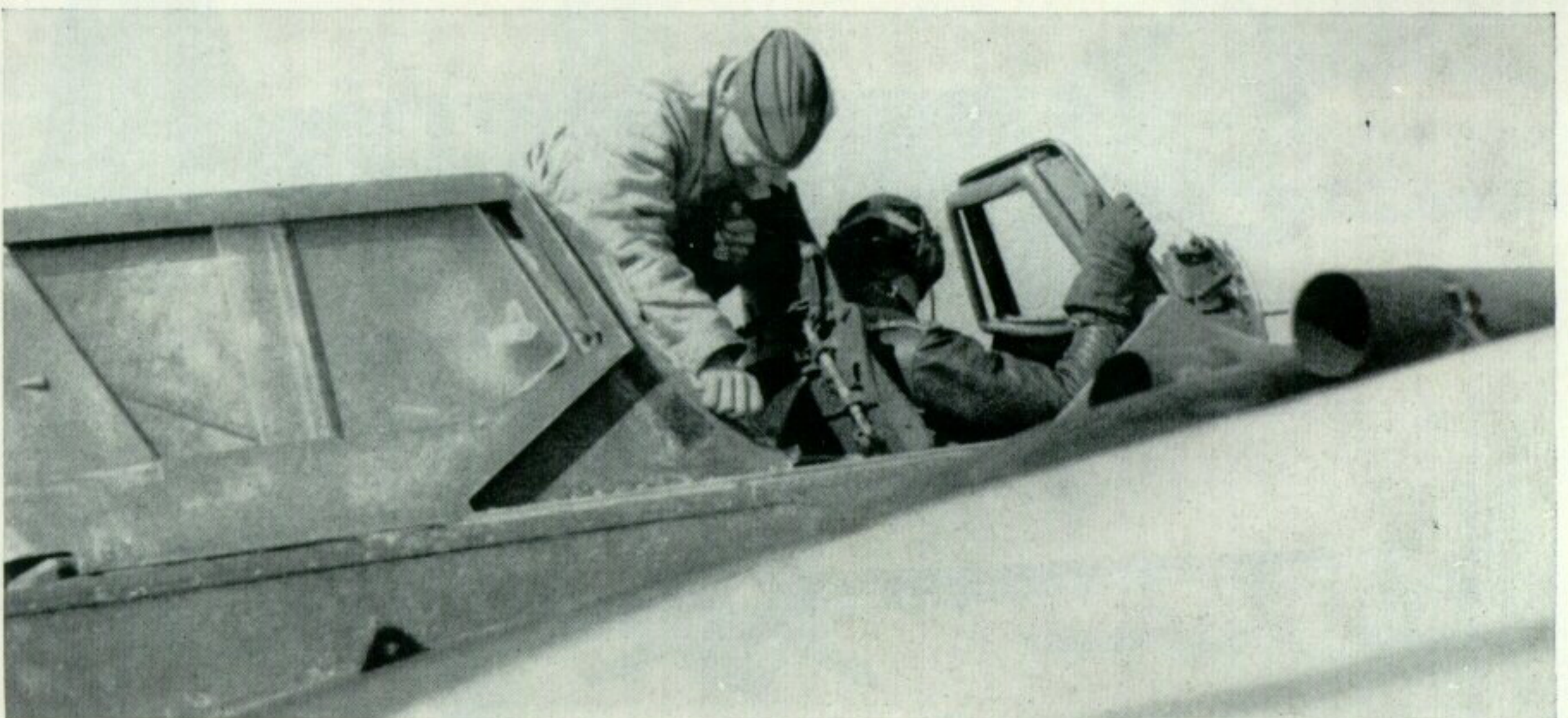
A Henschel pilot prepares for a sortie in Russia. Note the massive construction of the cockpit, a self-contained unit composed almost entirely of armour plate. (Photo: R. C. Seeley collection)
