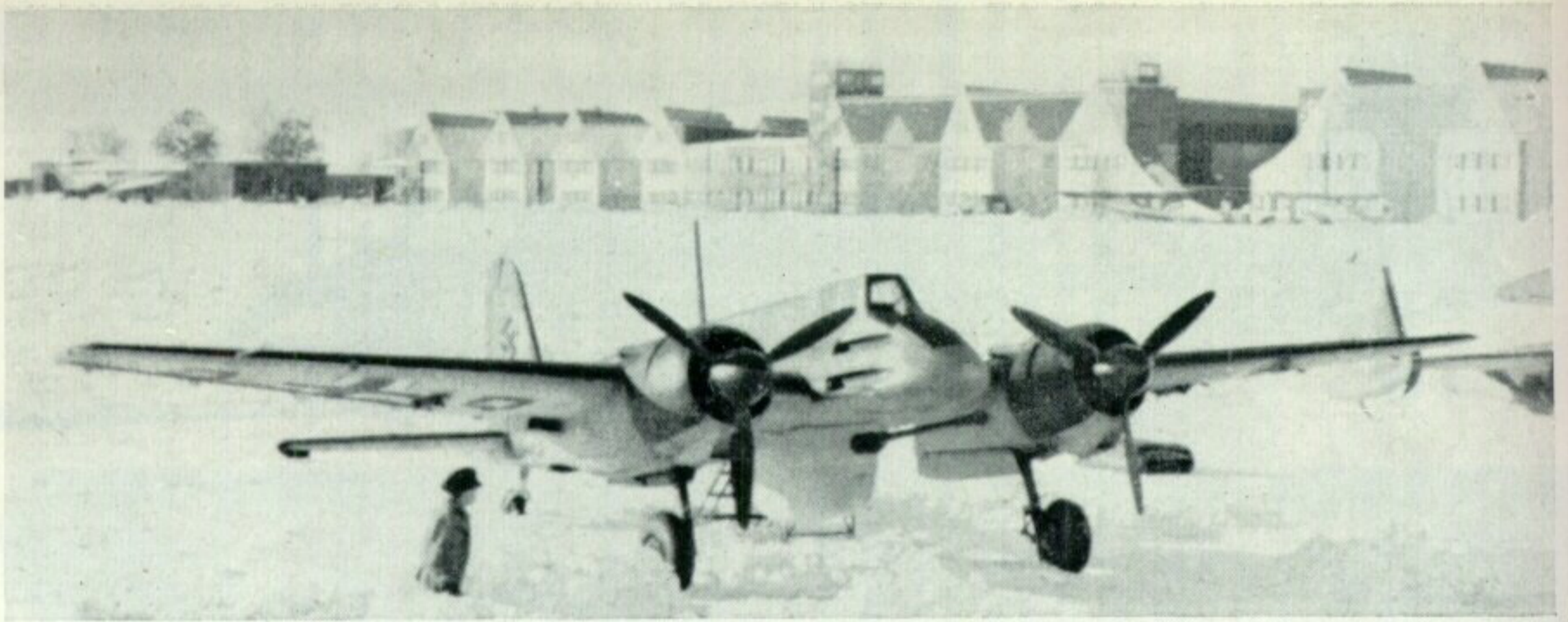
Hs 129B-2 with test installation, probably of BK 5 cannon. This machine is believed to have been photographed at the Travemünde experimental establishment; note hangars camouflaged as private houses in background. (Photo: R. C. Seeley collection)
