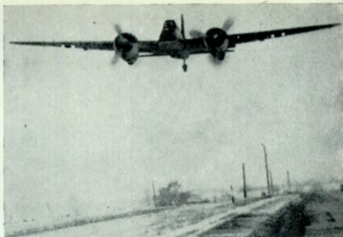
The Hs 129B-0 appeared late in 1940; the Gnome Rhône 14 M engines offered better power and the variant displayed superior handling characteristics to the A-0.
