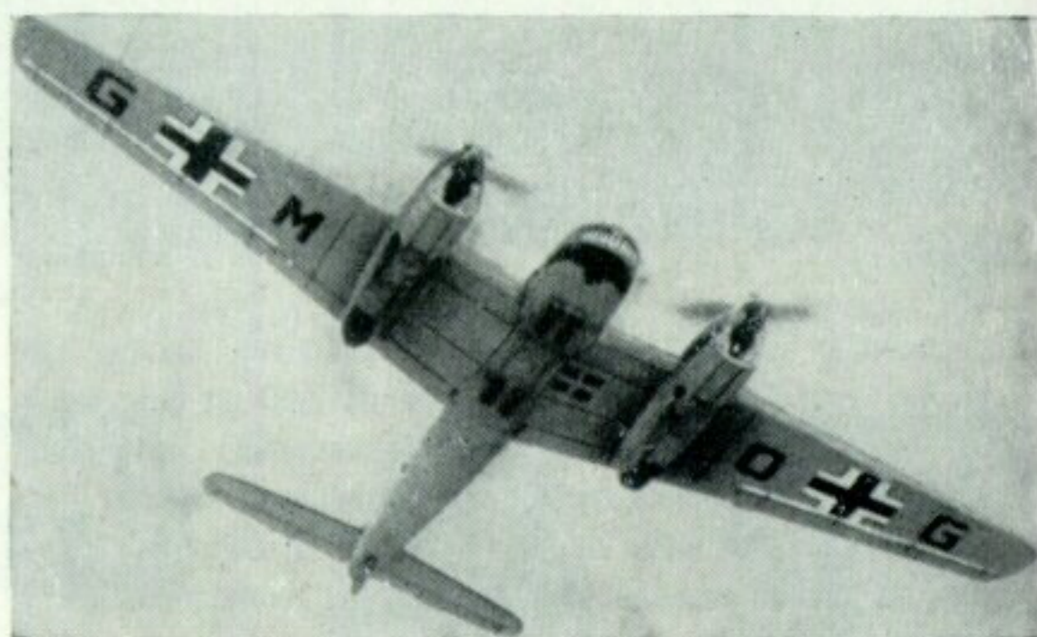
Another flying view of the Hs 129A-0 shows the fuselage bomb racks.
