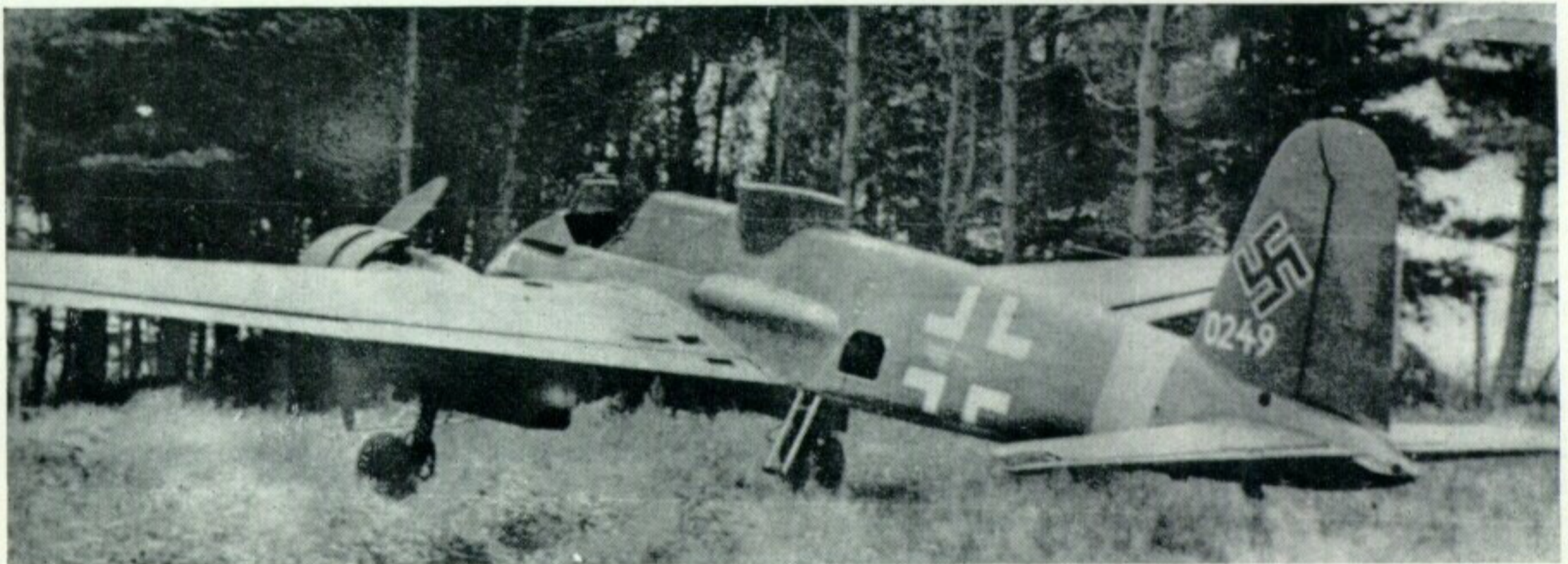
W. Nr. 0249, one of the three B-2 models experimentally fitted with the 77-mm. SG 113A recoil-less rocket mortar. The rhomboid-shaped mounting can be seen protruding from the fuselage spine. (Photo: Gruppe 66 Archives)
