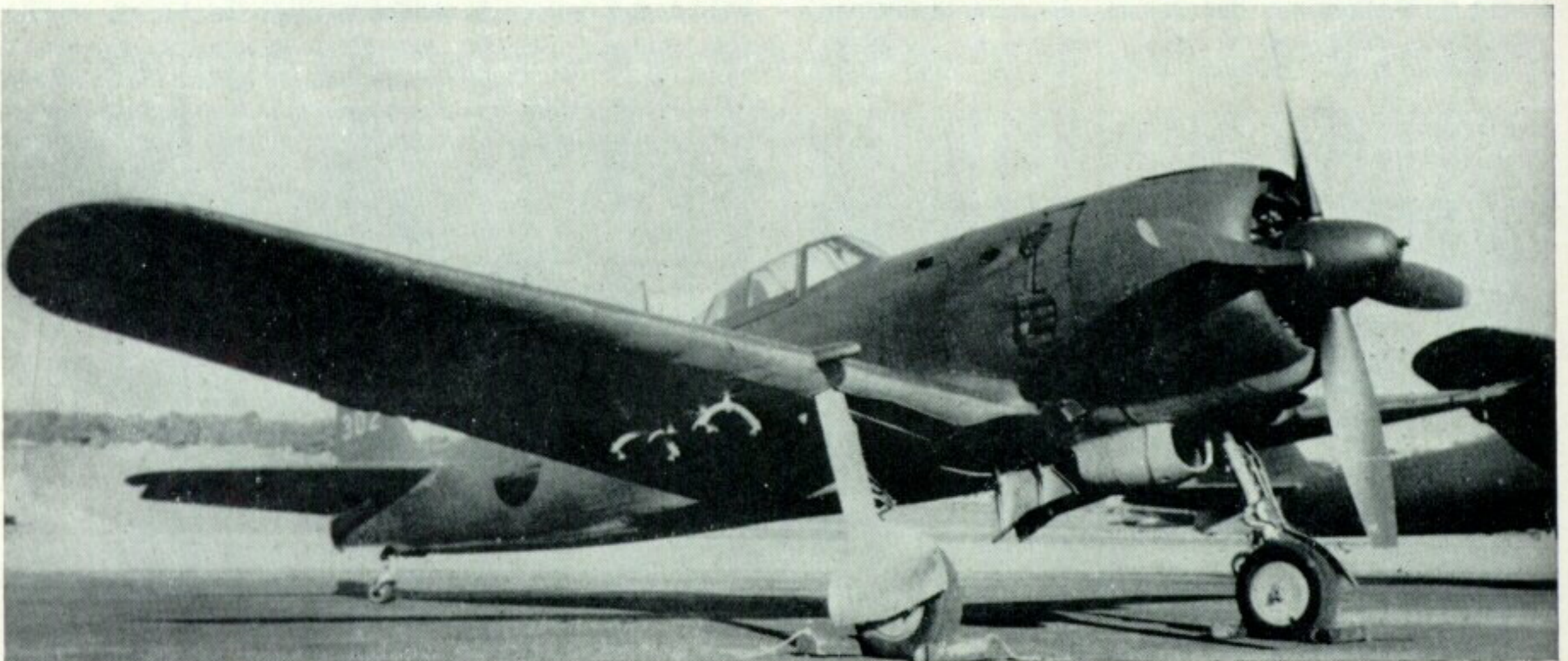
Three views of a Ki-84-Ia in test livery. The cannons in the wings are the standard 20-mm. Ho-5 weapons, faired for trial purposes. (Photos: Witold Liss, The Australian War Memorial, H. Nowarra)
