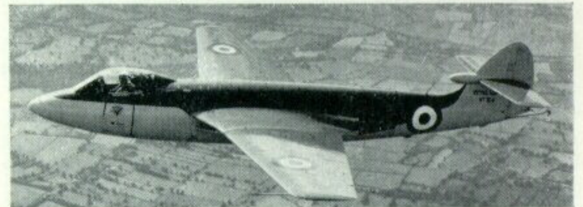
Introduced during the initial production run at Hawkers was the bullet fairing on the tailplane seen here on WF159.
