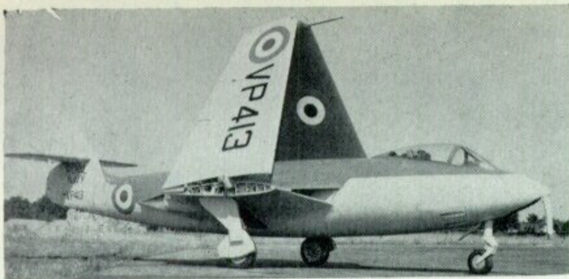
First of the N.7/46 prototypes, VP413 demonstrates (above) the method of wing folding and (below) the ample area of wing flap and airbrake of the Sea Hawk. (Photos: above, Cyril Peckham; below, Ministry of Defence, Neg. No. 16963D)
