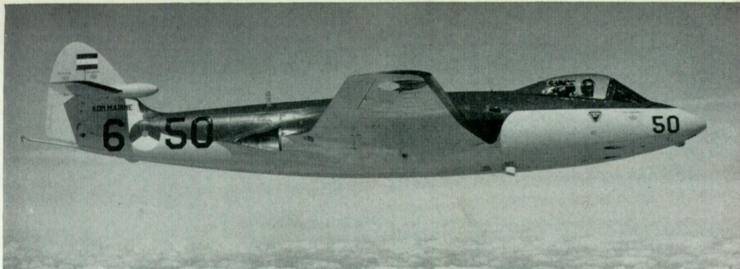
Netherlands Sea Hawk Mk. 50. Main external difference from the F.G.A. Mk. 6 lay in the blade aerial for Philips UHF radio—standard equipment among some NATO air forces. (Photo: Sir W. G. Armstrong Whitworth Aircraft Ltd., Neg. No. A976)
