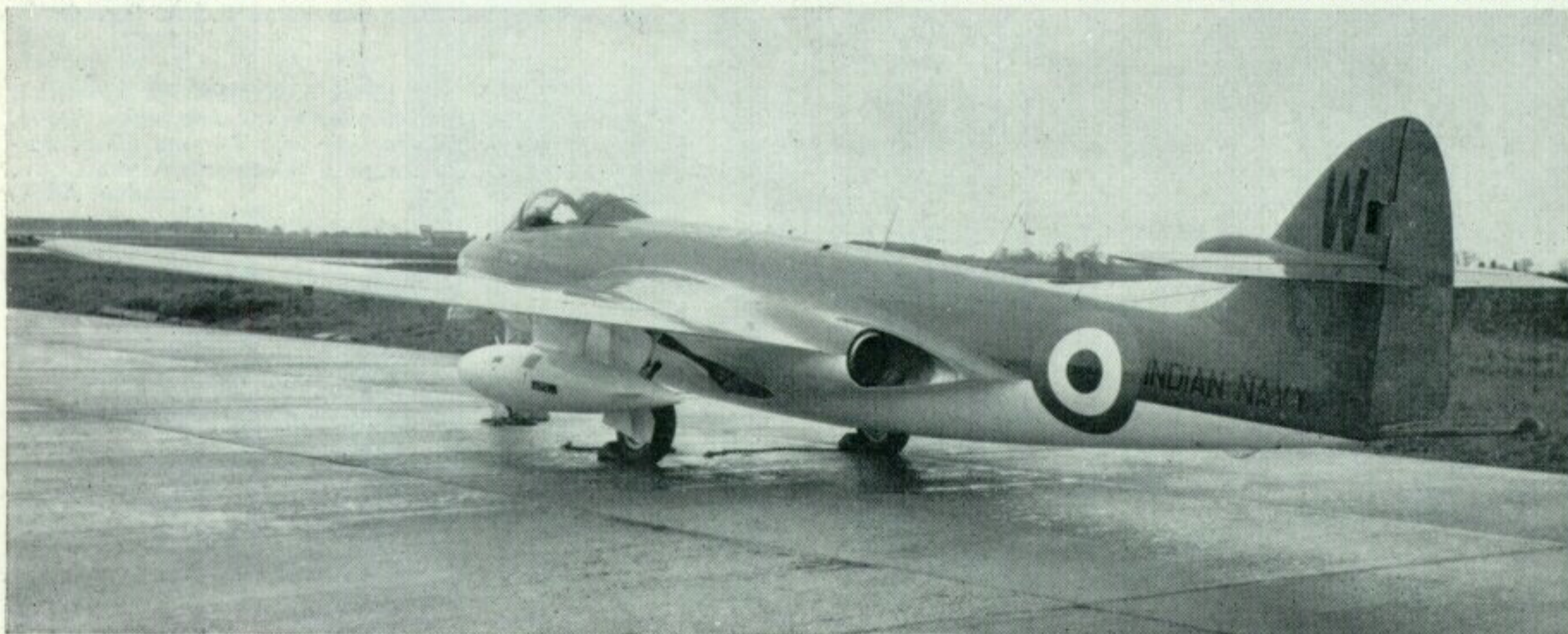
One of the relatively few photos available of the Indian Sea Hawk Mk. 6. The serial number, IN151, appeared in small black characters on the fin just below the tailplane. (Photo: Sir W. G. Armstrong Whitworth Aircraft Ltd., Neg. No. A1107)
