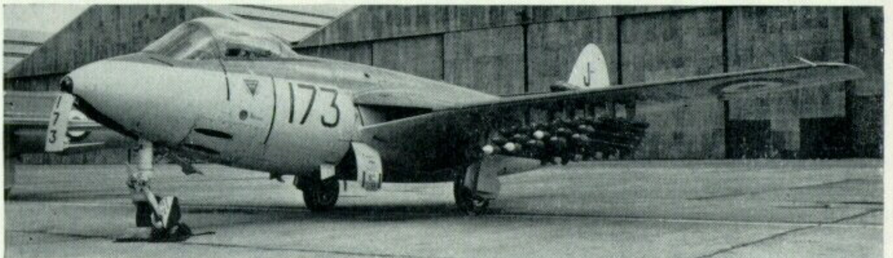
A Sea Hawk F.G.A. Mk. 4 armed with thirty 3-in. rocket projectiles with 25-lb. warheads. (Photo: Sir W. G. Armstrong Whitworth Aircraft Ltd., Neg. No. A810)
