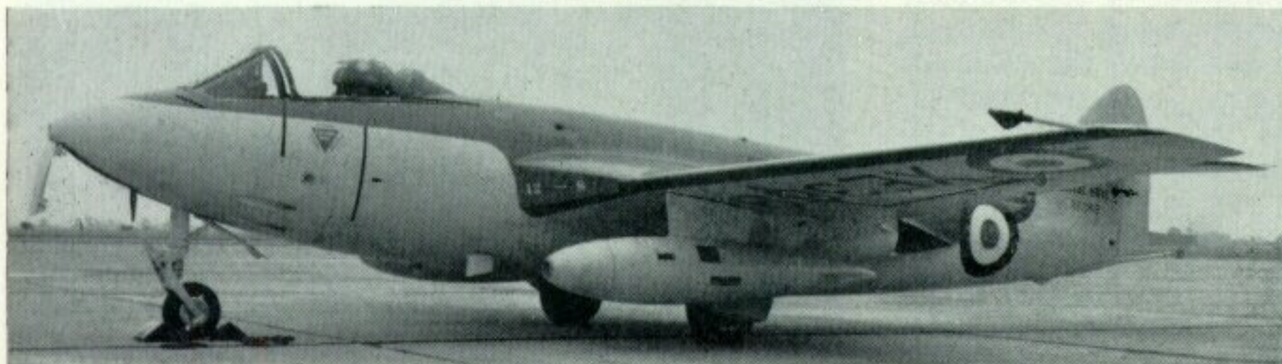
Sea Hawk Mk. 6 XE369 was used by A.W.A. for various trial installations; here it is seen with forward-facing F.95 low-level cameras mounted in the nose of an underwing drop tank. (Photo: Sir W. G. Armstrong Whitworth Aircraft Ltd., Neg. No. A835)
