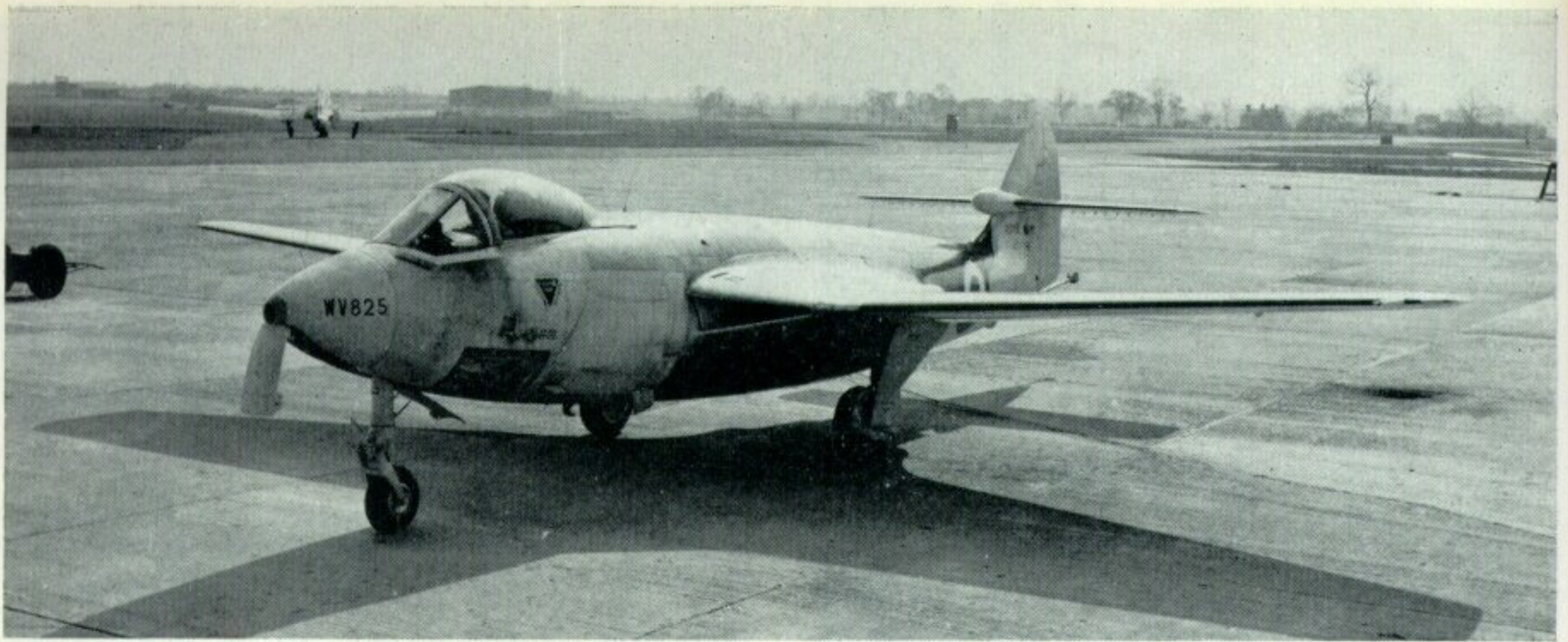
The Sea Hawk Mk. 4, WV825, used for trials with powered elevators, identifiable by the vortex generators on the tailplane. (Photo: Sir W. G. Armstrong Whitworth Aircraft Ltd., Neg. No. A675)
