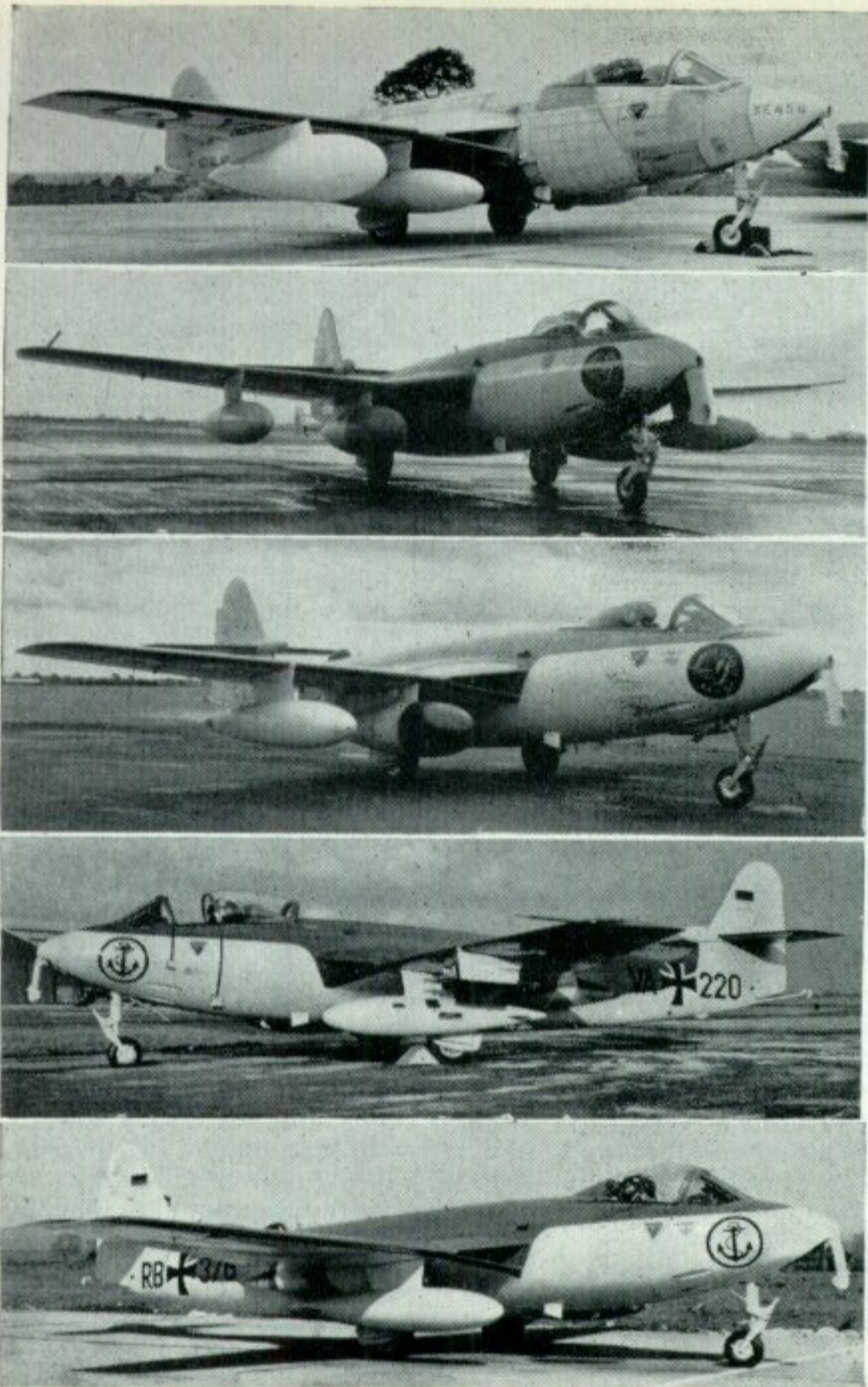
Development of the German Sea Hawks. Top to bottom: XE456 with early mock-up of Ekco radar outboard under wing. XE456 with later mock-up under inboard pylon; just visible is the instrumentation boom under the rudder (in place of arrester hook), and yaw meter on starboard wing tip to measure effect of increased fin area. Third photo shows XE456 equipped with prototype flight installation of Ekco radar and radome on rear fuselage: the standard arrester hook has been refitted. Fourth photo shows standard Sea Hawk Mk. 100 equipped with four wing pylons, four R.P. mountings and search radar sight-head. The bottom photo is of a German Sea Hawk Mk. 101 with Philips UHF radio (note blade aerial forward of rear fuselage radome). (Photos: Sir W. G. Armstrong Whitworth Aircraft Ltd., Neg. Nos. A826, A893, A954, A1046 and A1085)
