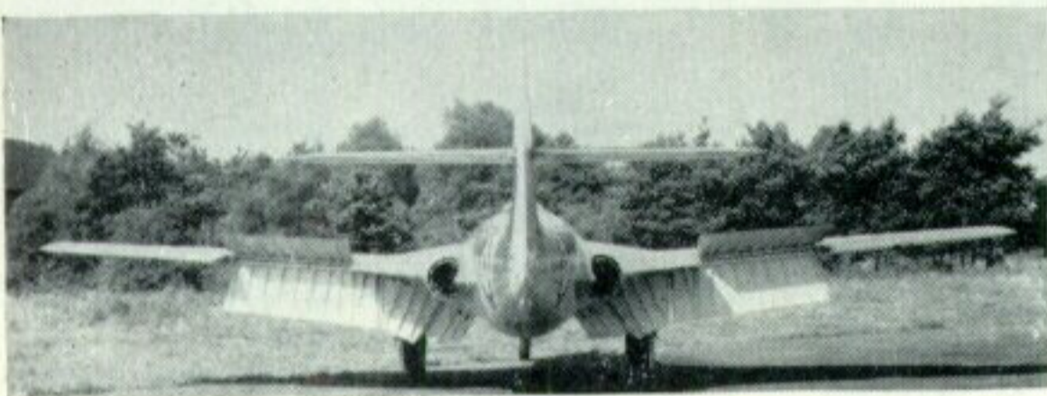
First of the N.7/46 prototypes, VP413 demonstrates (above) the method of wing folding and (below) the ample area of wing flap and airbrake of the Sea Hawk. (Photos: above, Cyril Peckham; below, Ministry of Defence, Neg. No. 16963D)
