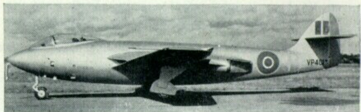
The Hawker P.1040, VP401, in its original configuration with rectangular heat shield fairings aft of the jet pipes. Photo taken immediately after arrival at Farnborough in September 1947. (Photo: Ministry of Defence, Neg. No. 16274C)
