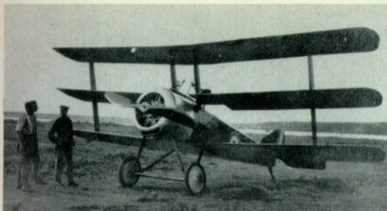
Another two-gun triplane, this aircraft had a Lewis gun in addition to its standard single Vickers.
