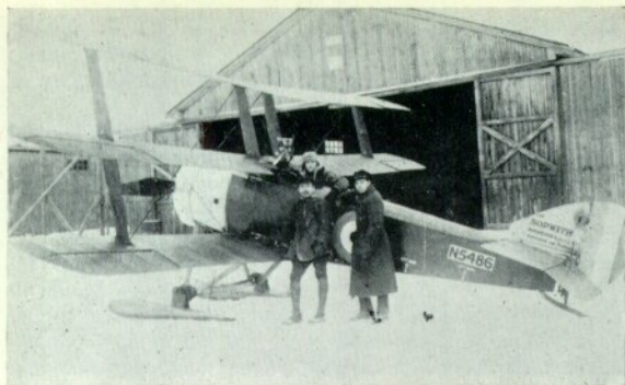
N5486, with ski undercarriage, which served with the Imperial Russian Air Service in 1917-18.
