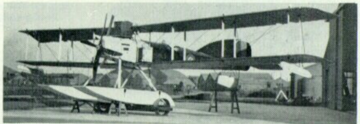
This Type D is No. 9048, built by Robey and powered by a 240-h.p. Sunbeam Gurkha driving a four-blade airscrew. Like No. 8359, it had a stack-type exhaust pipe.
