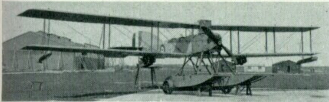
No. 8052 with two 65-lb. bombs under each lower wing. This was an early attempt to fit bomb racks to the Short 184 but was abandoned in favour of the under-fuselage bomb rail. This Short still had arched float cross-bars when this photograph was made.
