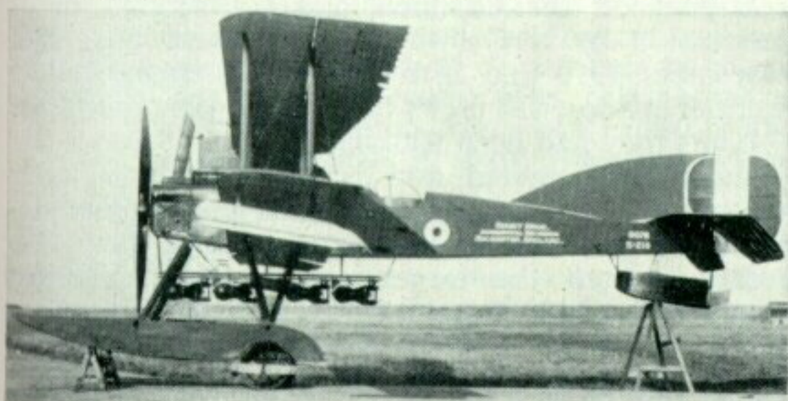
No. 8076 at the Isle of Grain with Whitehouse gun mounting on the rear cockpit and four 100-lb. bombs. This aircraft had a 260-h.p. Maori I or II driving a two-blade airscrew.
