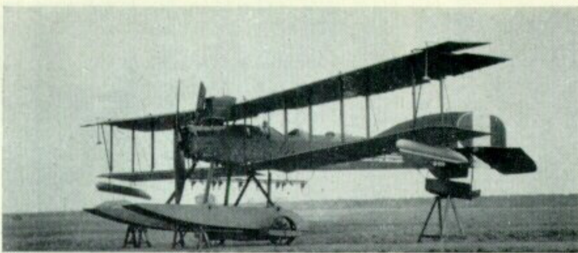
No. 8076 at the Isle of Grain, fitted with Martin stabilisers on the upper wings, 5th November 1917.
