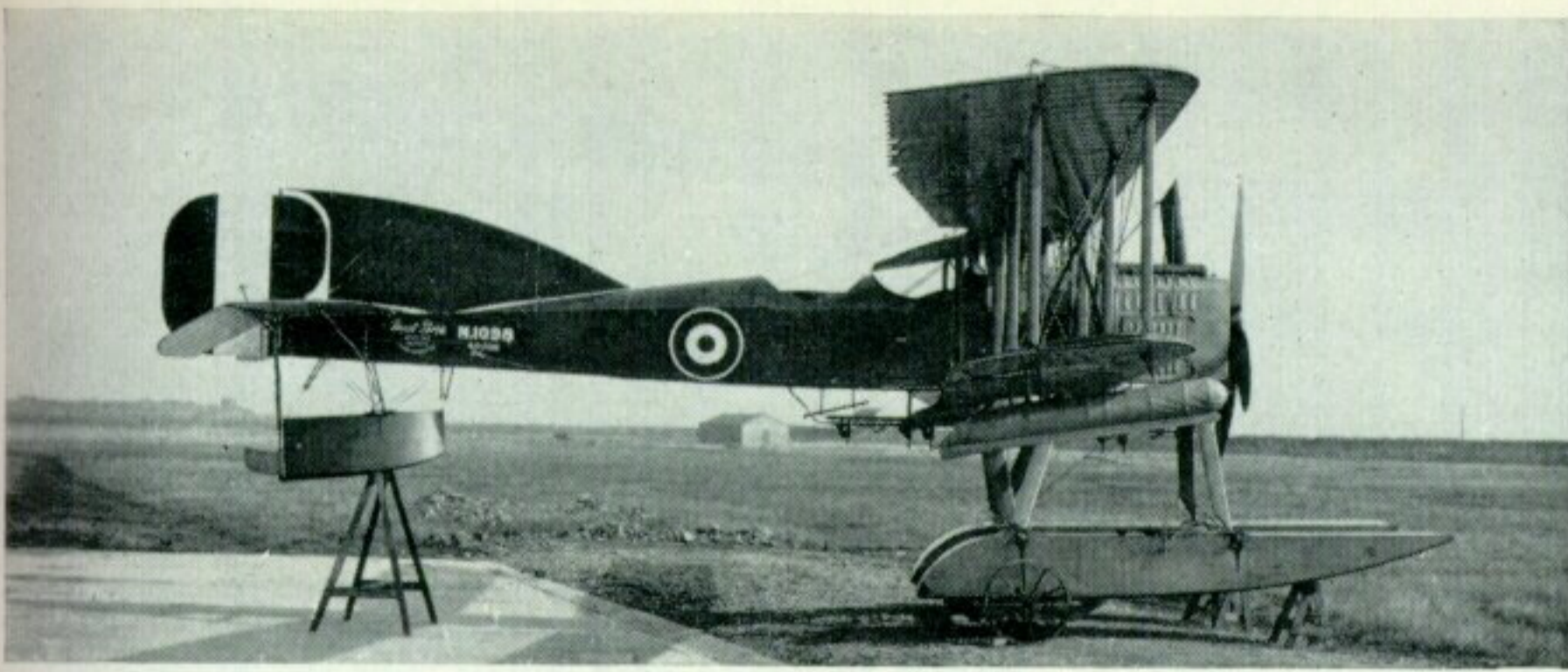
N1098 at the Isle of Grain, October 1917, with square frontal radiator on its Maori engine. This aircraft, although not originally built as an Improved 184, had the revised aileron system at the time when this photograph was made; it also had the longer tail-float struts.
