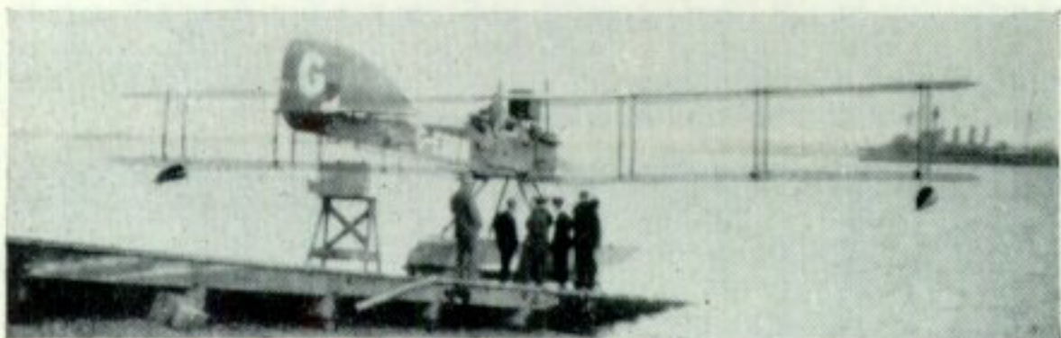
One of the five Short 184s that came on to the British civil register, G-EBBN was originally N9118; it was powered by a Maori III.
