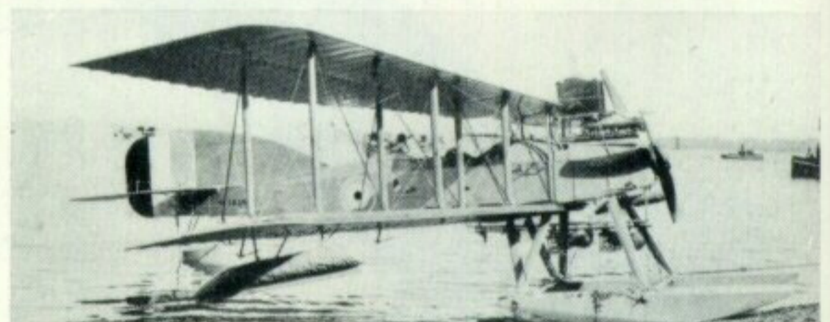
Left: The installation of the 240-h.p. Sunbeam Gurkha in No. 8014 did not differ externally from that of the 225-h.p. engine. The aircraft is seen at Grain on 9th December 1916, fitted with the underslung bomb rail with racks for four bombs. (Photo: Imperial War Museum MH2869.) Right: The Dover-type Renault installation with central elevated radiator, here exemplified on Short 184 N1616 built by Saunders.
