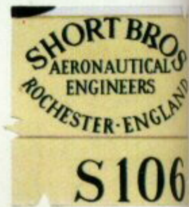
Manufacturer's plate displayed both sides of rudder (port shown) of S.106 illustrated above.
