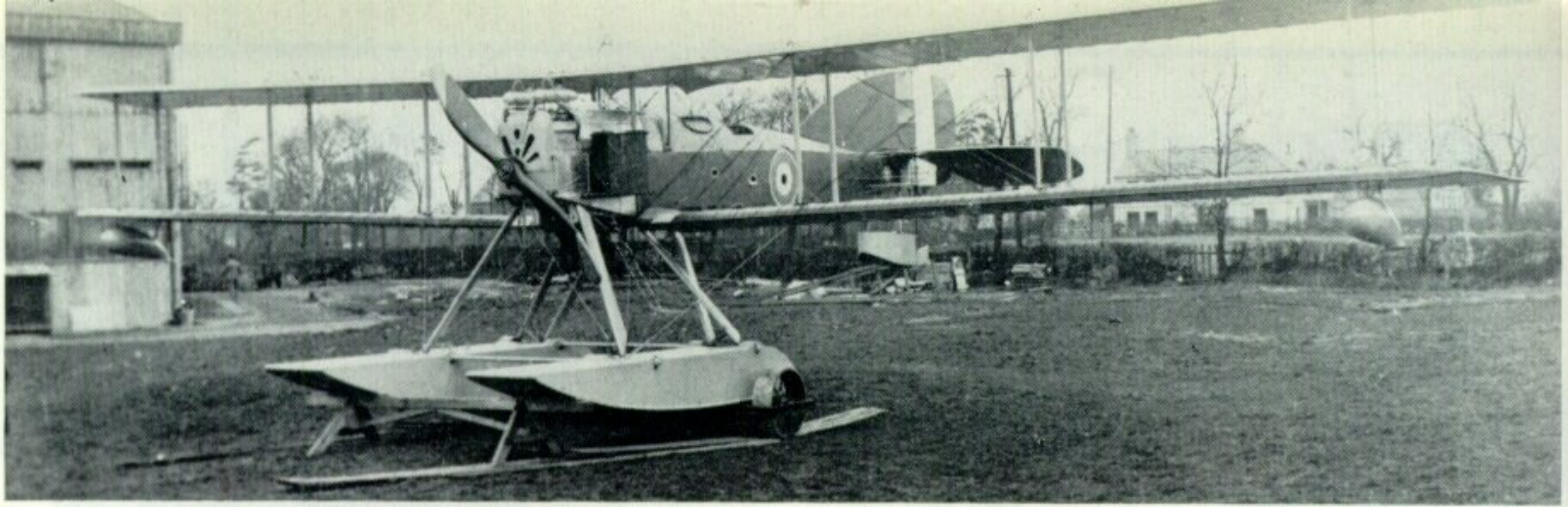
Sage-built Short Improved 184 powered by the 240-h.p. Renault engine with the original installation that embodied two flank-mounted radiators. This aircraft also has the later type of wing-tip floats.
