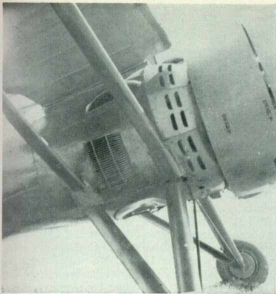
Details of the P-11c: (above) Cowling (note jettisonable fuel tank visible on underside of fuselage); (right) Main undercarriage gear. Photos: via the author.
