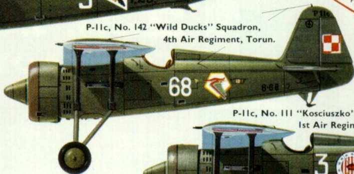
P-11c, 500 h.p. Gnome-Rhone 9 Krse. Mistral radial engine. Salon International d'Aeronautique, Paris.
