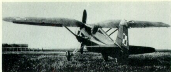
Standard production P-11c, with four-gun armament.
