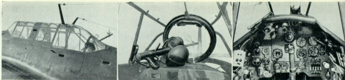
Left to right: Gunner's position in Ju 87 A; MG 15 gun position of a Ju 87 B-1; Ju 87 B-1 instrument panel.
