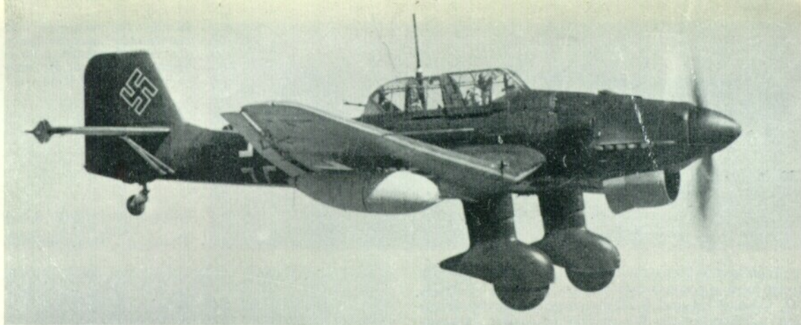
The Ju 87 R was basically a B-model with enlarged wing fuel cells and underwing tanks. They were employed extensively by the Stukaverbände, as range was almost doubled.
