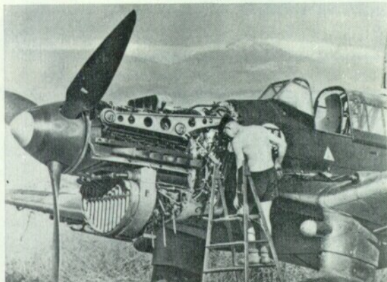
Jumo 211 Da powerplant of a Ju 87 B-2 with cowling removed. Note also contoured armour back-shield in cockpit.
