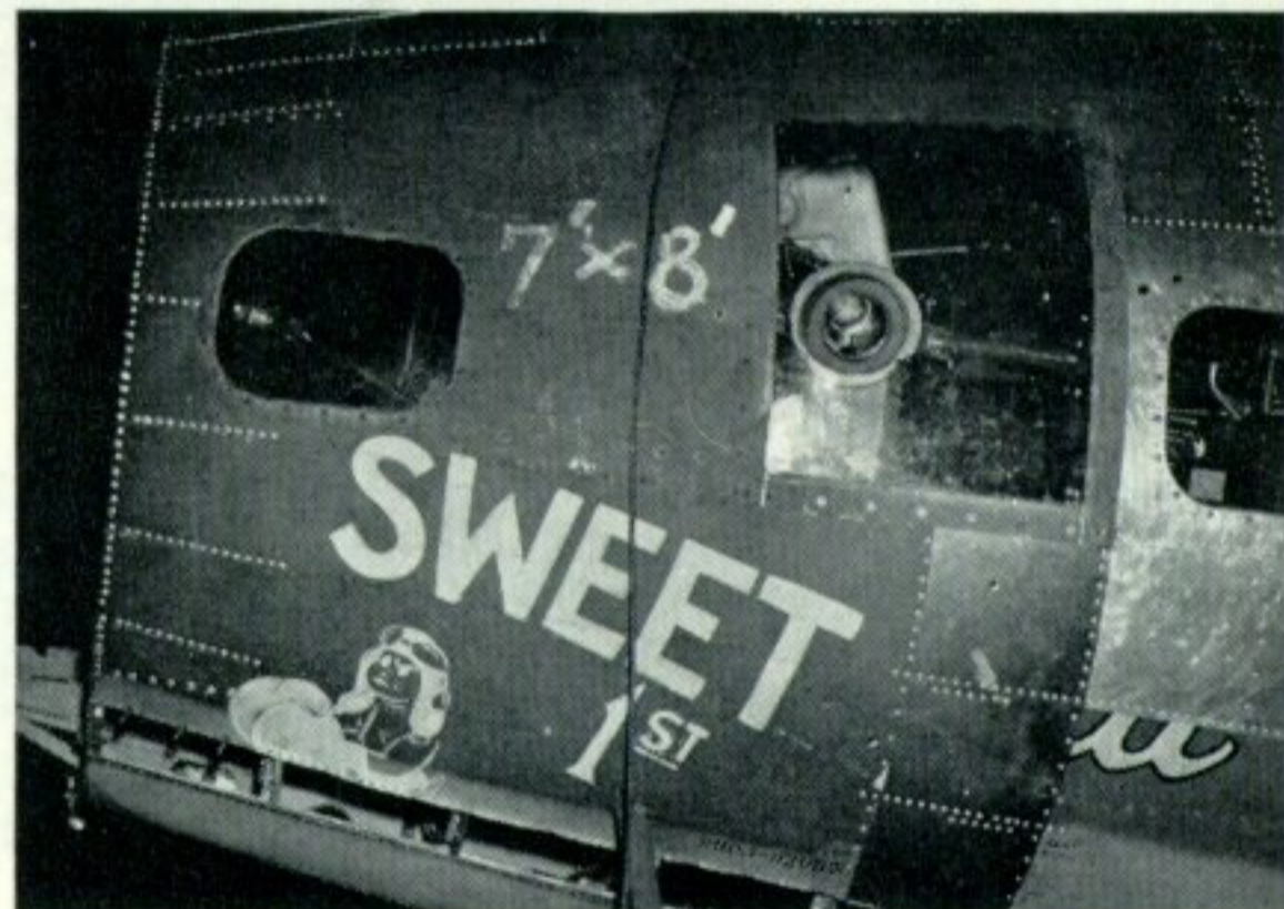
This unusual sequence graphically demonstrates the "repairability" of the Fortress. Top left shows "Eight Ball", a B-17F-25-DL (DO) of the 91st B.G., serial 42-3138, with nose damage from a runaway propeller. The area to be replaced is marked off with masking tape. Top right shows the section removed, with the replacement nose from "Sweet Pea 1st" ready. Bottom left shows the section in place. Bottom right shows job almost complete. (Photos: W. J. Connell collection)
