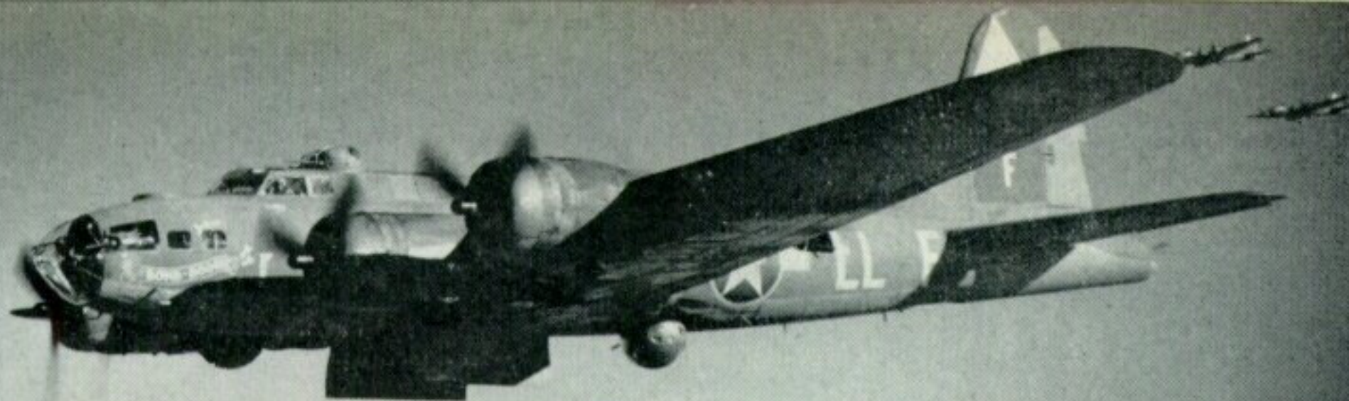
A late model B-17F "Bomb Boogie" of the 401st B.S., 91st B.G. with modified cheek gun position which allows .50 to fire directly forward. (Photo: U.S.A.F.)
