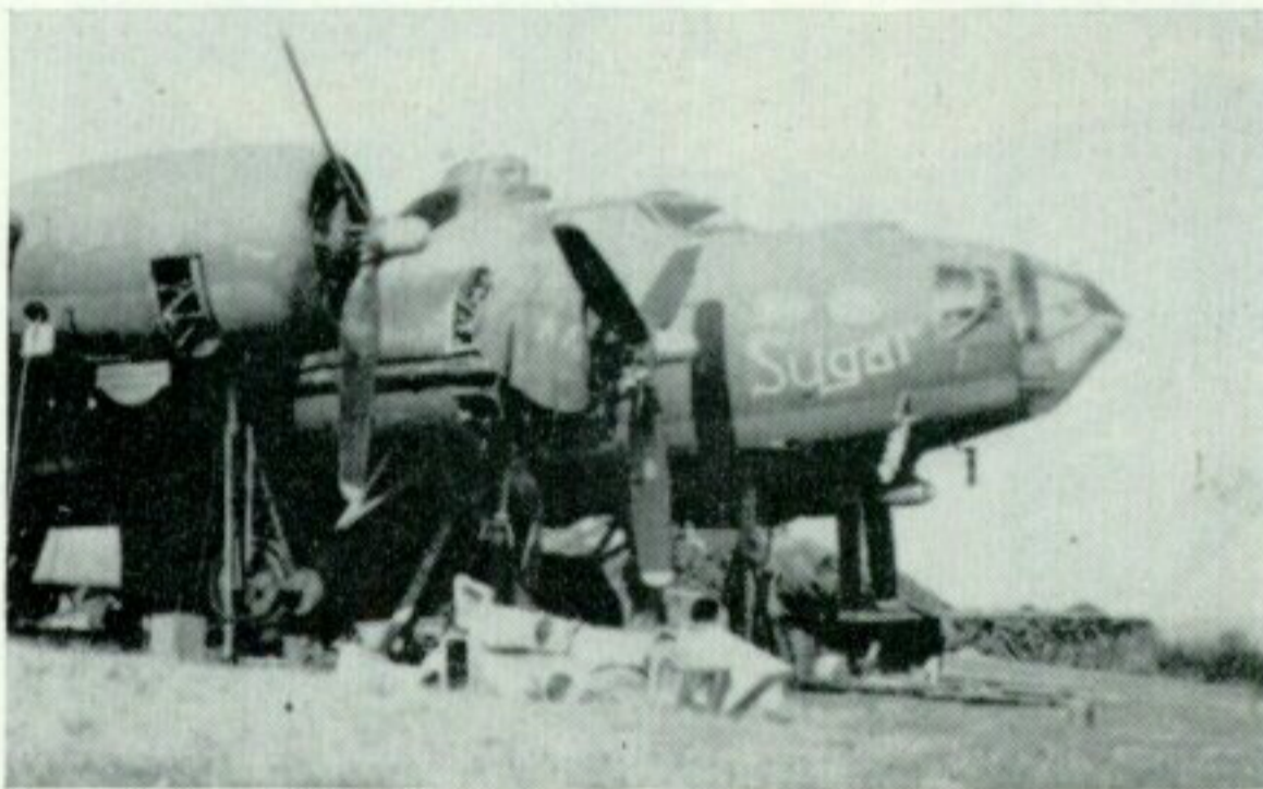
Left: "Sugar", a late model B-17F, displays the cheek positions usually associated with the B-17G. Right: "The Eagle's Wrath", a B-17F-20-BO, serial 41-24524, of the 91st B.G., with twin nose guns. The armour plate covering the bombardier's optical-flat panel is a pointed reminder of the B-17's vulnerability to head-on attack, one of the main reasons for the failure of the Unescorted Daylight Precision Bombing theory. (Photos: W. J. Connell collection)
