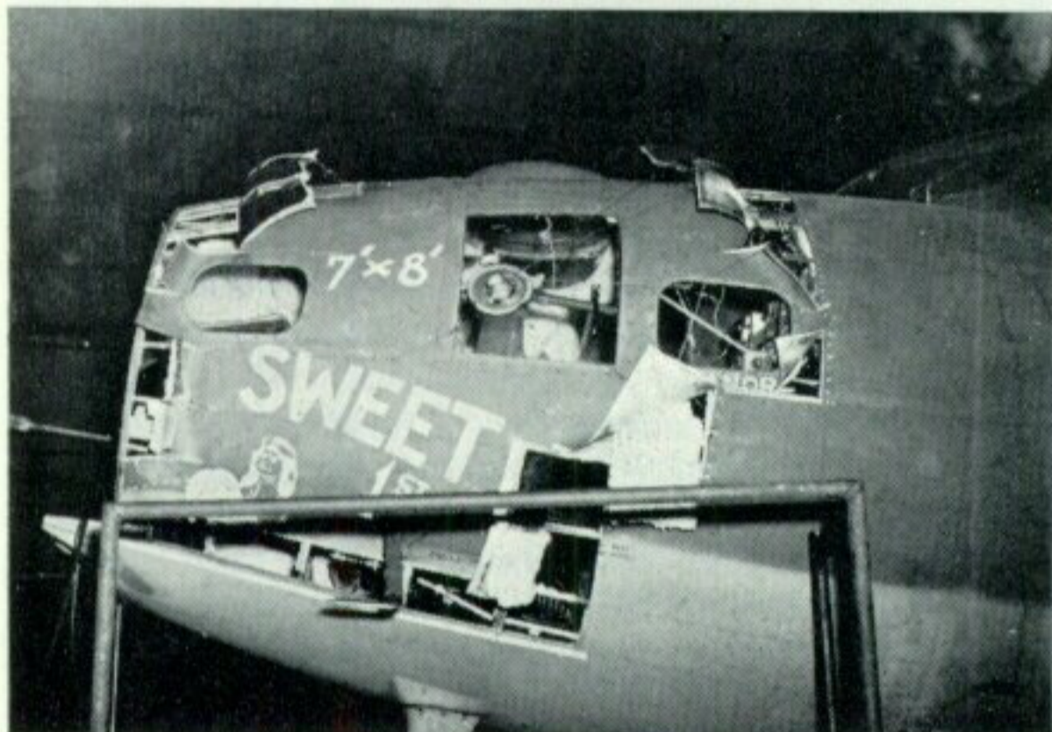
This unusual sequence graphically demonstrates the "repairability" of the Fortress. Top left shows "Eight Ball", a B-17F-25-DL (DO) of the 91st B.G., serial 42-3138, with nose damage from a runaway propeller. The area to be replaced is marked off with masking tape. Top right shows the section removed, with the replacement nose from "Sweet Pea 1st" ready. Bottom left shows the section in place. Bottom right shows job almost complete. (Photos: W. J. Connell collection)
