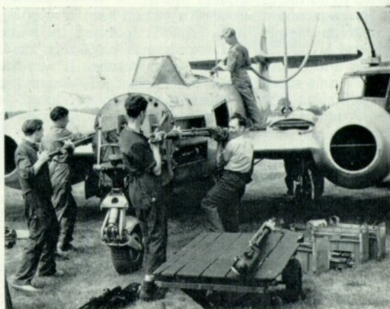
In the field with the Meteor 4. Above: high-speed refuelling of a Norwegian Mk. 4. Below: armourers change the four 20-mm. cannons. (Photos: Ministry of Defence)
