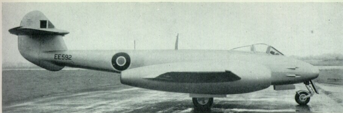
Side, rear and underside flying view of a typical Meteor F. Mk 4 powered by Rolls-Royce Derwent 5 turbo-jets. E.E.592 was a type G.41F Gloster-built aircraft. (Photos: Ministry of Defence)
