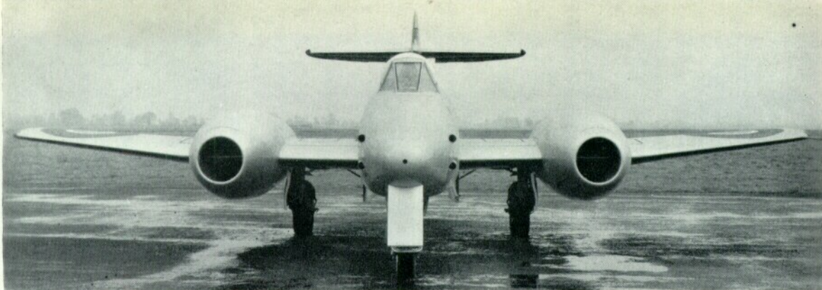
The small frontal area and clean lines of the Mk. 4 show up well in this head-on view. It also illustrates the good grouping and positioning of the four 20-mm. guns and shows the cine camera vision tube in the nose.
