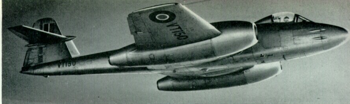
The prototype Meteor F. Mk. 8 was VT150, originally produced as an F. Mk. 4. Modification of the Mk. 4 airframe included a new tail assembly and a 30-inch fuselage extension. (Photo: Hawker Siddeley Aviation Ltd.)
