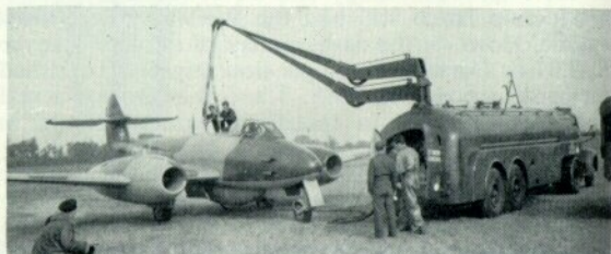
In the field with the Meteor 4. Above: high-speed refuelling of a Norwegian Mk. 4. Below: armourers change the four 20-mm. cannons. (Photos: Ministry of Defence)
