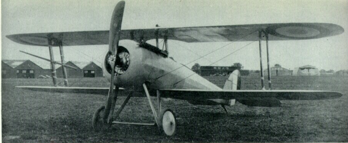
Prototype Nieuport 28 showing absence of dihedral on upper wing.
