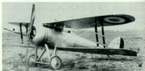
Modified Nieuport 28 prototype, still with single-unit interplane struts but dihedral added to top wing by shortening centre section struts and bringing wing down to fuselage. (Photo: Nieuport)
