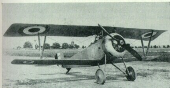
Above, left: The most famous fighting ancestor of the Nieuport 28—the Model 17. (Photo: Signal Corps, U.S. Army). Right: The beginning of the Nieuport 28—a modified Model 24 with 160-h.p. Gnome engine and centre section struts altered to permit mounting of single Vickers machine gun outboard of the struts. New tail shape had appeared on Model 23. (Photo: Nieuport)
