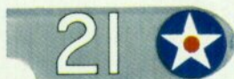
Wing detail for 5800. "21" in four positions, port and starboard upper, port and starboard undersurfaces.
