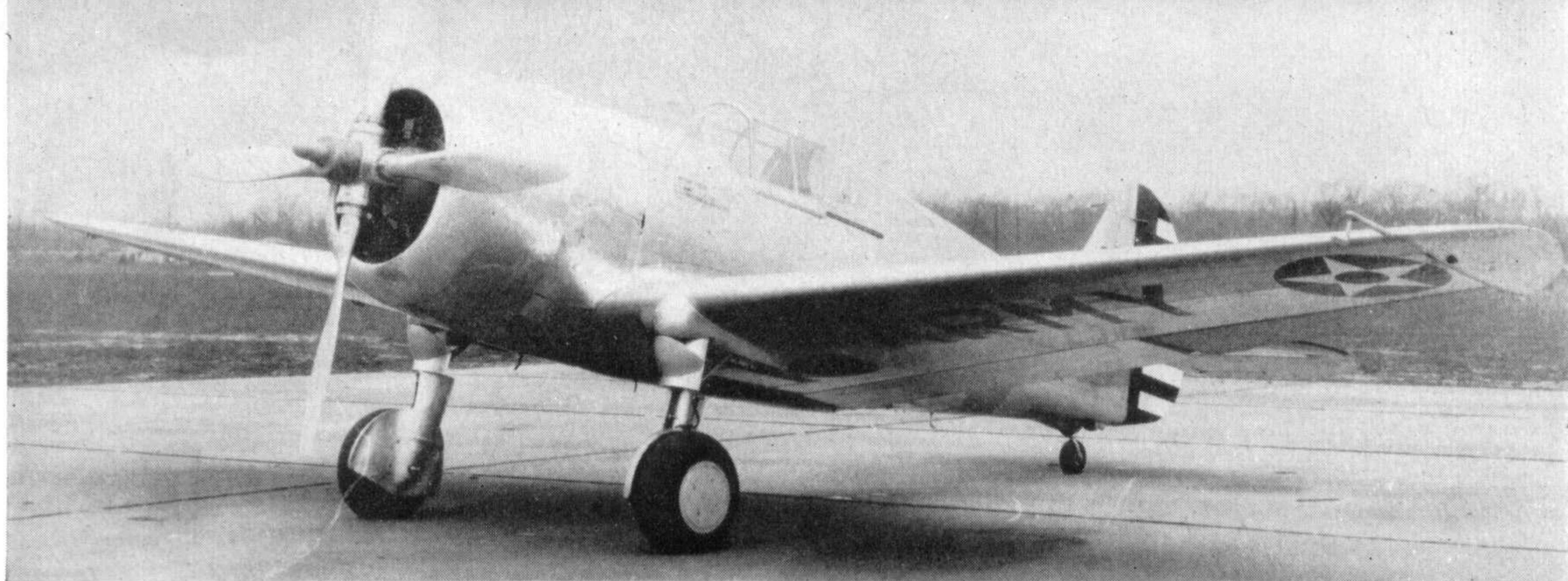
Curtiss Model 75E, one of three tested by the Air Corps as Y1P-36. The machine illustrated, serial 37-68, has been fitted with an experimental four-blade Curtiss electric propeller. (Photo: U.S.A.F.)
