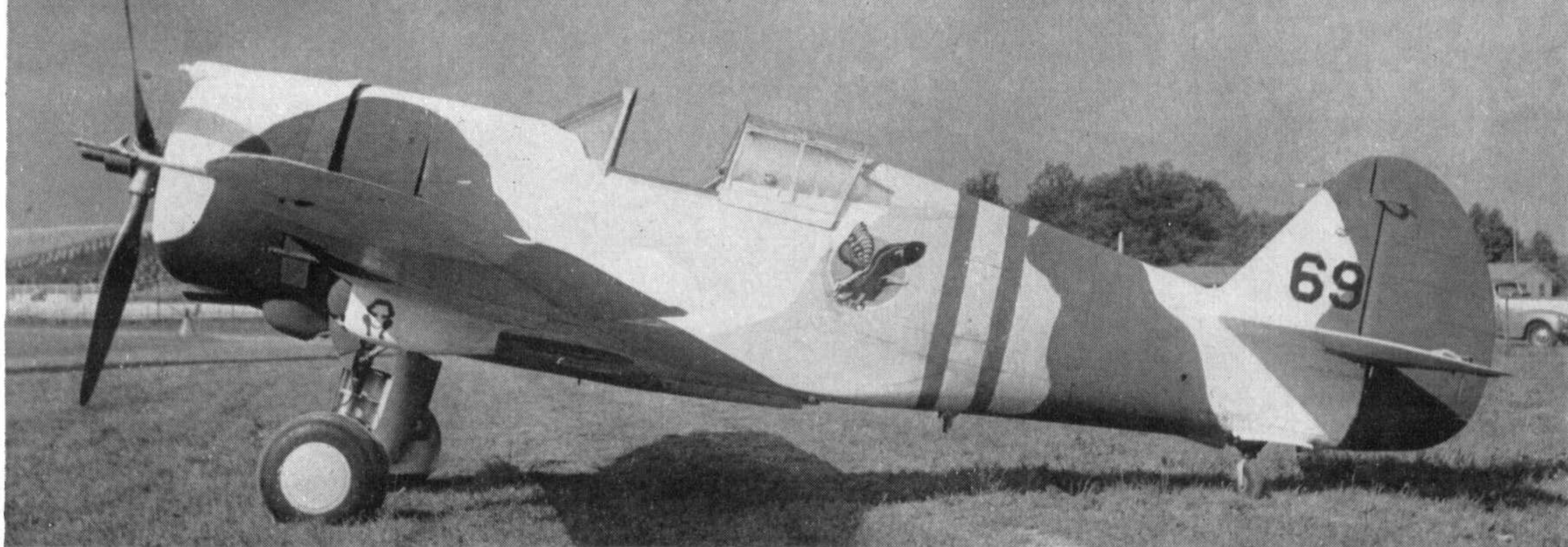
Above: A P-36C, probably of the 27th Pursuit Squadron, with the experimental camouflage of the 1939 War Games. The external underwing ammunition box for the .30 calibre wing guns is clearly visible. (Photo: courtesy Gordon S. Williams.) Below: Another P-36C with a different War Games camouflage pattern; these schemes were applied with washable paint and could easily be removed. (Photo: courtesy William T. Larkins)
