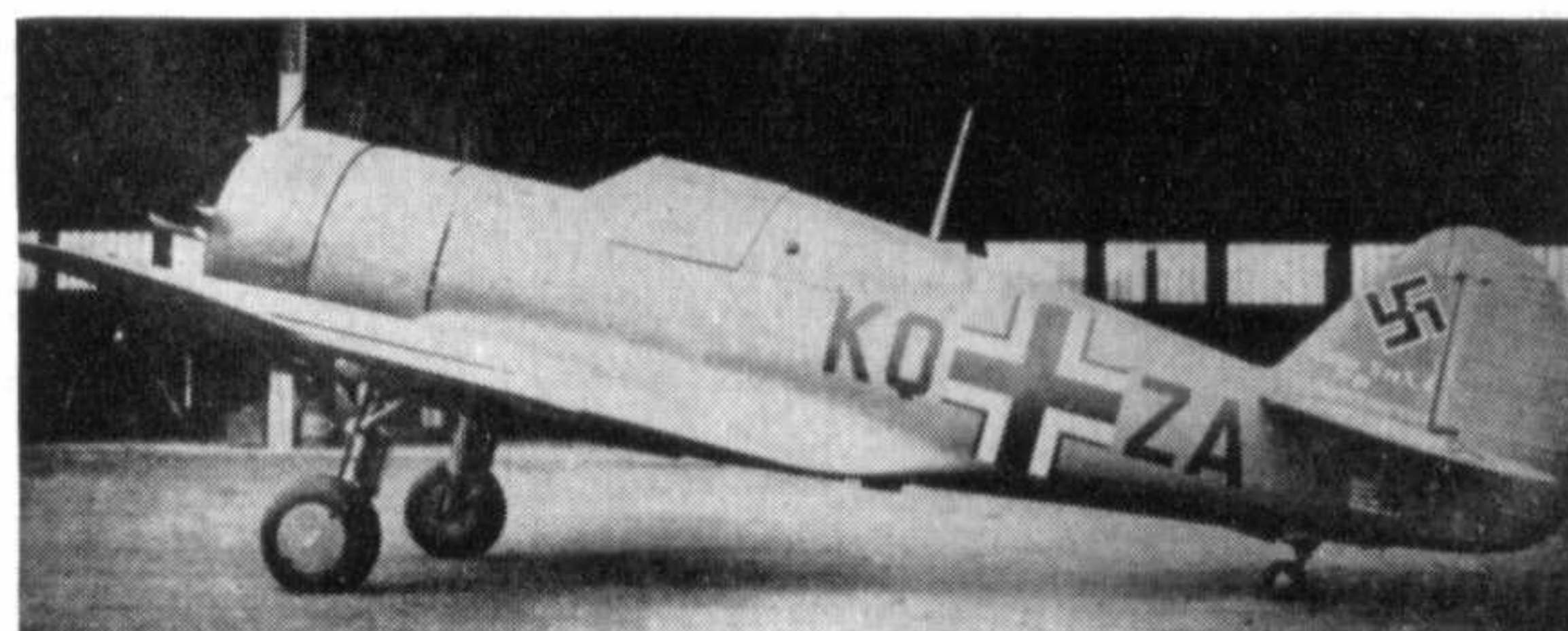
Left: Hawk H75A-2 of l'Armée de l'Air; compare wide rudder stripes with those on the aircraft illustrated at the foot of page 3, where the stripes were kept aft of the rudder hinge line. (Photo: courtesy Charles W. Cain.) Right: A Cyclone-powered H75A-4 taken over by the Luftwaffe for training use after the fall of France in 1940. (Photo: courtesy H. J. Nowarra)
