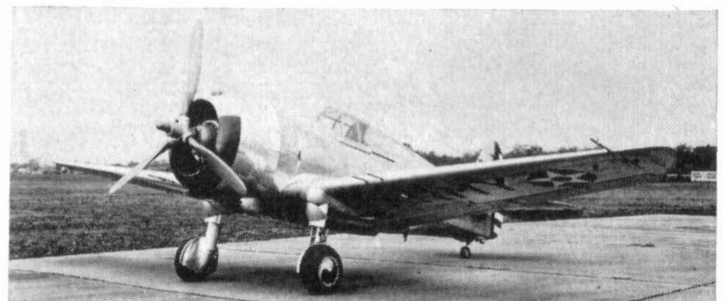
Left: P-36B, a temporary designation assigned to P-36A 38-20 while being used as a test-bed for a 1,100-h.p. R-1830-25 engine. Right: The single XP-36D was created by installing .30 calibre machine guns in each wing panel of P-36A 38-174. Note segmented colouring on cowling of an aeroplane used by a Group Headquarters Squadron. (Photos: U.S.A.F.)
