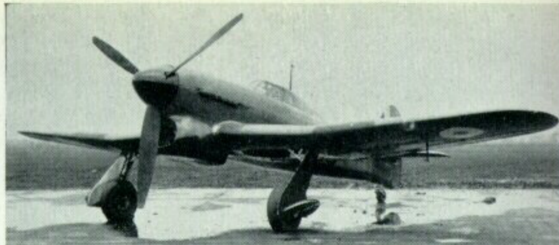
Two early photos of the second Typhoon prototype, P5216. That on the left, taken at Boscombe Down, shows the 12-gun wing to advantage as well as the hinged door flaps attached to the leg fairings. Note also the tailwheel doors. Right: A later photo taken at Langley after the tailwheel doors had been removed.
