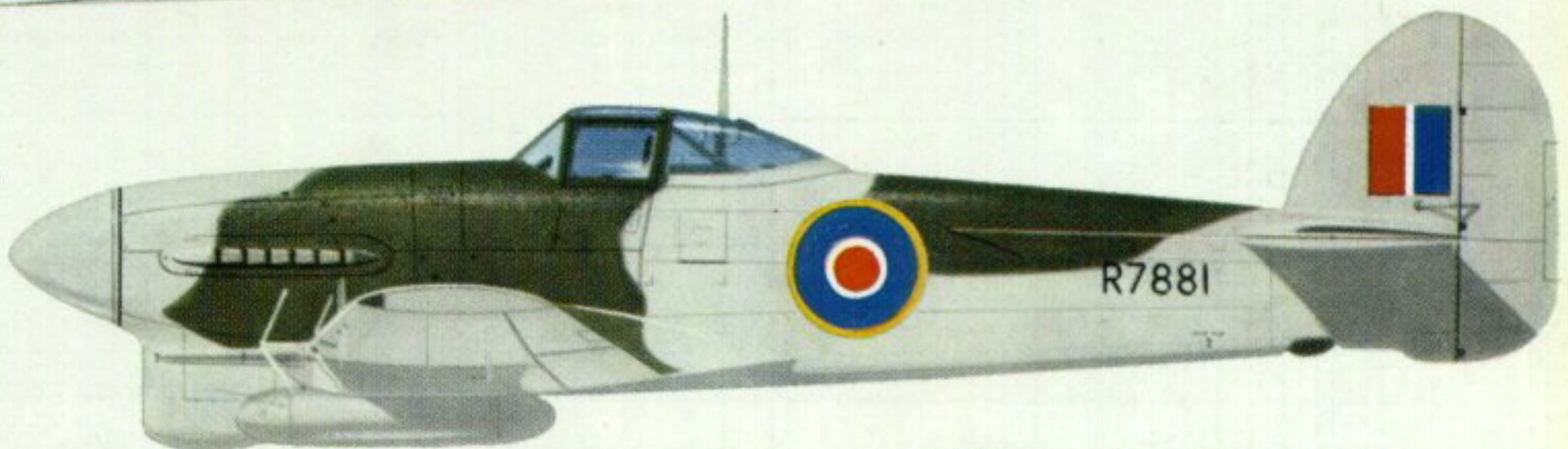
Typhoon T.T.I (believed SW500); target tug flown by 2nd Tactical Air Force, late 1945, and by No. 56 O.T.U., 1946 (markings of latter shown).
