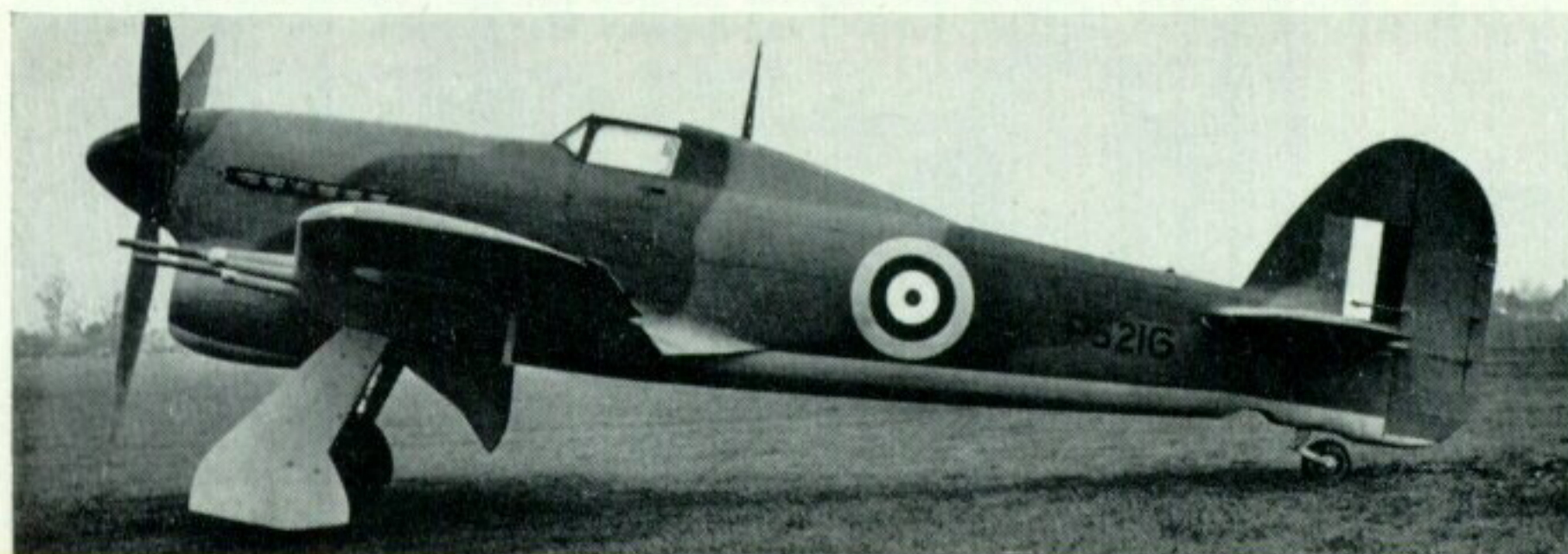
P5216 after it had been brought up to the initial production standard. Centrally-hinged mainwheel doors have been fitted, as has the four-cannon armament. Standard "dark earth and spinach" camouflage has been applied, but the absence of the "circled-P" is curious. (Photo: Hawker Siddeley Aviation Ltd., Neg. No. TYG5)
