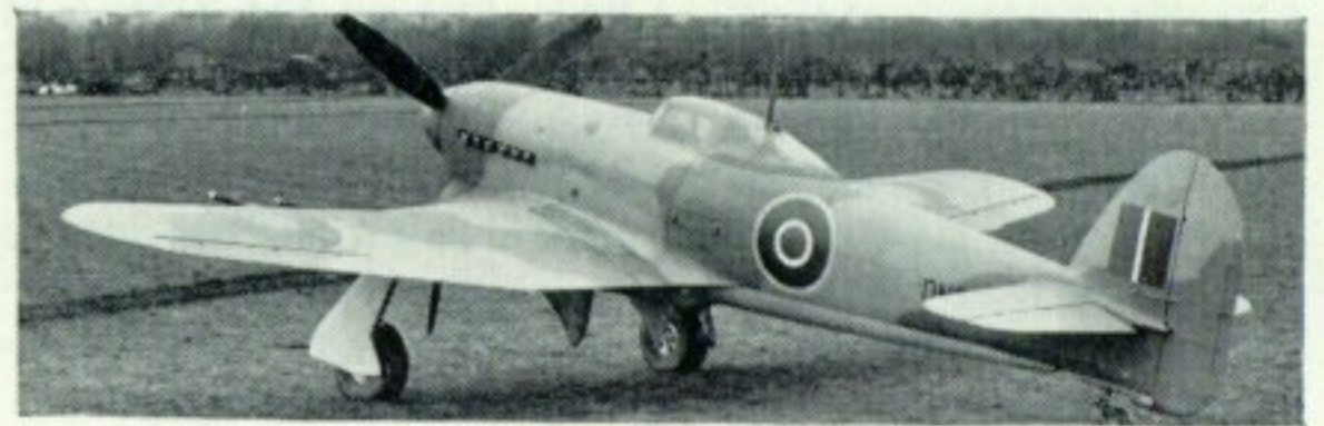
Two views of one of the tropical Typhoons. Just visible is the ventral air exit fairing between the central wheel doors. Colour scheme was sand and dark green upper surfaces and pale blue undersurfaces. Two other Typhoons, R8925 and R8889, were also equipped for tropical trials and all were shipped to Khartoum early in 1943.
