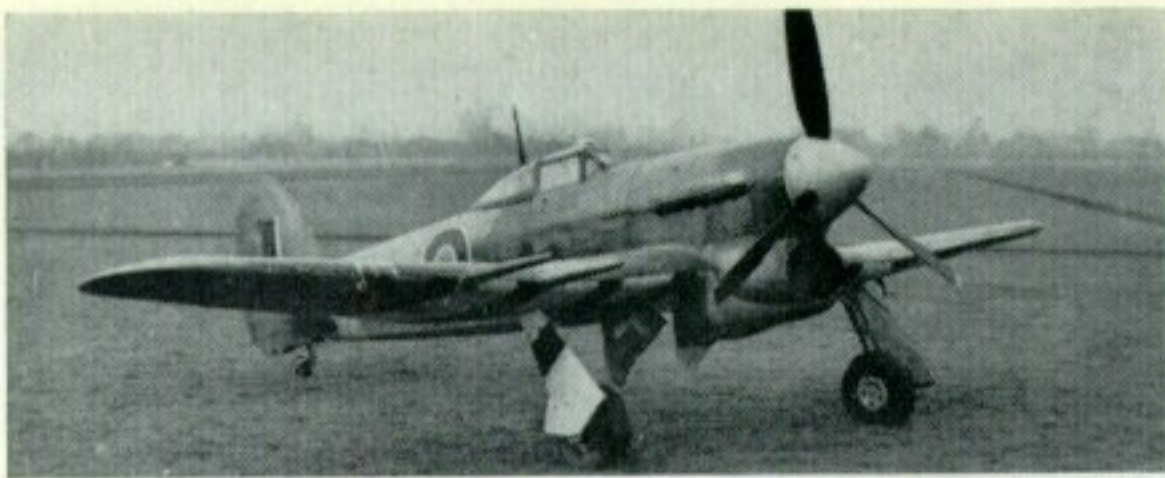
Cleaning up the Typhoon. A programme was initiated in 1942 to increase the performance by attention to detail; pictures of R8809 show the change in hood shape, elimination of external rear view mirror, adoption of whip aerial, fairing of cannon barrels and addition of exhaust manifold plinth. (Photos: Hawker Siddeley Aviation Ltd., Neg. Nos. TYG4 and TYG37)
