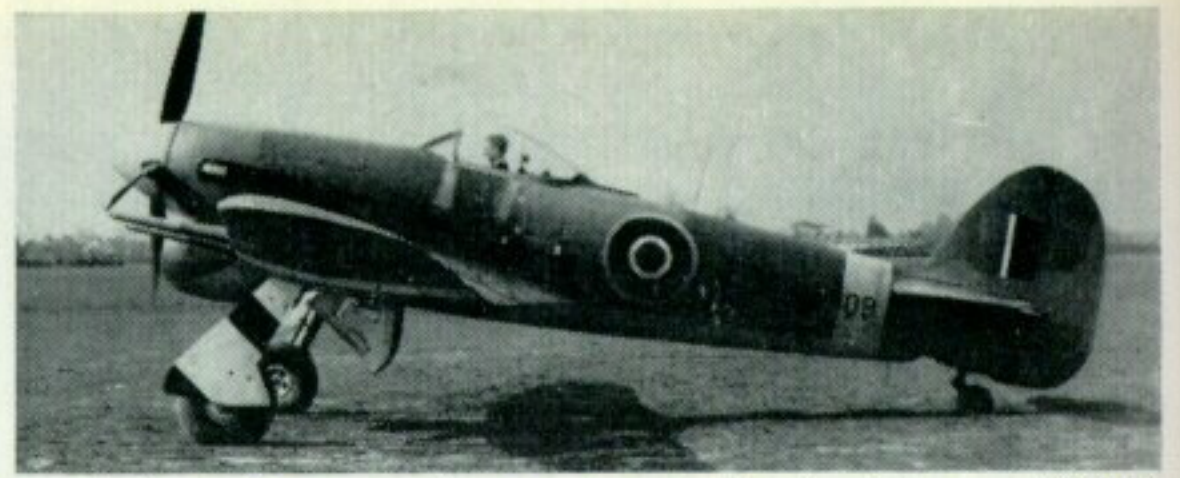
Cleaning up the Typhoon. A programme was initiated in 1942 to increase the performance by attention to detail; pictures of R8809 show the change in hood shape, elimination of external rear view mirror, adoption of whip aerial, fairing of cannon barrels and addition of exhaust manifold plinth. (Photos: Hawker Siddeley Aviation Ltd., Neg. Nos. TYG4 and TYG37)
