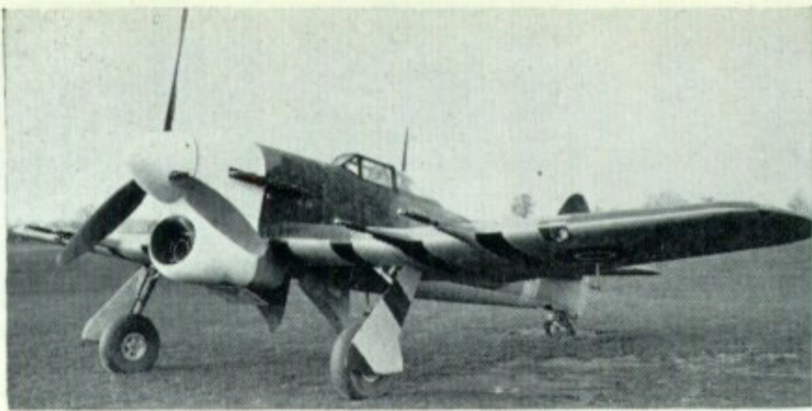
Typhoon IB, R8224, was used for investigation into recognition schemes to eliminate confusion with the Focke-Wulf Fw 190A. The white nose was tried in an effort to so modify the Typhoon's appearance as to leave no superficial resemblance. After various alternative schemes had been discarded, reliance was placed on the now-familiar black and white stripes under the wings.
