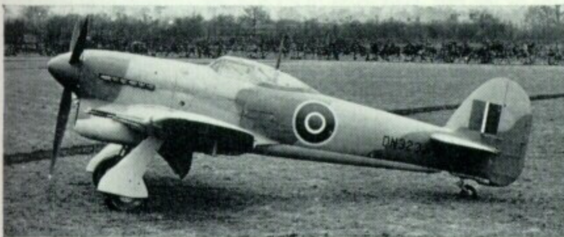
Two views of one of the tropical Typhoons. Just visible is the ventral air exit fairing between the central wheel doors. Colour scheme was sand and dark green upper surfaces and pale blue undersurfaces. Two other Typhoons, R8925 and R8889, were also equipped for tropical trials and all were shipped to Khartoum early in 1943.
