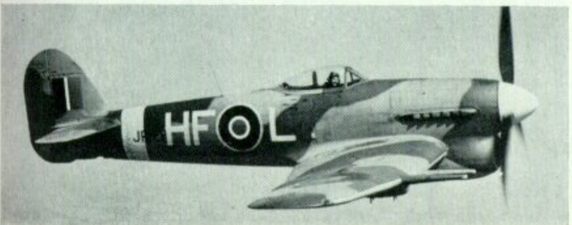
For many months No. 183 (Fighter) Squadron flew Typhoons on fighter-bomber strikes. These two pictures are interesting in that both aircraft are carrying the same code letters; that above, R8884, was one of the first Typhoons modified to carry underwing bombs (note old canopy and unfaired cannon). JR128 displays faired exhaust stacks, faired cannon, sliding canopy, whip aerial and 3-blade propeller.
