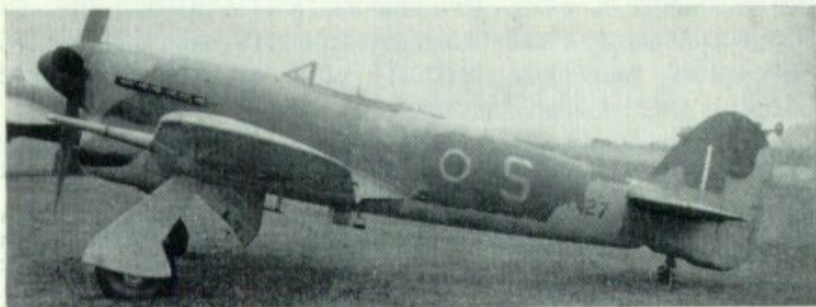
Two views of a Typhoon F.R.IB, EK427. Armed with the outboard cannon only, these aircraft were equipped to carry a forward-facing camera in the starboard inboard gun bay, an oblique camera in the port wing and one or two vertical cameras in the fuselage. About sixty such aircraft were thus modified. (Photos: Ministry of Defence, and Imperial War Museum)
