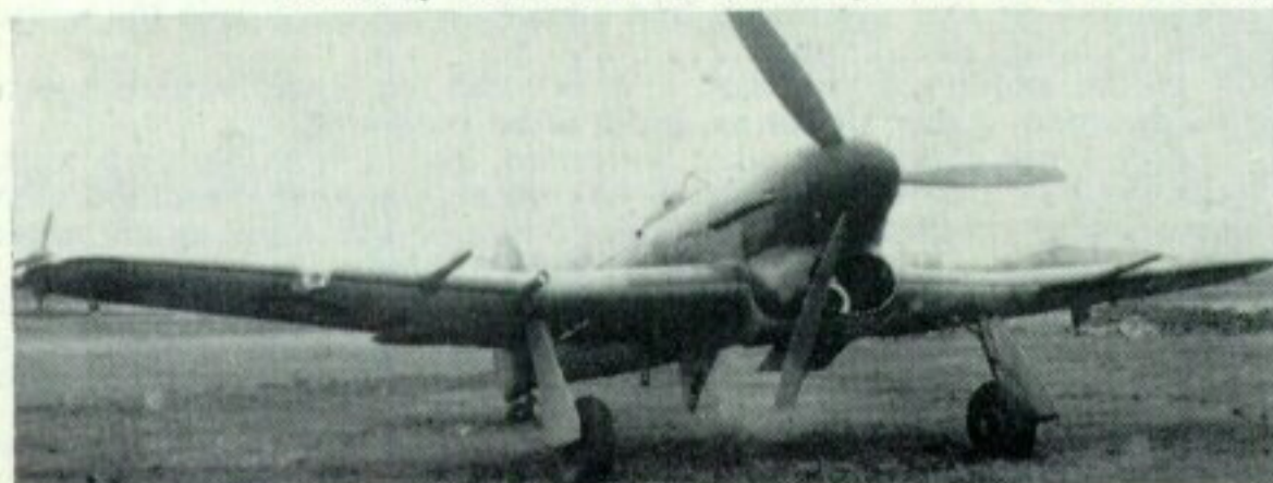
Two views of a Typhoon F.R.IB, EK427. Armed with the outboard cannon only, these aircraft were equipped to carry a forward-facing camera in the starboard inboard gun bay, an oblique camera in the port wing and one or two vertical cameras in the fuselage. About sixty such aircraft were thus modified. (Photos: Ministry of Defence, and Imperial War Museum)
