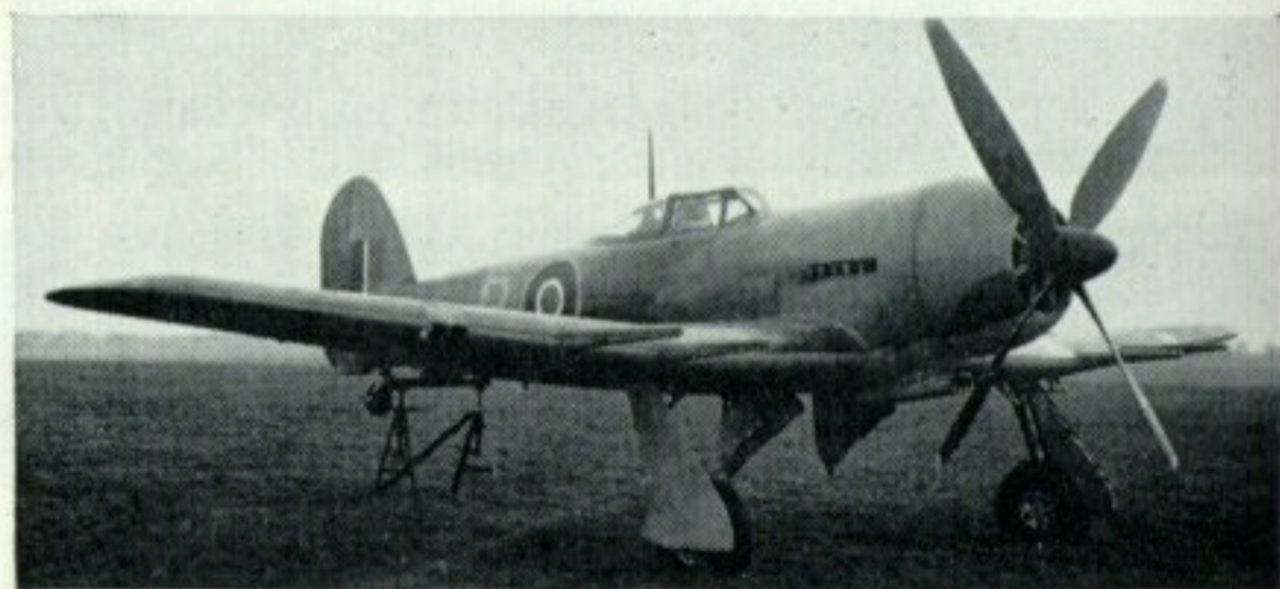
One of the interesting installations carried out on the Typhoon was that of the annular radiator with Sabre II and IV engines in R8694. By and large this was a successful experiment but disruption to production lines forestalled any interest by the Air Ministry. Top speed was quoted by Napiers at 452 m.p.h.
