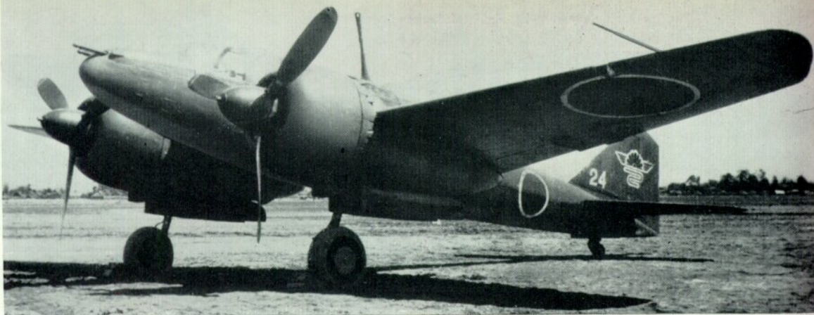
Army Type 100 Air Defence Fighter of the 16th Dokuritsu Hikotai. Note oblique-mounted 37-mm. Ho-203 cannon. (Photo: courtesy Aireview)
