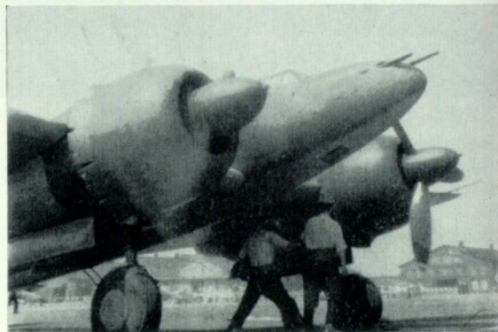
A Ki-46-III Kai prepares for take-off; note nose battery. (Photo: R. Ward collection)
