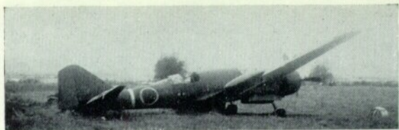
Although the strengthening of the undercarriage was one of the requirements of the Ki-46-III development, the Model 3 still suffered chronic weakness of the landing gear struts.
