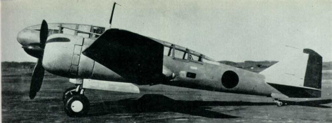
Port side view of the Ki-46-IV reveals turbo-supercharger installation at the rear of the engine nacelle. (Photo: courtesy Aireview)
