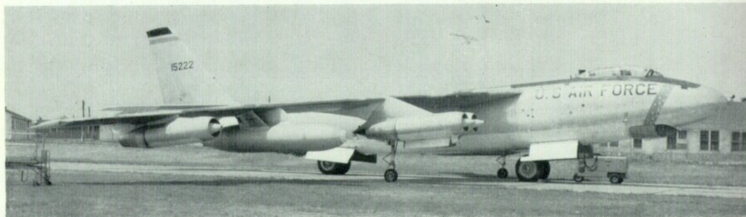
Boeing-built B-47E with auxiliary fuel tanks and the star-spangled blue band of a Strategic Air Command aircraft painted on the nose. (Photo: Peter M. Bowers)
