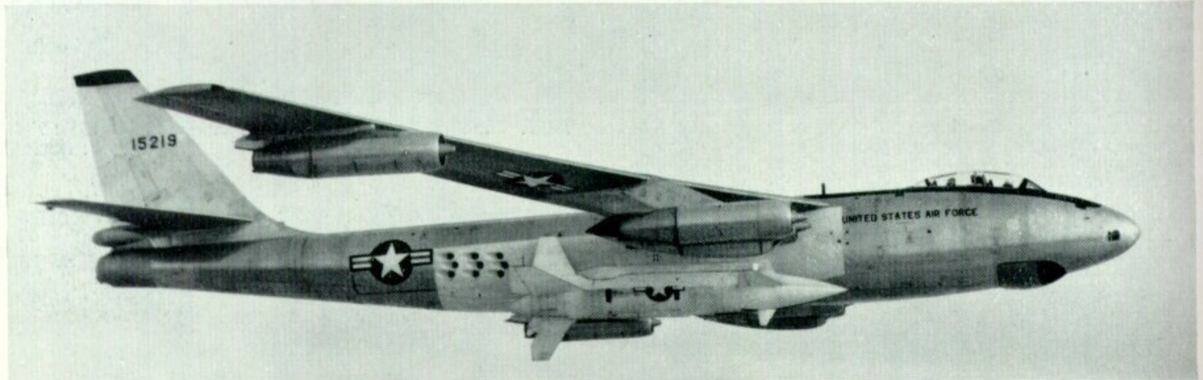
YDB-47E carrying Bell GAM-63 "Rascal" missile. The white-painted area on the B-47 fuselage is to provide a good background for photos of the missile release during tests. (Photo: Boeing)
