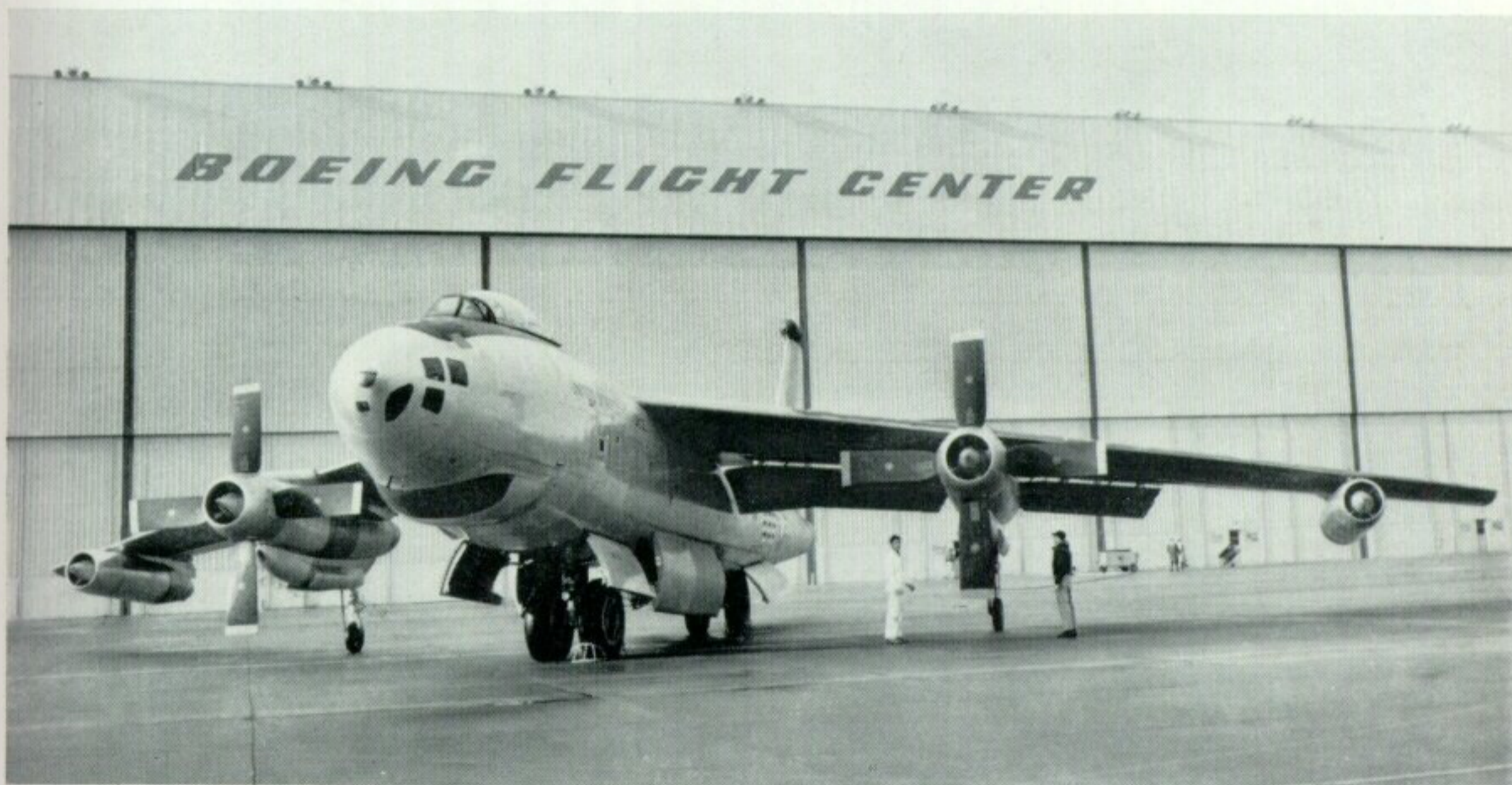
The four-bladed Curtiss turbo-electric propellers, each 15 feet in diameter and having "paddle-type" blades 24 inches wide, were used with the T-49s. Changes necessary to adapt the 600-mile-an-hour bombers for the test duties included removal of the original twin-jet inboard engine pods, modification of wing flaps to allow installation of the T-49s, and changes in instrumentation and controls for four engines rather than the normal six engines. (Photo: Boeing)
