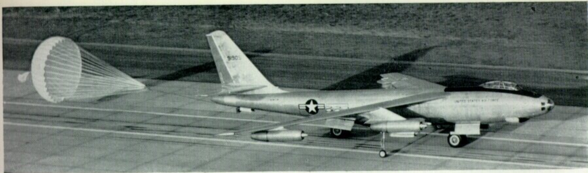
The No. 6 B-47A demonstrates the use of the thirty-two-foot diameter deceleration parachute.
