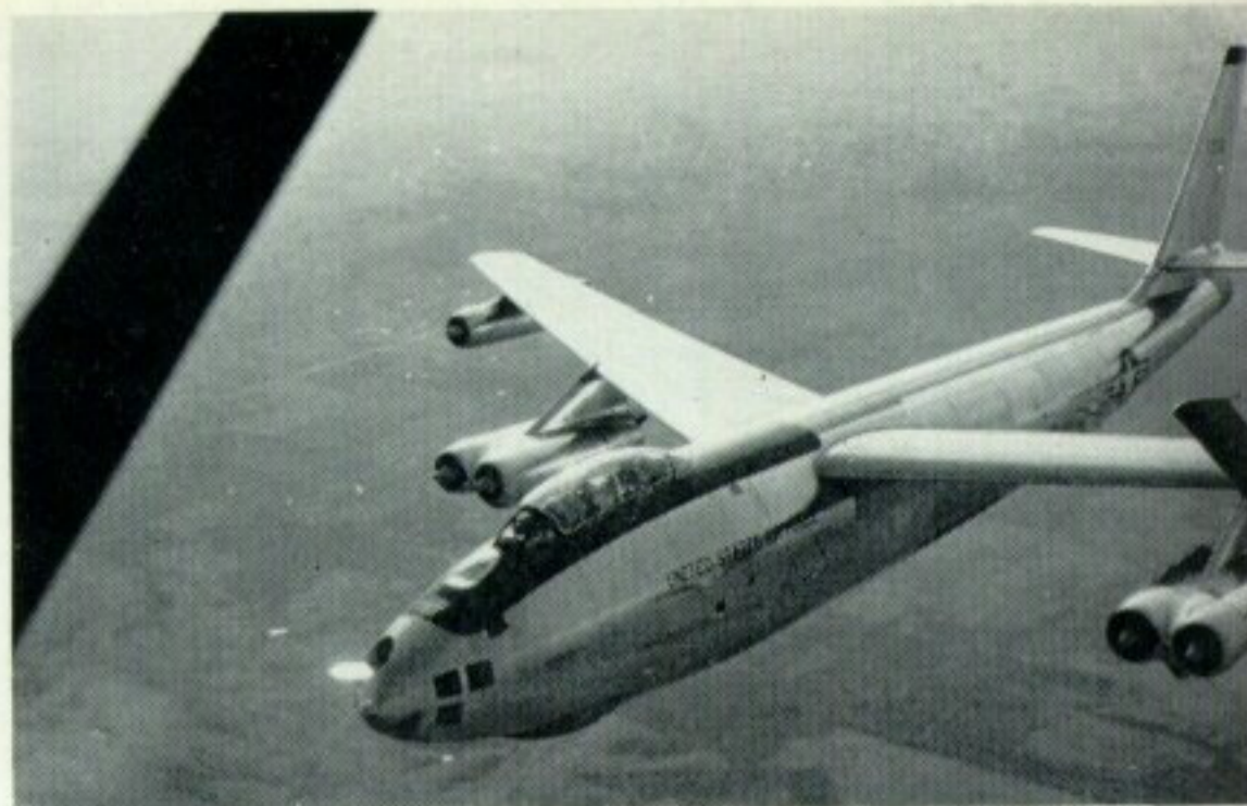
Early B-47E with in-flight refuelling receptacle in nose opened. (Photo: Boeing)
