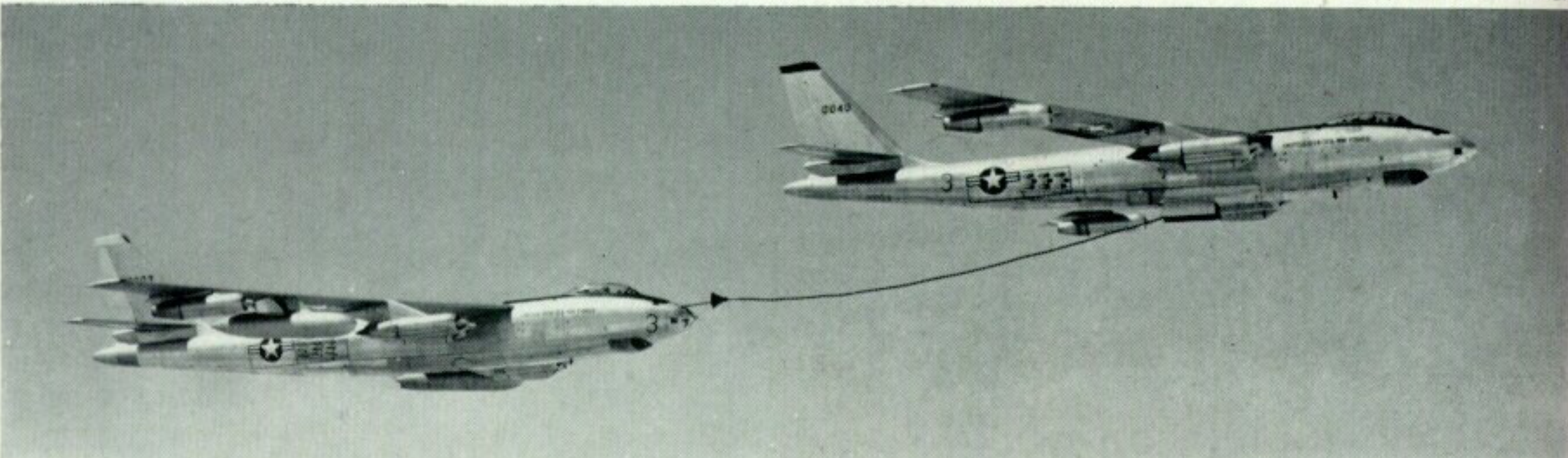
The YB-47F being refuelled from the KB-47G hose tanker. Both of these experimental machines were converted from B-47B airframes. (Photo: Boeing)
