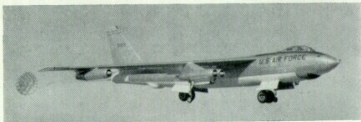
A Lockheed-built B-47E with the sixteen-foot diameter "Ribbon" approach parachute during landing. (Photo: Peter M. Bowers)
