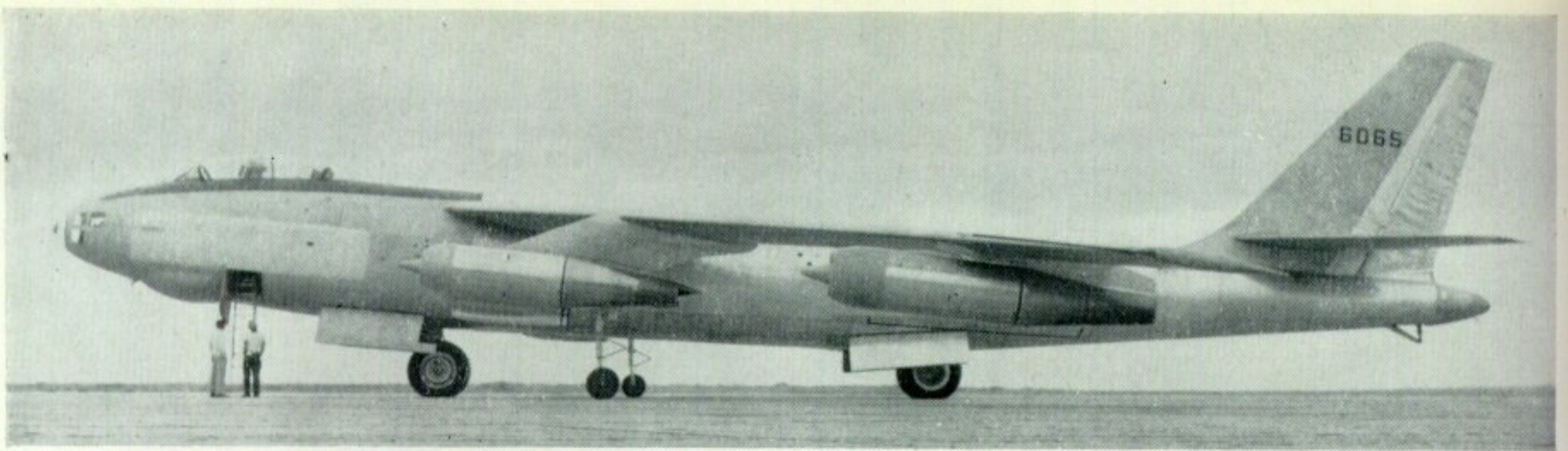
The No. 1 XB-47 shows the ground angle established by the tandem landing gear.
