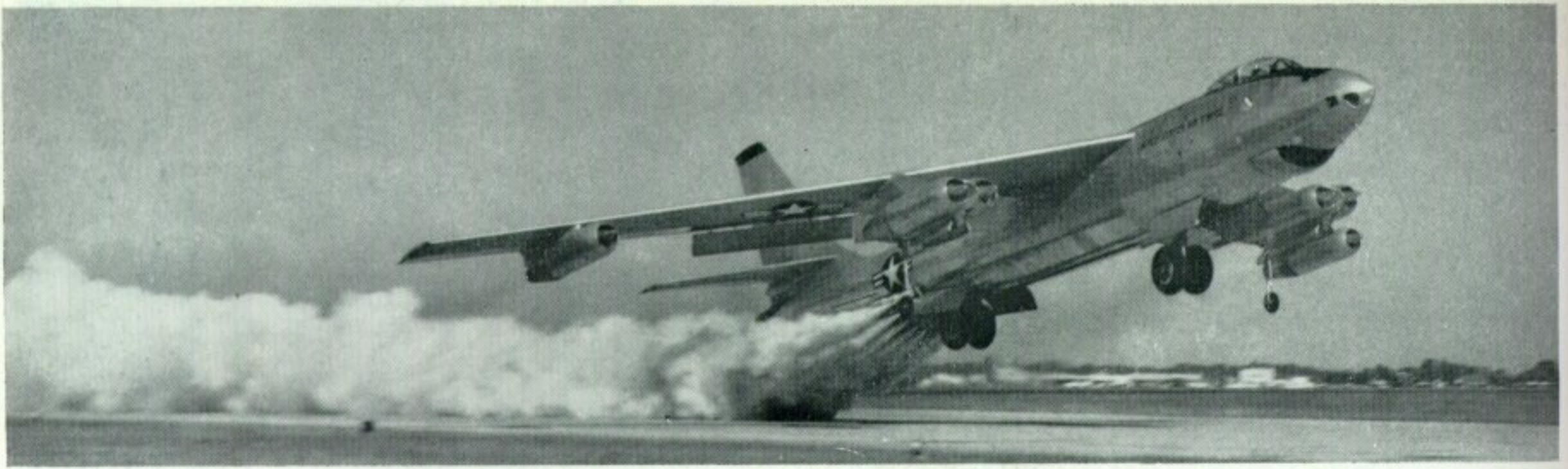
B-47E taking off with the assistance of thirty-three externally-mounted JATO bottles.
