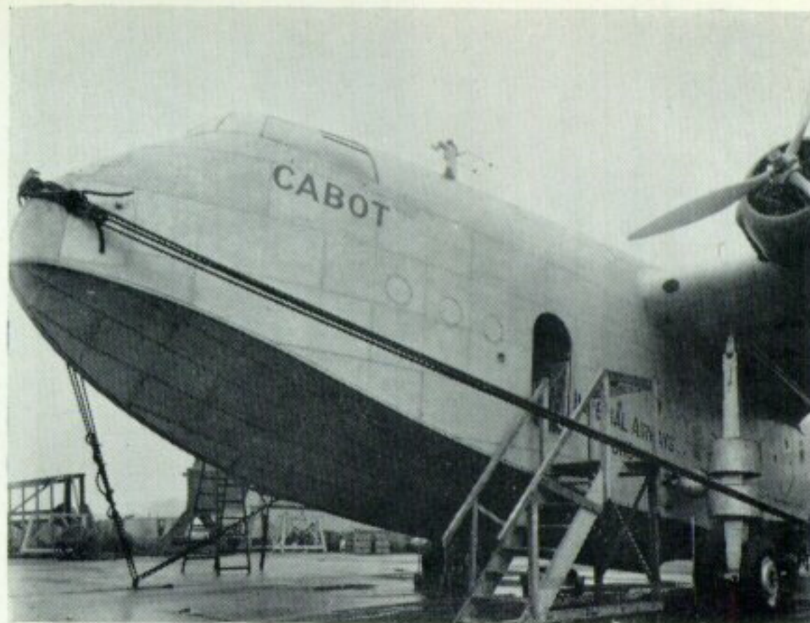
Cabot, first "C" Class boat to take-off at an a.u.w. of 46,000 lb. (Photo: Short Bros. and Harland)
