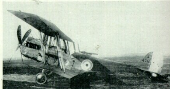
Left: On A3186 the area of the upper fin was slightly increased, but the underfin remained its original size. Right: Subject of the official performance test report quoted in the table on page 12, A4716 had the standard design of upper fins and underfins fitted to all operational R.E.8s until the end of the war. (Photos: Imperial War Museum Q56852 and Q63817)
