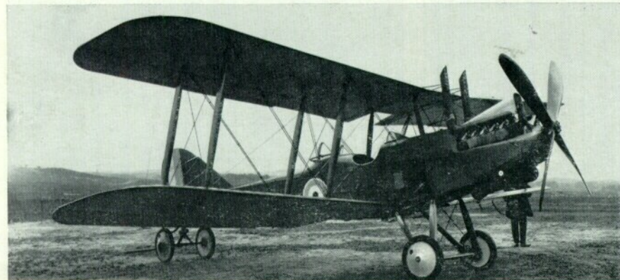
The R.E.9 A4600 at Farnborough, 24th September 1917, with enlarged upper fin. (Photo: Crown copyright)
