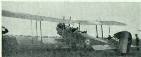
A3406 fitted with the enlarged fin and balanced rudder designed for the R.E.8 but almost indistinguishable from the corresponding surfaces designed for the R.E.9 and R.T.1.
