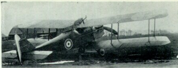
The first Siddeley-built R.T.1, B6625, with 200-h.p. Hispano-Suiza engine. The pilot's gun was a Lewis above the centre section. The external gravity tank was somewhat similar to that of the early production S.E.5. (Photo: Crown copyright)
