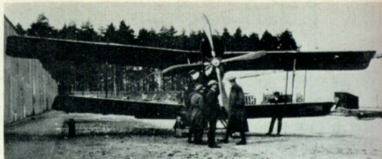
The R.E.8 B738 with supercharged R.A.F. 4d engine, R.A.F. variable-pitch airscrew and balanced rudder similar to that of A3406. The tall figure immediately to the right of the aircraft is Lt. Harold Elliott who was then in charge of the Engines Flight at Farnborough and flew as flight observer in this aircraft and in the Maori-powered R.E.9 A3561.
