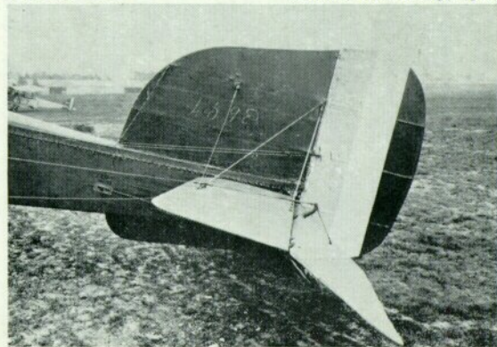
The 12 sq. ft. fin fitted to A4598. This photograph is dated 10th May 1917 (Photo: Crown copyright)
