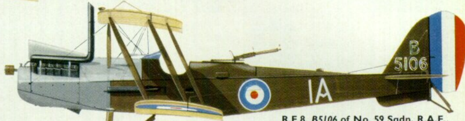
R.E.8, B5106 of No. 59 Sqdn. R.A.F., Vert Galand, May 1918. Fitted with deep sump cowling and navigation lights.
