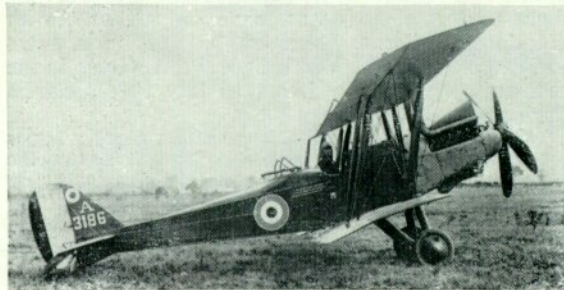
Left: On A3186 the area of the upper fin was slightly increased, but the underfin remained its original size. Right: Subject of the official performance test report quoted in the table on page 12, A4716 had the standard design of upper fins and underfins fitted to all operational R.E.8s until the end of the war. (Photos: Imperial War Museum Q56852 and Q63817)
