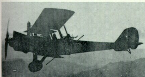
The Davis-gun R.E.8 in flight over inhospitable country. Although seen here in silhouette only, this photograph gives a clear impression of the gun's enormous length.
