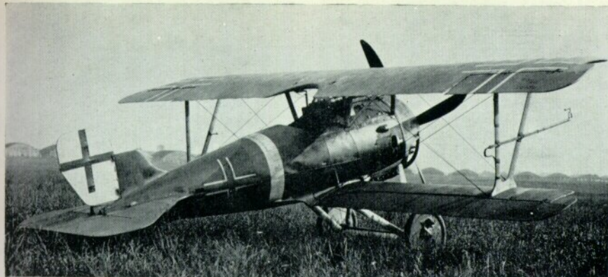
Note this S.S.W. D III in Allied hands does not have headrest. Attachment to "V" struts is probably a yaw meter. (Photo: Imperial War Museum)
