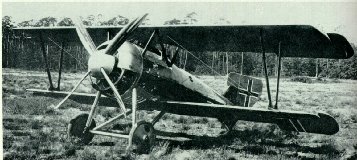
An aircraft of the third production batch; D III D 3008/18. Note at this stage spinner was not punched with cooling louvres.
