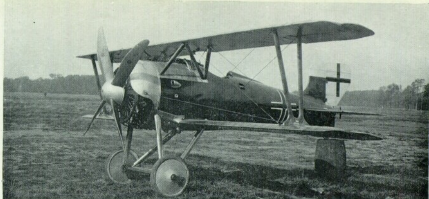
S.S.W. D IV "ex works". Note bright metal panels and lozenge-fabric-covered wings and wheel discs. (Photo: Egon Krueger)
