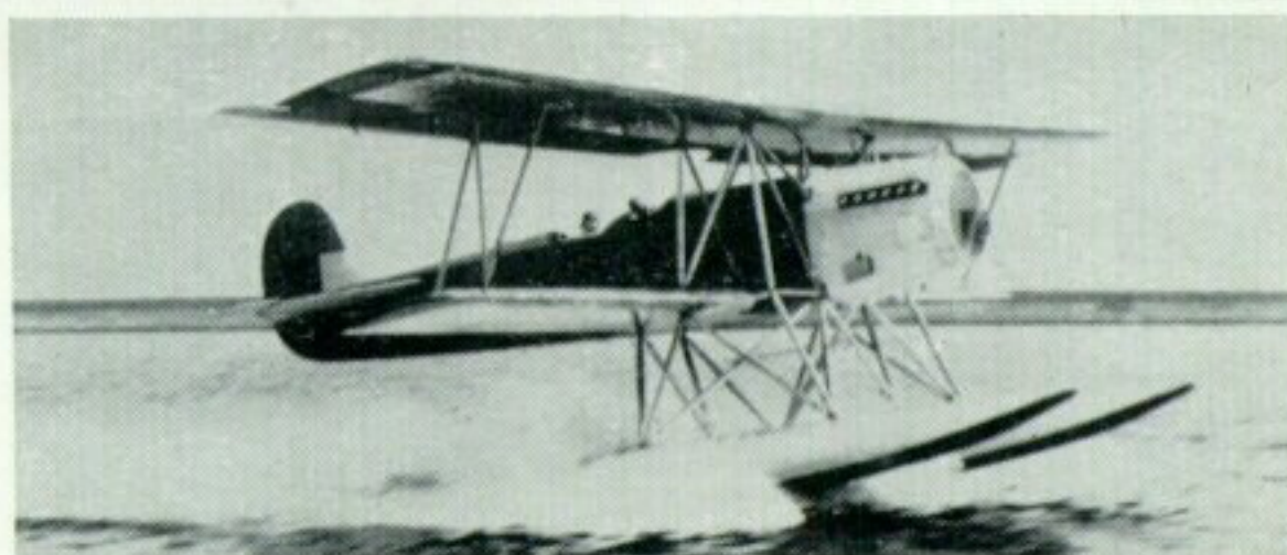
Six C.V-Ws, basically C.V-Cs with float undercarriages, were delivered to the Dutch Naval Air Service in 1925. The variant was not a success, and there were many landing accidents. (Photo: Royal Netherlands Navy)
