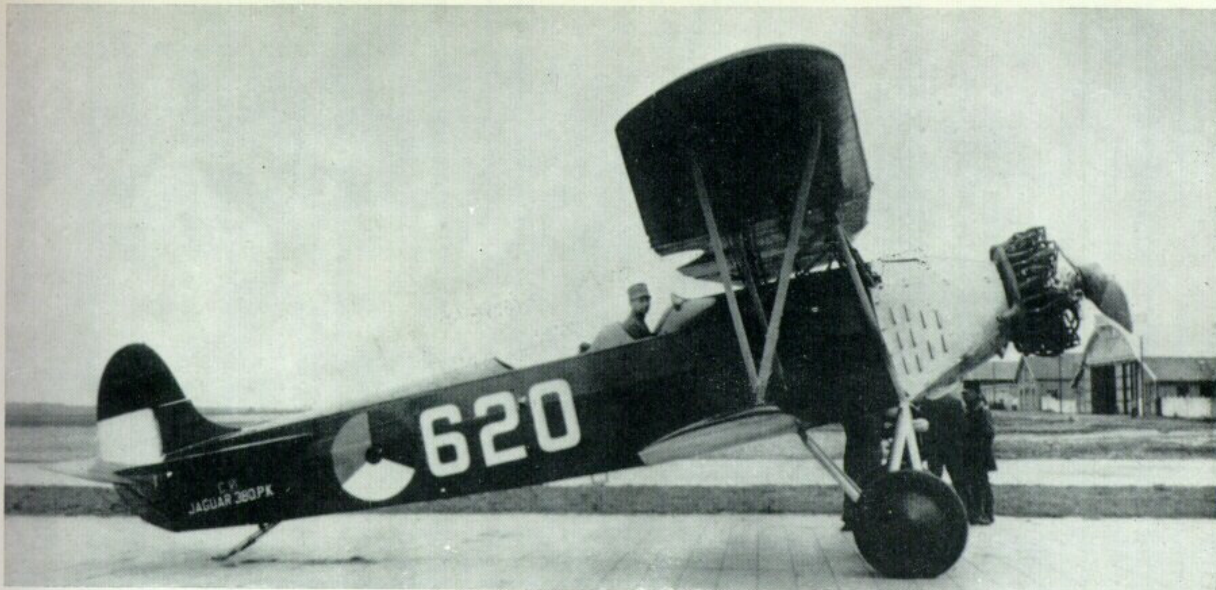
"Fokker C.VI" development of the basic C.V-D, powered by a 380-h.p. Jaguar engine. (Photo: Royal Netherlands Air Force)
