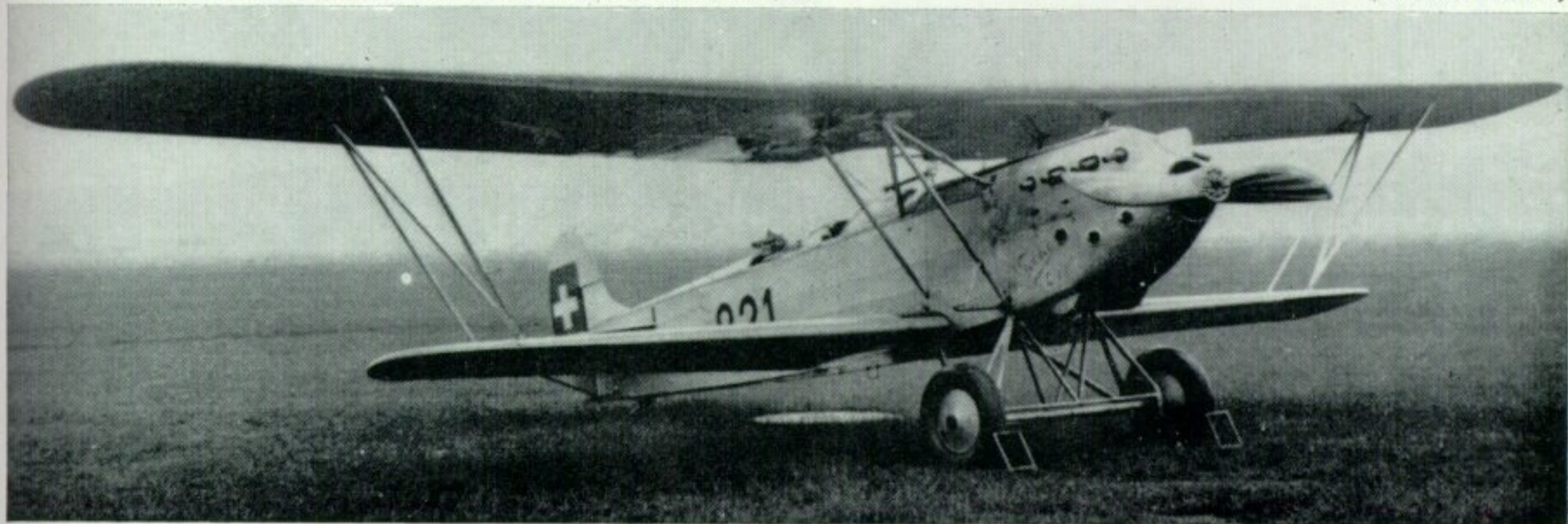
Swiss-built C.V-E No. 321, with a 475-h.p. Lorraine-Dietrich engine. (Photo: Fokker)
