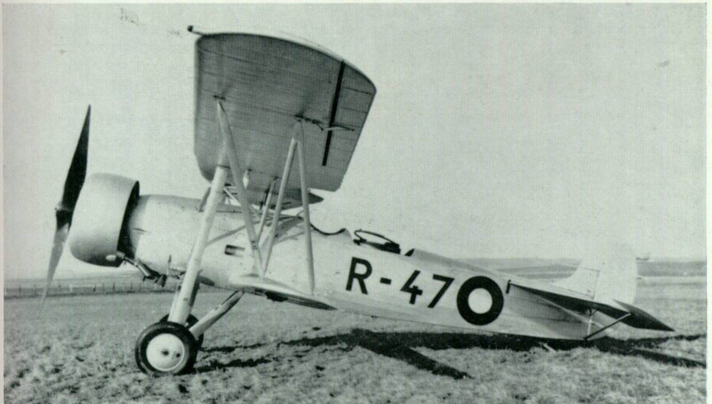
Danish-built machine with modified cowl-ring and gun mounting in rear cockpit.
