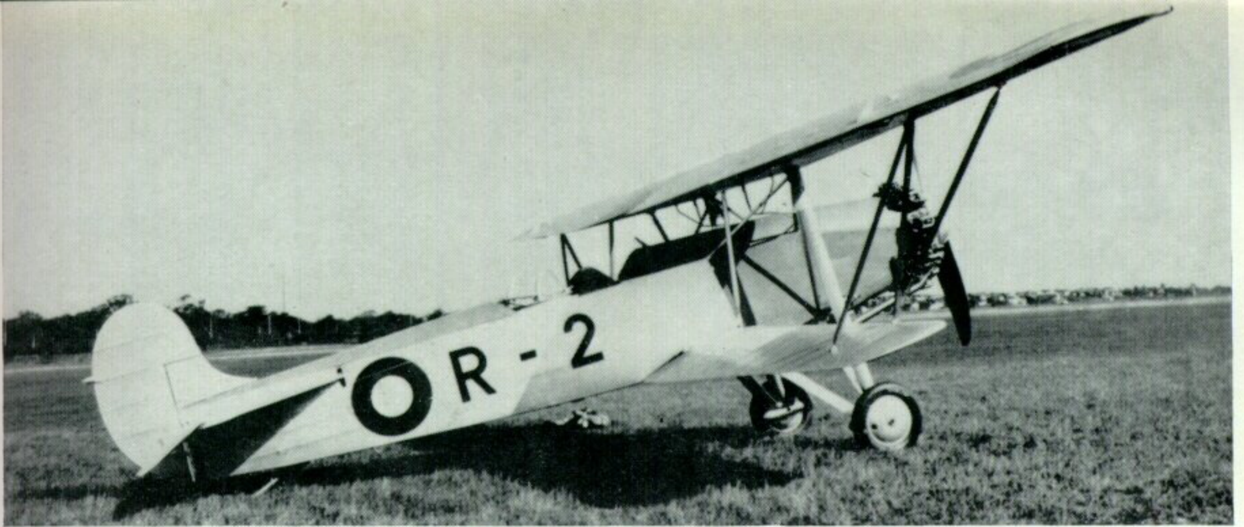
Danish C.V-E with Jupiter VI engine. The code R-2 appears to be a re-issue; the original R-2 was powered by a Lorraine Dietrich engine, and was a C.V-B of the first order batch.
