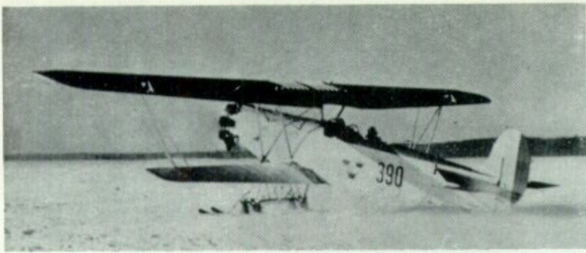
Swedish C.V-E (S-6B) with ski undercarriage. (Photo: Fokker)
