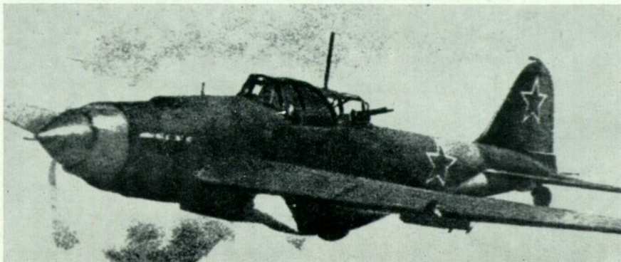
Underwing racks are clearly visible in this view of an Il-2m3 in flight. (Photo: courtesy Skrzydlata Polska)
