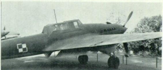
Views of the Il-2m3 preserved at the Polish Armed Forces Museum at Warsaw: note the extremely heavily armoured cockpit. The great crew and engine protection afforded by the Ilyushin's construction led to its being christened "The Flying Tank" by wartime crews, and one of the outstanding features of its operational career was its ability to absorb considerable combat damage.
