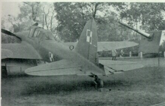
Views of the Il-2m3 preserved at the Polish Armed Forces Museum at Warsaw: note the extremely heavily armoured cockpit. The great crew and engine protection afforded by the Ilyushin's construction led to its being christened "The Flying Tank" by wartime crews, and one of the outstanding features of its operational career was its ability to absorb considerable combat damage.
