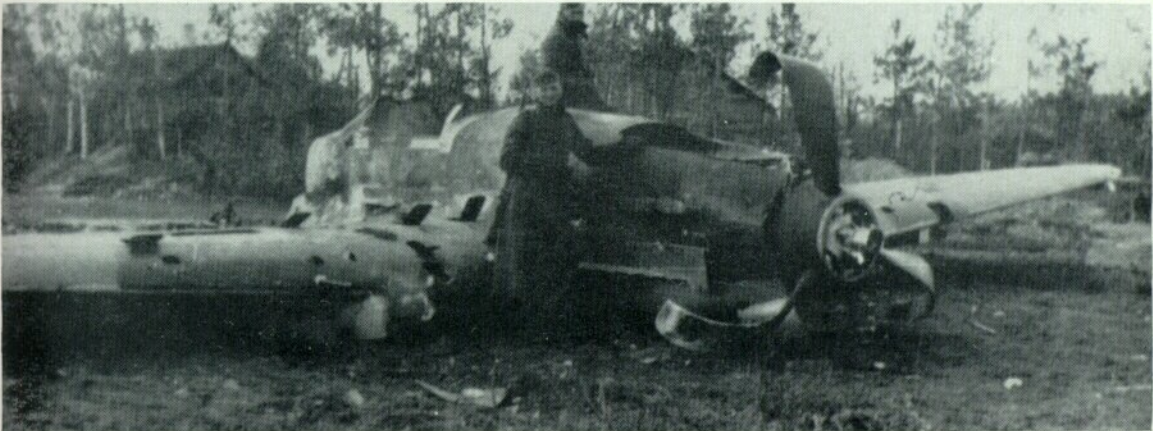
Below: Characteristically, this crashed II-2 has broken in two behind the cockpit; the fuselage centre-section remains relatively undamaged despite severe punishment to the other sections of the aircraft.
