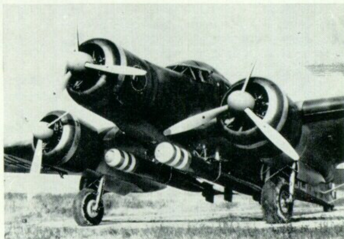
Experimental installation of two torpedoes; trials at Gorizia in the spring of 1938 proved that the dual installation caused a marked deterioration in the Sparviero's performance.
