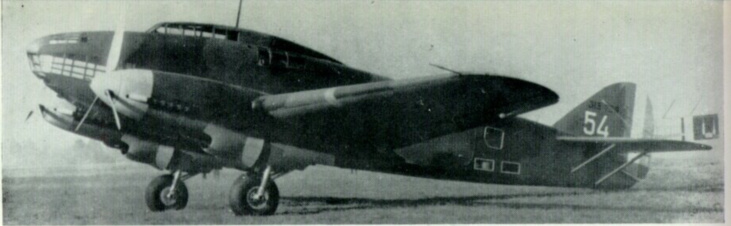
A Junkers Jumo-powered S.M.79JR of the Rumanian Air Force; licence production of this variant was carried out by Industria Aeronautica Romana at their Bucharest plant. (Photo: R. Ward Collection)
