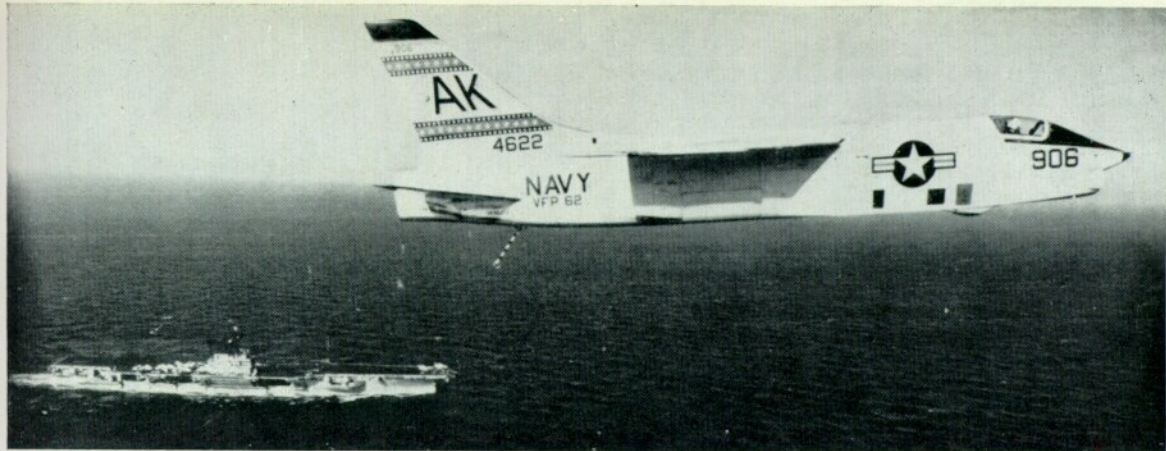
An RF-8A reconnaissance aircraft, No. 144622, of Navy Squadron VFP-62. The machine is seen here in the landing pattern over the U.S.S. Forrestal, with arrestor hook extended. (Photo: U.S. Navy)
