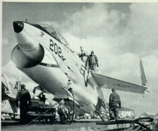
Left: This photograph of an F-8A on the flight deck of the U.S.S. Saratoga gives a good view of the knife-edge air intake. Note also the retractable step and the gun-camera window in the side of the plastic nose-cone; later versions had this installation repositioned on the underside of the cone. (Photo: Chance Vought.) Right: Detail view of the "Mighty Mouse" 2-7.5 in. rocket pack installed in the F-8A, B, C, and D variants.
