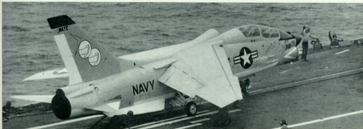
The sole two-seater Crusader trainer made ready for launching on the port catapult of the U.S.S. Independence . Note "Dual Control" fin emblem.
