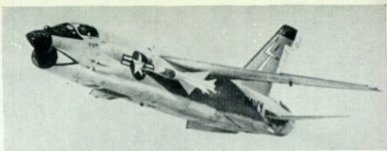
An F-8E in flight with the French Matra R-530 missile on the fuselage pylon.
