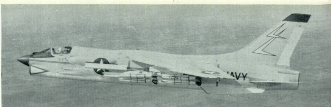
F-8E 149159 with underwing bomb load and Zuni rockets on the fuselage stations.
