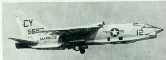
A reconnaissance Crusader of VMCJ-2, 145623, with retro-fitted ventral fins.
