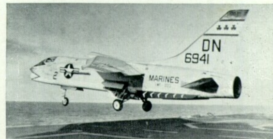
An F-8C, 146941, of VMF-33 during launching by steam catapult from U.S.S. Forrestal ; this photo was taken during the carrier qualification trials in the Atlantic.
