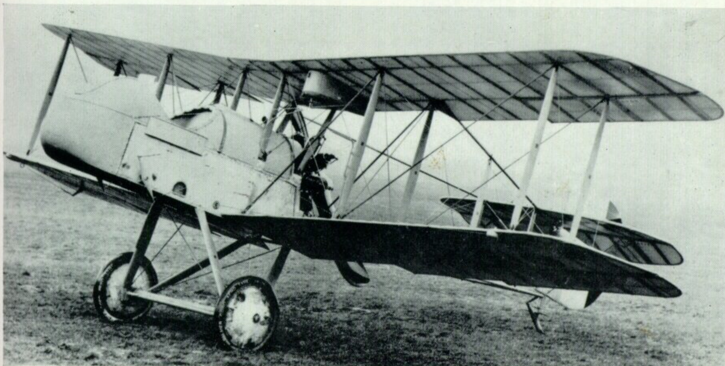
Four aspects of No. 5943, a production D.H.2 of the first batch. These aircraft had longer ailerons than those of the prototype, and the gravity tank was, originally at least, mounted under the port upper mainplane.
