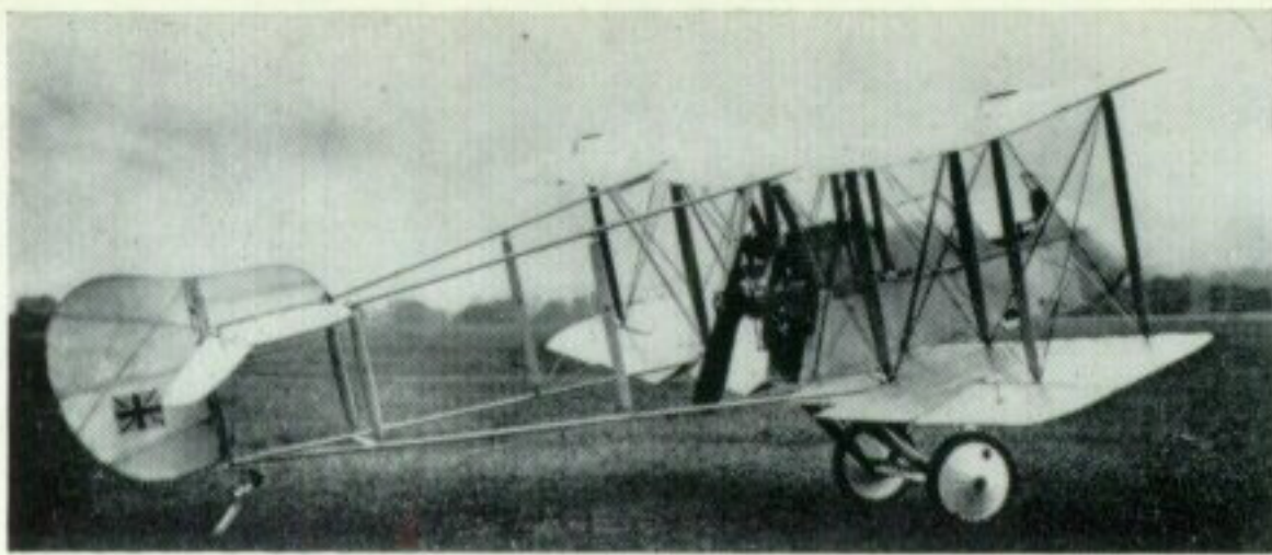
This three-quarter rear view of the prototype shows that only the port side of the forward decking was cut away to accommodate the gun-mounting. At this time there was no national marking on the upper surface of the wings.
