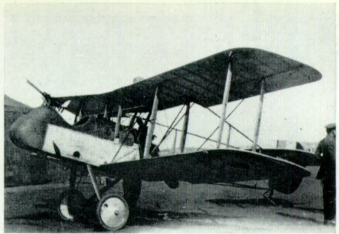
On this D.H.2 the windscreen was mounted on the rear of the Lewis gun, which is seen partly elevated.
