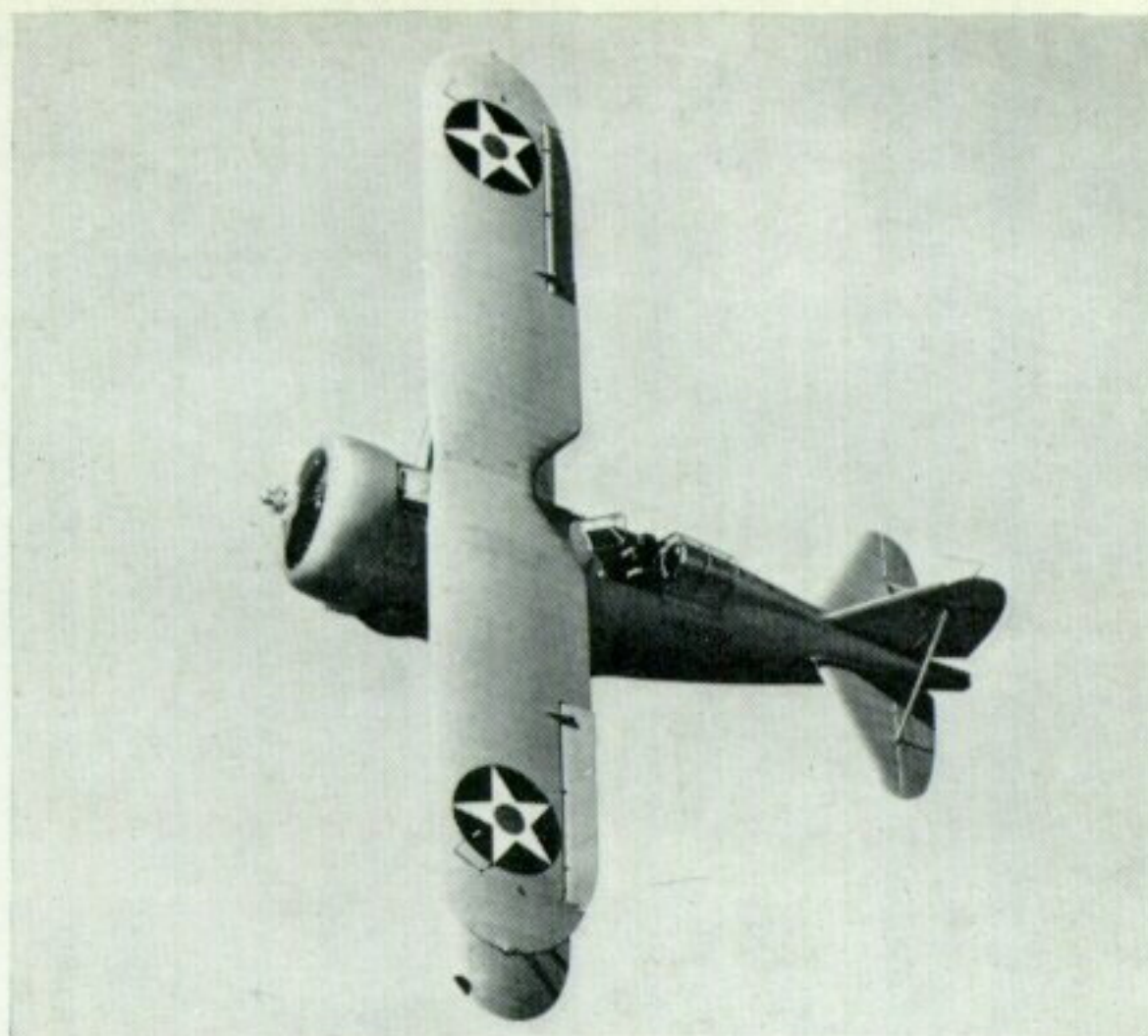
F3F-3 (1463) in slow roll, showing wing plan; formation lights just outboard of star insignia. Photographed 7th April 1939 at Anacostia. (Photo: U.S.N. Archives 464996)
