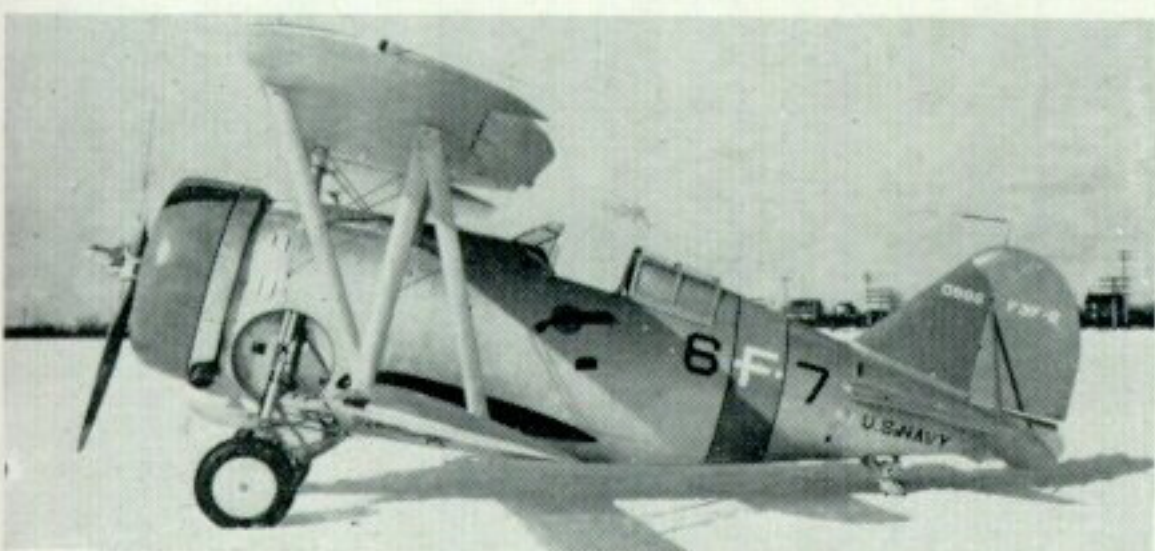
F3F-2 (0986) factory fresh at Bethpage, Long Island, before delivery to VF-6. Note louvre above leading edge of stabiliser designed to reduce CO content in cockpit.
