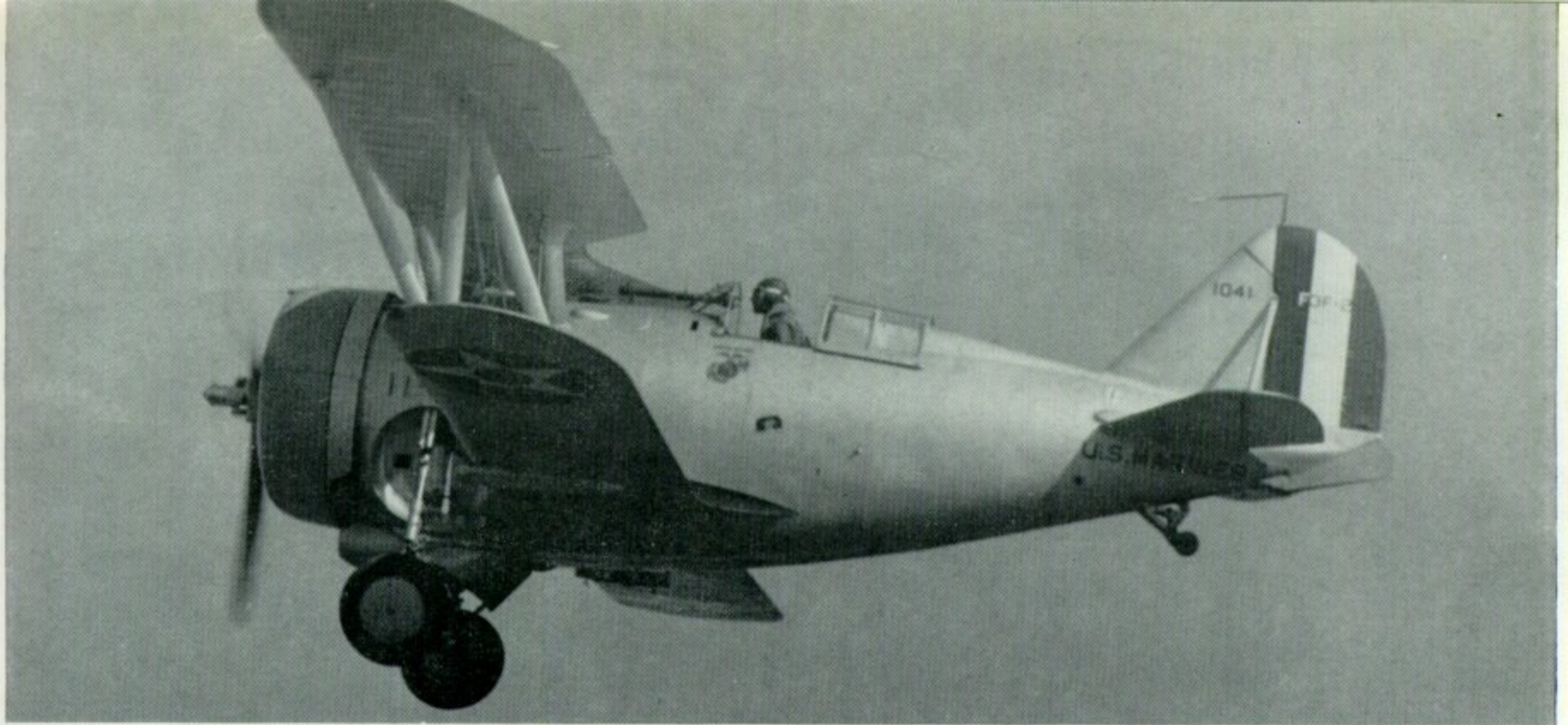
F3F-2 (1041) from VMF-1 coming in to land at the 1938 National Air Races, with pilot's seat cranked up and stabiliser cranked down; compare oleo leg extension with ground photos. Note bomb racks on opposite sides to usual arrangement. A small after carrier approach light is just visible between A and R of MARINES; comparison of photos points out the smaller bulge over the .30 calibre weapon than over the starboard gun. (Photo: Jim Tenety)
