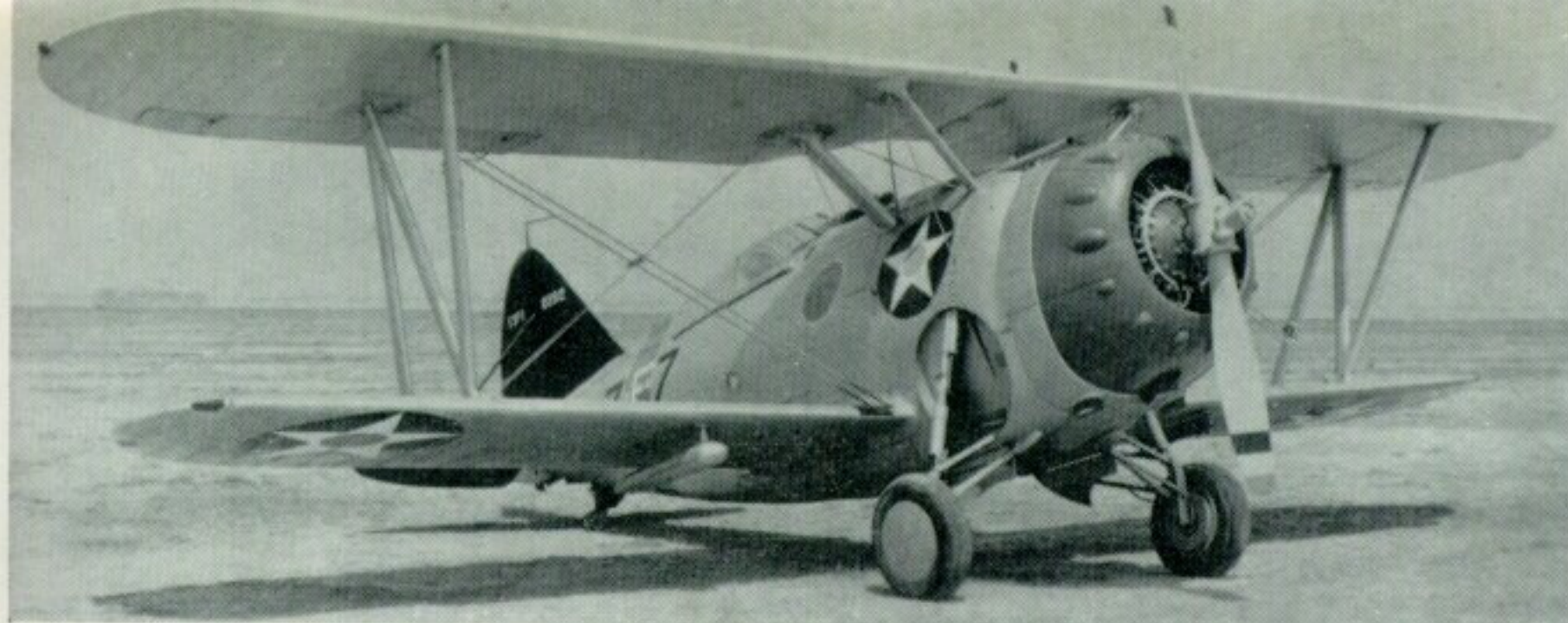
7-F-7 with the black-painted tail of U.S.S. Wasp aircraft, and chrome yellow paint carried under the leading edge of the wing to prevent airflow disturbance at division line. This machine, F3F-1 (0262), carries neutrality patrol star, and a Mk. XLIII bomb rack under starboard wing.
