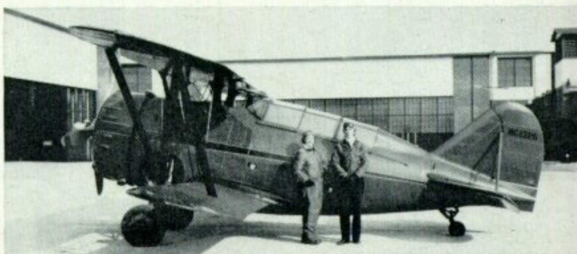
Grumman company hack and demonstrator. The upper wing of this G-32A design was flown on F3F-2 (1031) before conversion to show landing performance with flaps. (Photo: Grumman)
