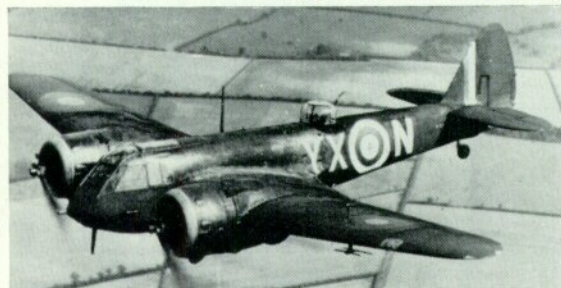
Mk. IF of No. 614 (County of Glamorgan) Sqn. with A.I. Mk. III radar.
