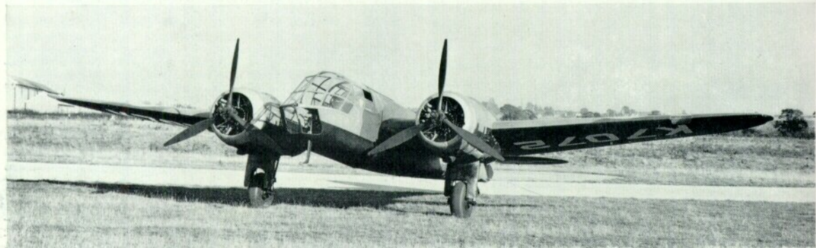
Below: Two views of Blenheim I K7072 after modification to Type 149 Bolingbroke I prototype by lengthening of nose, Filton, October 1937. Nose was subsequently re-designed.
