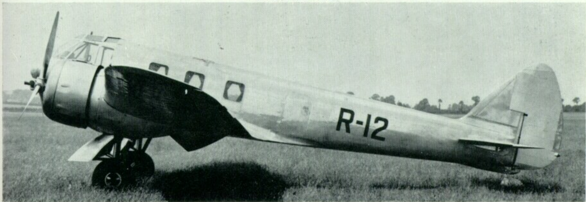
Type 142 at Filton. It first flew with four-bladed fixed-pitch wooden airscrews but is here seen after being fitted with three-bladed Hamilton-Standards.
