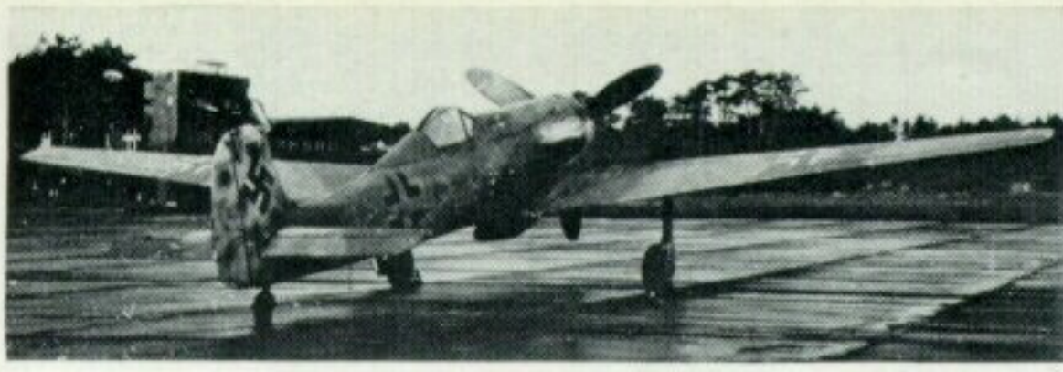
This view of a pre-production Ta 152H-0 shows to advantage the high aspect ratio wings of this high-altitude interceptor.
