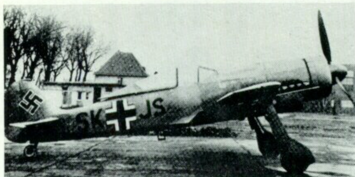
Fw 190V-13 (W.Nr.0036) coded S K + J S, was the first prototype of the proposed Fw 190C series; the engine was a 1,750-h.p. DB 603 A.
