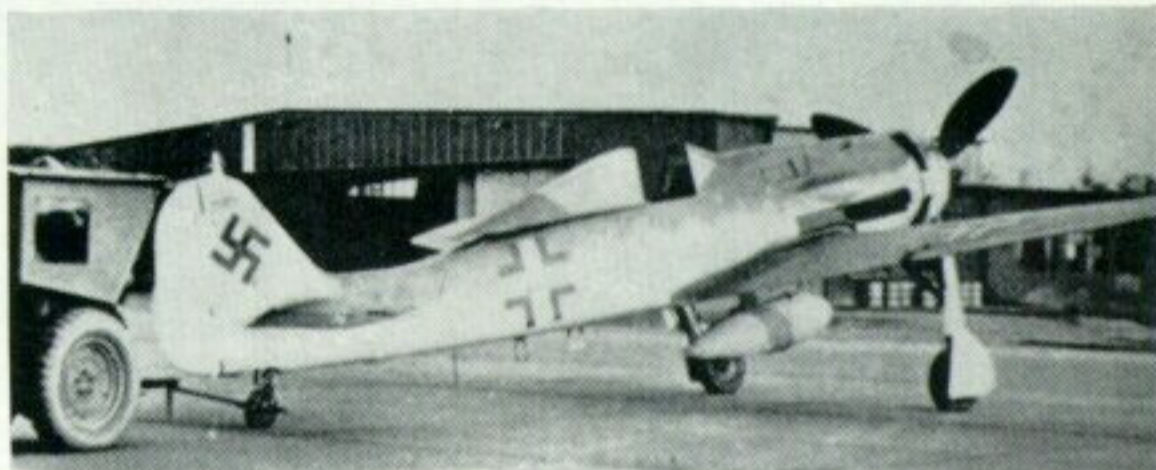
Three-quarter rear view of a D-9 with 300-litre drop tank. Absence of unit markings on a machine finished in standard camouflage and national insignia probably indicates a production aircraft undergoing manufacturer's tests prior to delivery to the Luftwaffe. (Photo: H. J. Nowarra)
