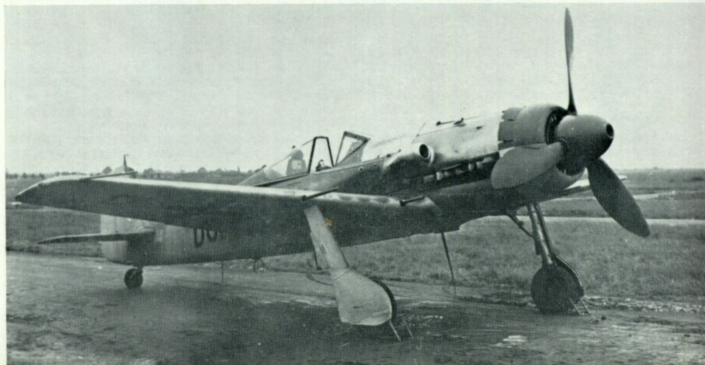
Second prototype for the operational D-9 and D-10 series was the Fw 190V-53 (W.Nr.170003). Note the distinctive engine cowling and propeller unit, with paddle-bladed airscrew. (Photo: H. J. Nowarra)
