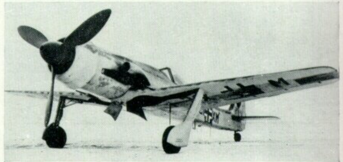
The Ta 152C-0/R/11 pictured on page 3 of this Profile, an all-weather fighter version of the pre-production C series. This view probably captures the distinctive lines of the later Focke-Wulf fighters better than any other existing photograph. (Photo: Imperial War Museum)
