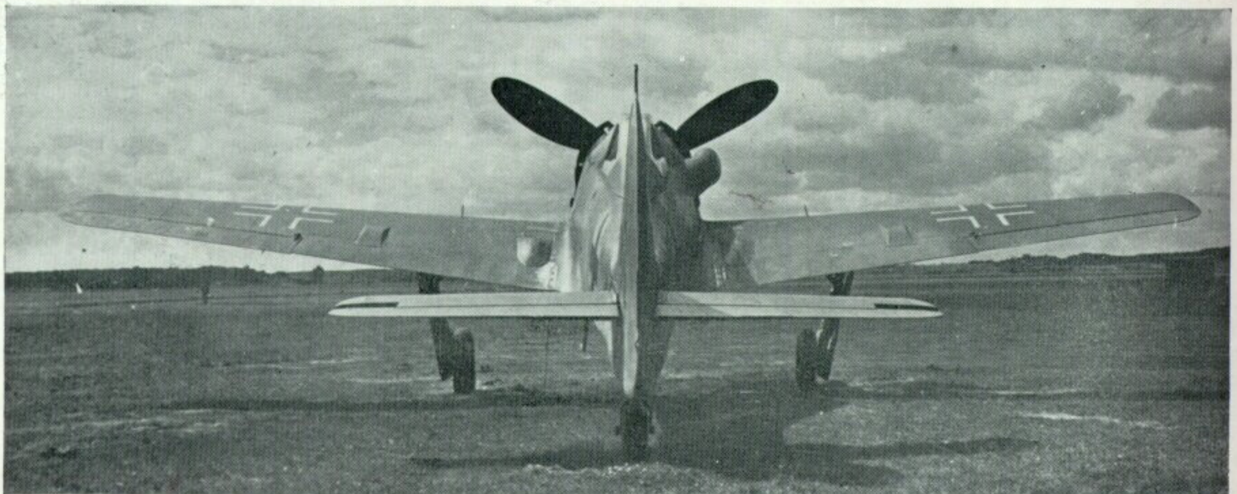
The prototype for the Fw 190D-11 was the V-56 (W.Nr.170924). Visible in this rear view are the small horns protruding above the inner wings, indicating undercarriage position.
