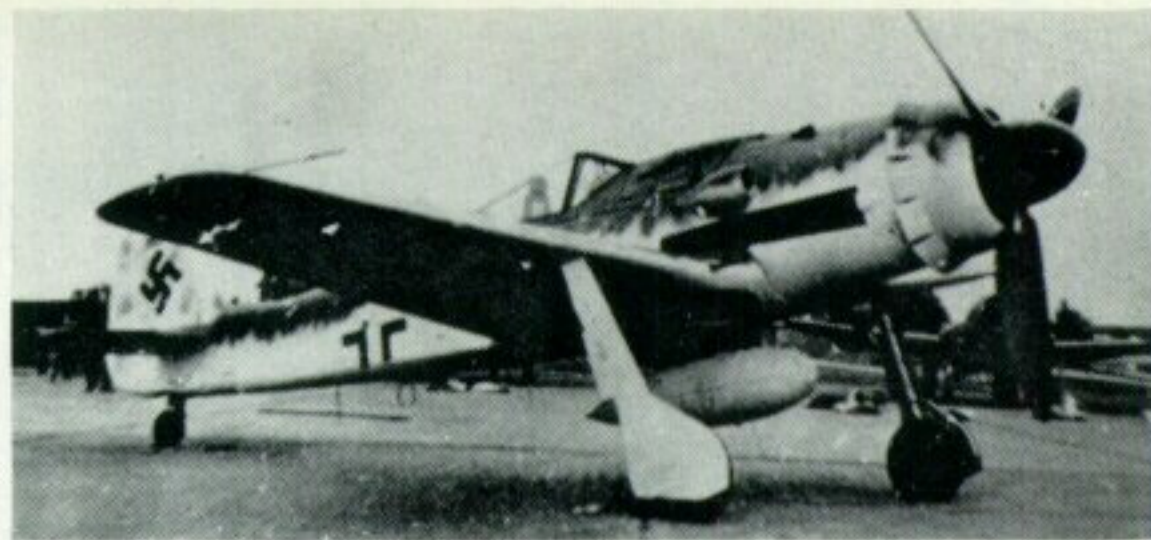
An early production Fw 190D-9, with 300-litre drop tank under the centre-section. (Photo: H. J. Nowarra)
