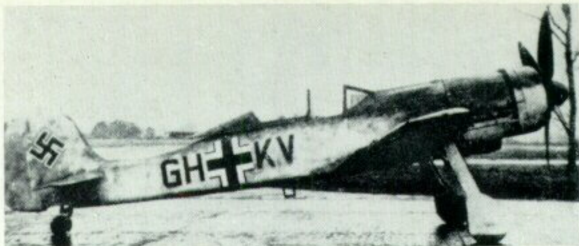
The Fw 190V-32/U1, a modification of the old V-32, was a forerunner of the Fw 190C. The machine was unarmed, and power was provided by a DB 603 G engine.
