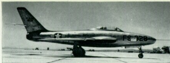
The URF-84F prototype 51-1828, with sliding canopy. (Photo: Bowers' Collection)
