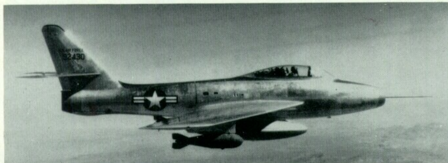
Briefly designated YF-46A, the swept-wing prototype 49-2430 is seen here with external load. (Photo: Republic)
