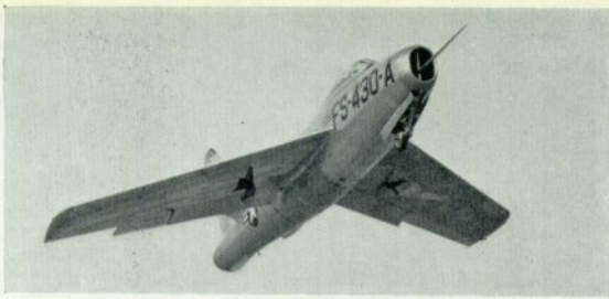
The prototype after being rebuilt with the British Sapphire engine. (Photo: Republic)
