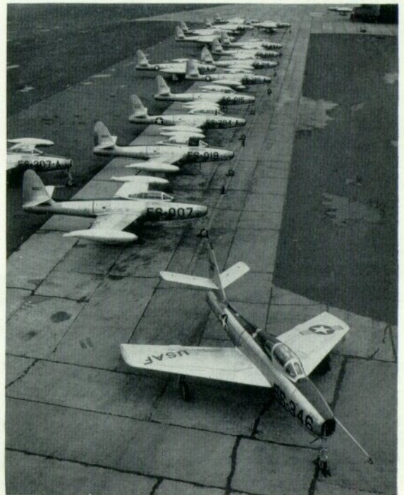
Contrast the first F-84F-1 with the line-up of F-84G-11 Thunderjets. (Photo: Republic)
