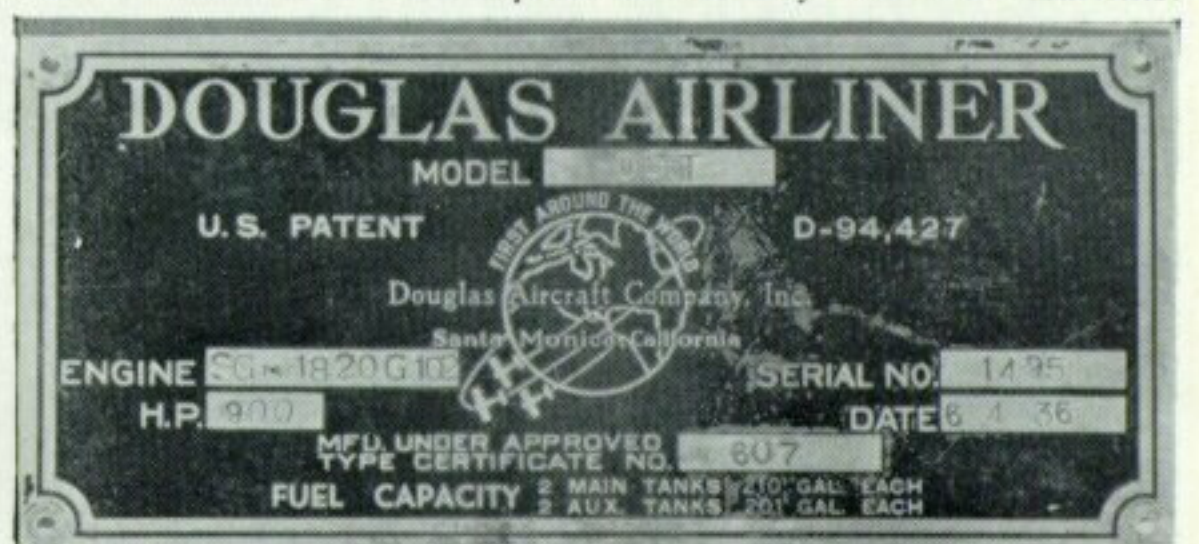
Maker's plate of the second DC-3 built, a DST model c/n 1495, built 4th June 1936. Actual plate now held by William T. Larkins.
