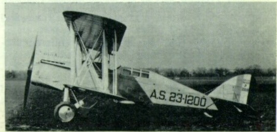
Left: DH-4B stationed at McCook Field for use as an engine test bed. This one carries a twin-row British Armstrong-Siddeley "Jaguar" radial. (U.S. Air Force Photo). Right: The DH-4B-5 with two-seat rear cockpit fitted as a cabin. In its civil version this was called "The Honeymoon Express". (U.S. Air Force Photo).
