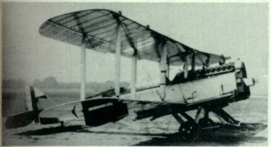
Left: Liberty Plane fitted with hydrovane and flotation gear developed at the Grain Naval Air Station in Britain. The top engine cowling was soon removed from all American DH-4's in service. (U.S. Air Force Photo).
