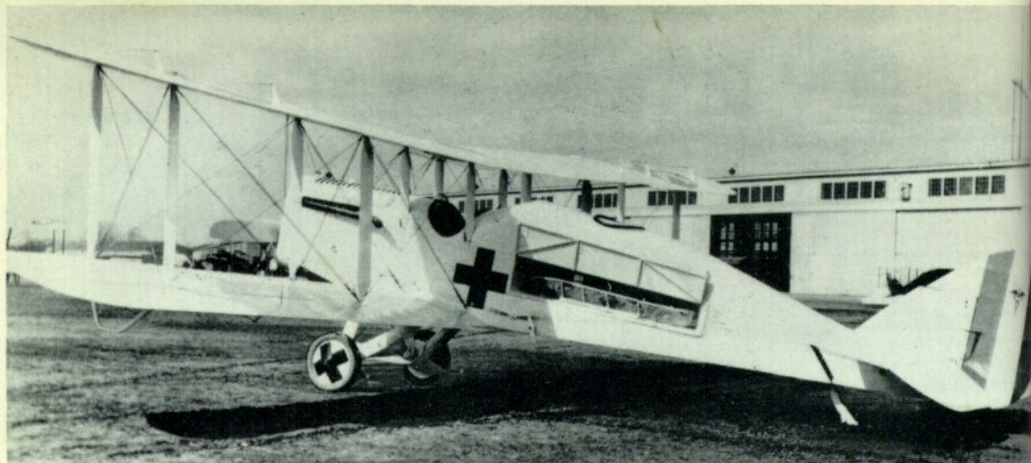
Liberty Plane modified to a two-litter ambulance under the designation of DH-4Amb-2. Second litter is stowed in top fuselage superstructure with access from starboard side. (U.S. Air Force Photo)
