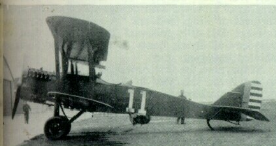
Atlantic-Fokker DH-4M-2K target with post-1927 Army tail stripes. Reel for tow cable is carried below the fuselage.
