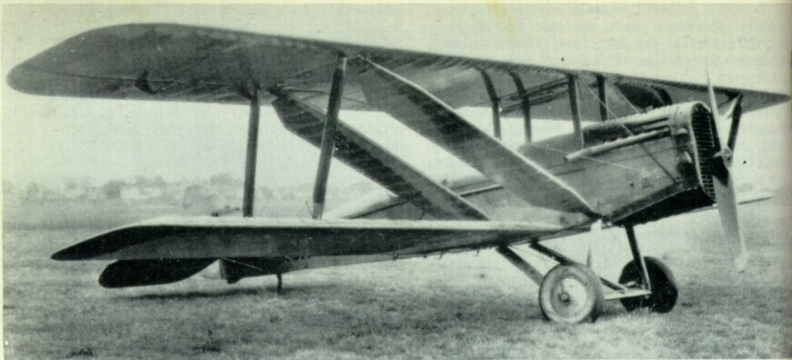
Another experimental mailplane conversion with high-lift wings developed by the Bellanca Aircraft Corp. The wide "Lifting" wings were a well-known feature of the Bellanca monoplanes for nearly two decades. (U.S. Air Force Photo)
