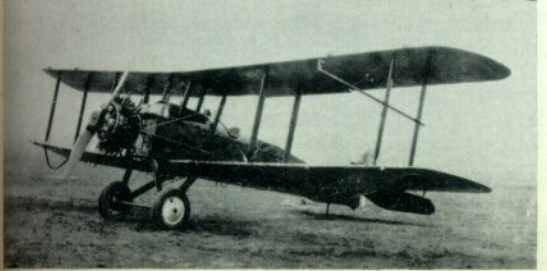
Left: DH-4B stationed at McCook Field for use as an engine test bed. This one carries a twin-row British Armstrong-Siddeley "Jaguar" radial. (U.S. Air Force Photo). Right: The DH-4B-5 with two-seat rear cockpit fitted as a cabin. In its civil version this was called "The Honeymoon Express". (U.S. Air Force Photo).
