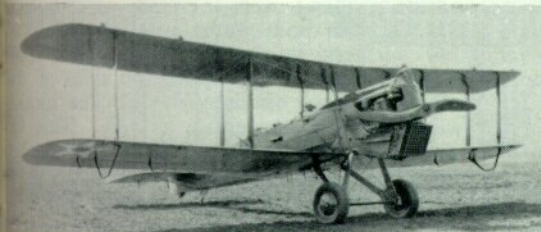
The DH-4M-2's were built by Fokker in his new American plant, known as the Atlantic Aircraft Corp. This is DH-4M-2S with turbo-supercharger.
