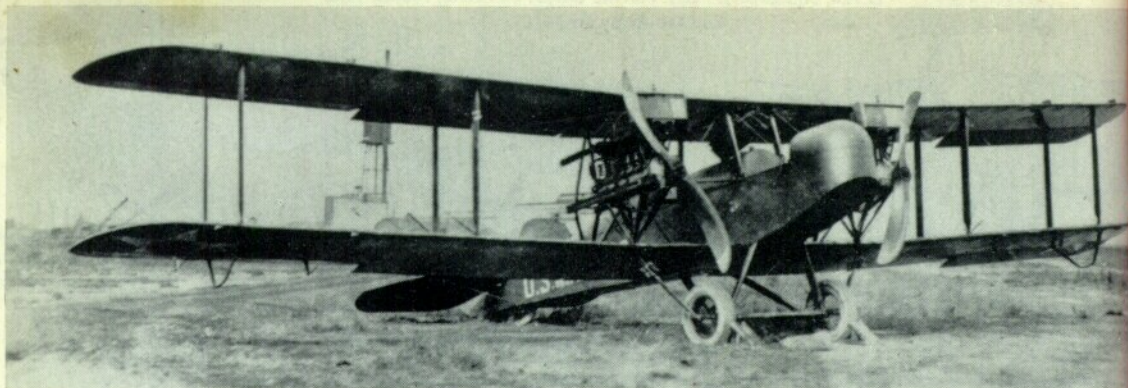
Short-lived twin-engine version of the DH-4 mailplane, this one powered with two Hall-Scott L-6 200 h.p. engines.
