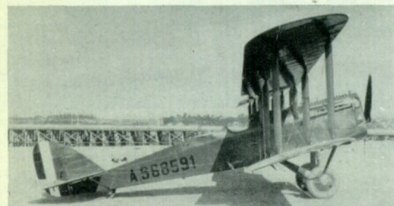
The second XDM-4H built by the Boeing Airplane Company, fitted with the original wooden DH-4B undercarriage. (Photo: The Boeing Company)
