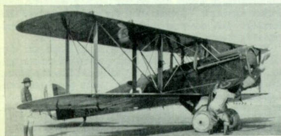
DH-4B of 91st Observation Squadron rigged for racing. Double flying wires have been taped over, the wing dihedral reduced, the front cockpit covered over. (courtesy James A. Morrow)
