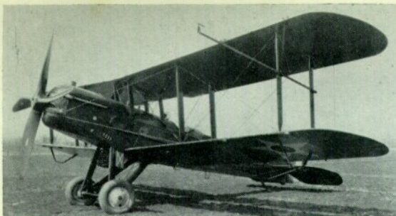
The single DH-4BS, specially adapted for high-altitude flights with a turbo supercharger, special geared-down Liberty engine, and extra long undercarriage legs to accommodate the large-diameter low-speed propeller. (U.S. Air Force Photo)
