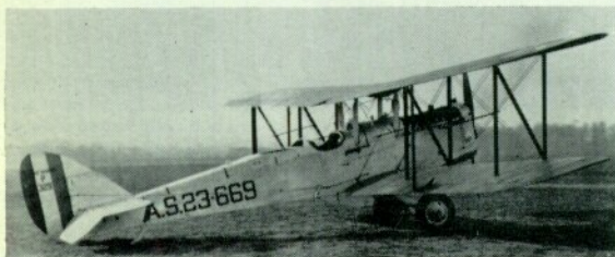
Standard DH-4B conversion as accomplished by the Gallaudet Aircraft Corp. but fitted with the improved wings of the Loening COA-1 amphibian. (U.S. Air Force Photo)
