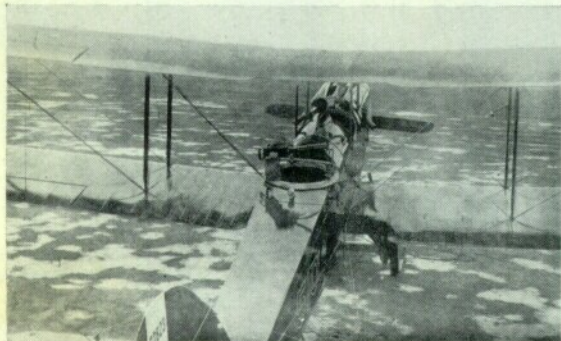
Cockpit details of the Liberty Plane. Normal armament was two Marlin machine guns for the pilot and two Lewis guns for the observer. (Photo: courtesy Gordon S. Williams)
