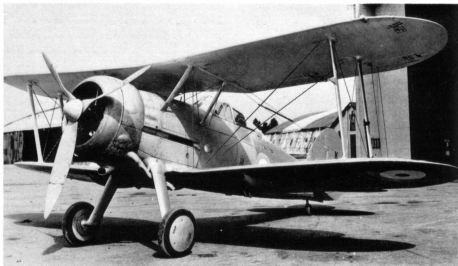
This Gladiator I, K7964, underwent prolonged trials with Fairey metal 3-blade propellers of various pitches in conjunction with different reduction gear ratios in efforts to arrive at the best take-off and climb performance. It is seen here at Martlesham Heath. (Photo: Imperial War Museum, Neg. No. MH5725)
