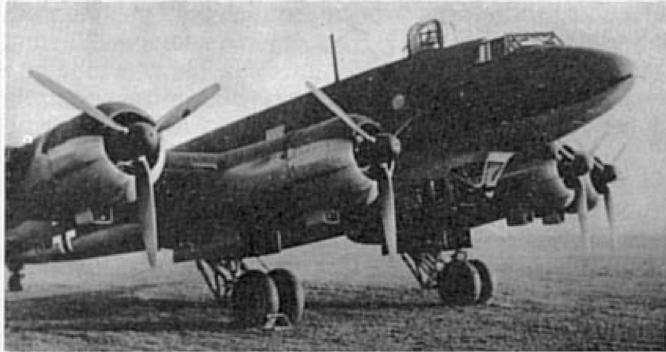
General nose lay-out of the C-3/U1 variant; note that armament has been removed. (Photo: H. J. Nowarra)
