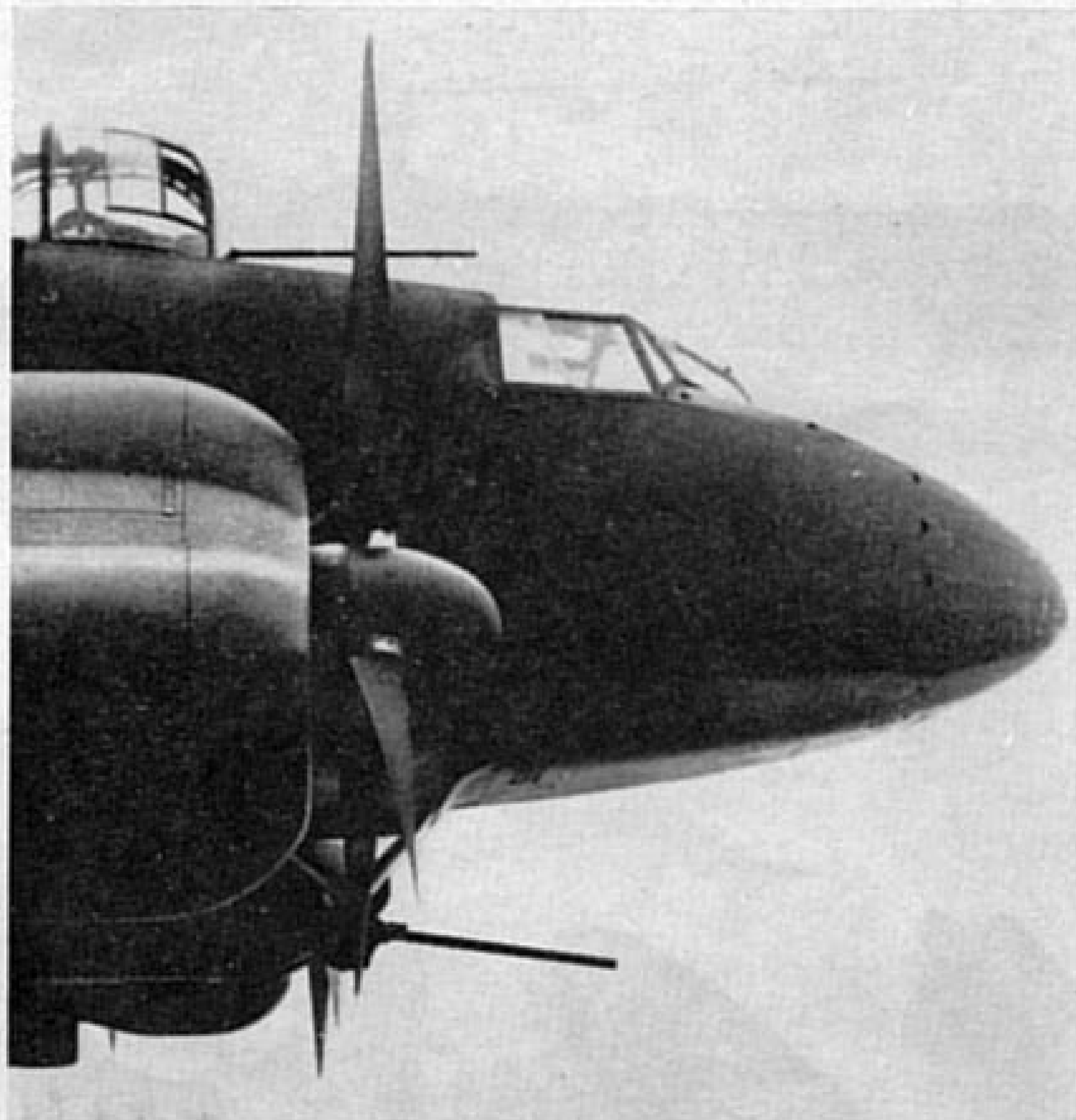
Nose close-ups of the Fw 200C-3/U1, showing the 15 mm MG 151 cannon in the dorsal turret and the 20 mm MG 151/20 cannon in the forward ventral position.
