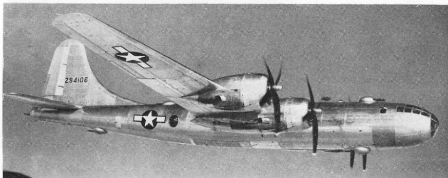
The four-gun upper forward turret of the B-29A-30BN is just visible in this photograph of 42-94106.
