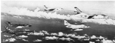
A Scimitar about to be refuelled by a A-4C of VA-83 while a Sea Vixen positions itself for a refill from an A-3B from VAH-5. RF-8A from VFP-62 observes.
