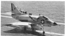
An A-4C from VA-66, tanker configured, taxiing forward for positioning for a catapult launch.
