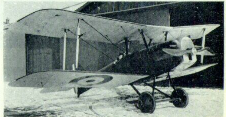
Captain Albert Ball in A4850 at London Colney. The modifications to this aircraft allowed the pilot to sit lower down in the fuselage.
