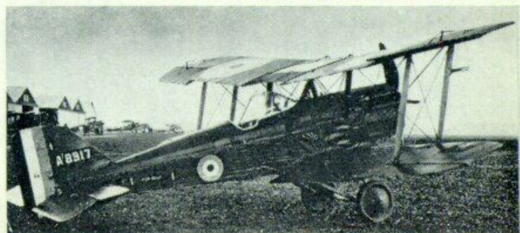
A8917, second of the two S.E.5's completed without armament. The drain bowls for the tanks in the centre-section leading edge can be seen in the \frac{3}{4} -front view; the overflow pipes are visible in the other.
