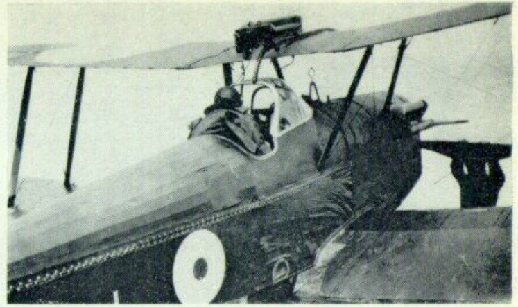
On the original production S.E.5 the pilot sat high, as seen here in this photograph of A8903 being started up.
