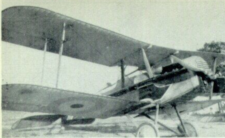
This S.E.5 of No. 60 Squadron was flown by Captain W. A. Bishop. Painted in the early style adopted briefly by No. 60 Squadron, it had a blue nose and blue diagonal stripe on the rear fuselage. Long exhaust pipes were fitted, and the aircraft evidently had the centre-section leading-edge gravity tank.
