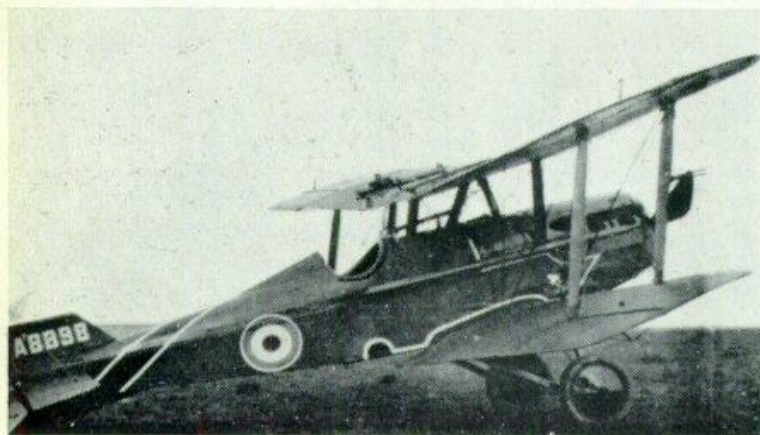
The first S.E.5 of the second production batch, A8898, after its transfer to No. 60 Squadron. It had like Bishop's aircraft, acquired long exhaust pipes.
