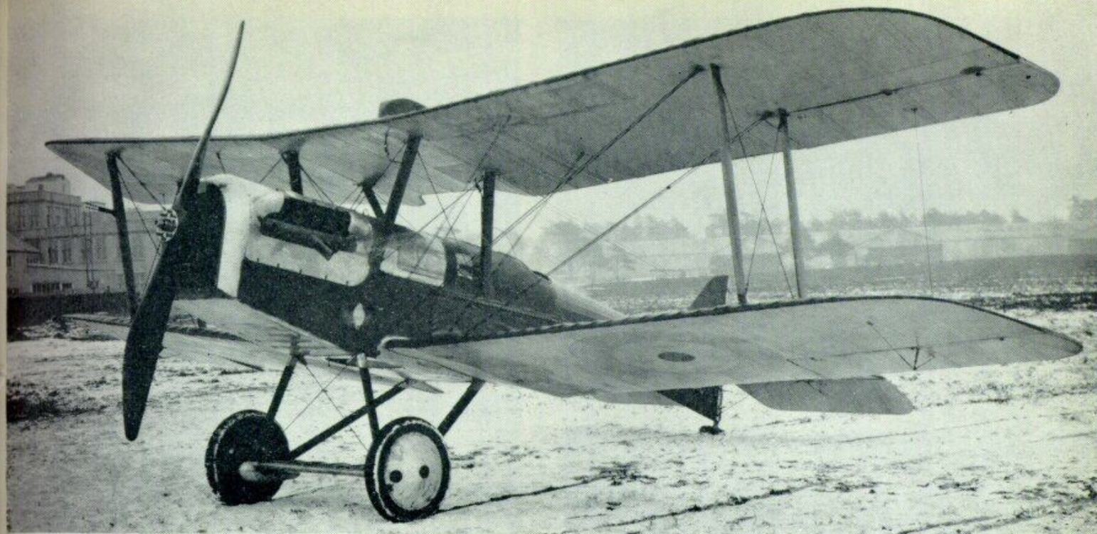
Above and Below: This aircraft was long believed to be the first prototype, but it has recently been established that these photographs were made at Farnborough on 15th January, 1917. This indicates clearly that this S.E.5 was in fact the third prototype A4563 in its original form without armament. It had the same type of windscreen as A4561 and the same transparent panels in the sides of the top decking ahead of the cockpit. The patched fabric on the inboard leading-edge portion of the port upper wing shows plainly where the original gravity tank was removed.
