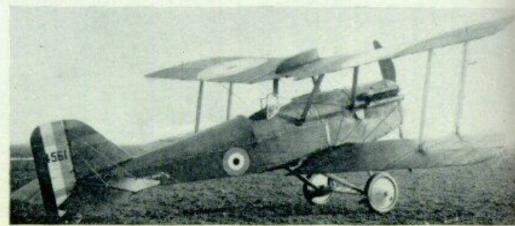
A4561 after modification with overwing gravity tank, Vickers gun, side extensions of the windscreen, revised exhaust manifold and new centre section with enlarged trailing-edge cut-out. (Photo: Imperial War Museum)
