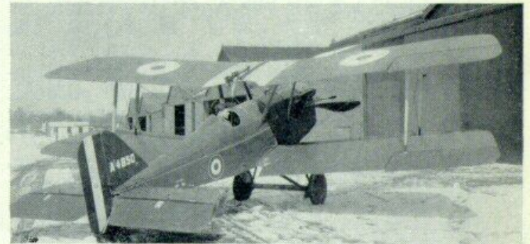
Captain Albert Ball in A4850 at London Colney. The modifications to this aircraft allowed the pilot to sit lower down in the fuselage.
