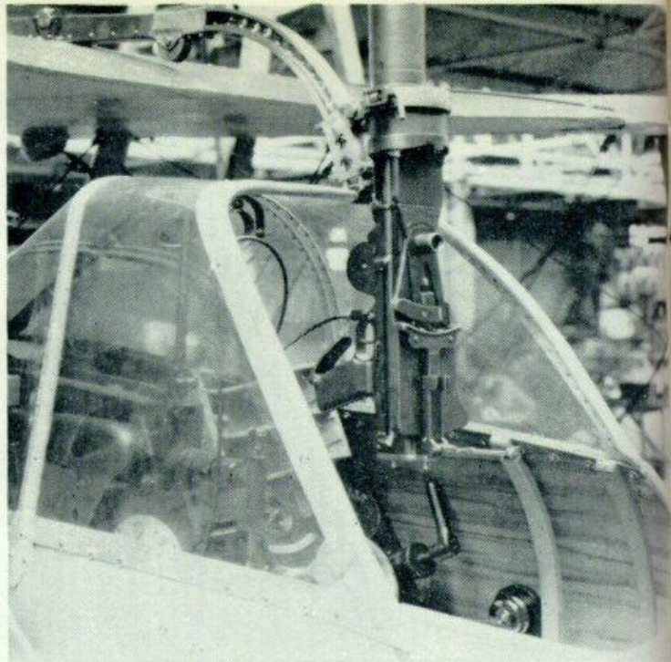
The large windscreen and cockpit details of a production S.E.5, showing the Lewis gun at the extreme positions permitted by the Foster mounting. (Photos: Crown copyright)
