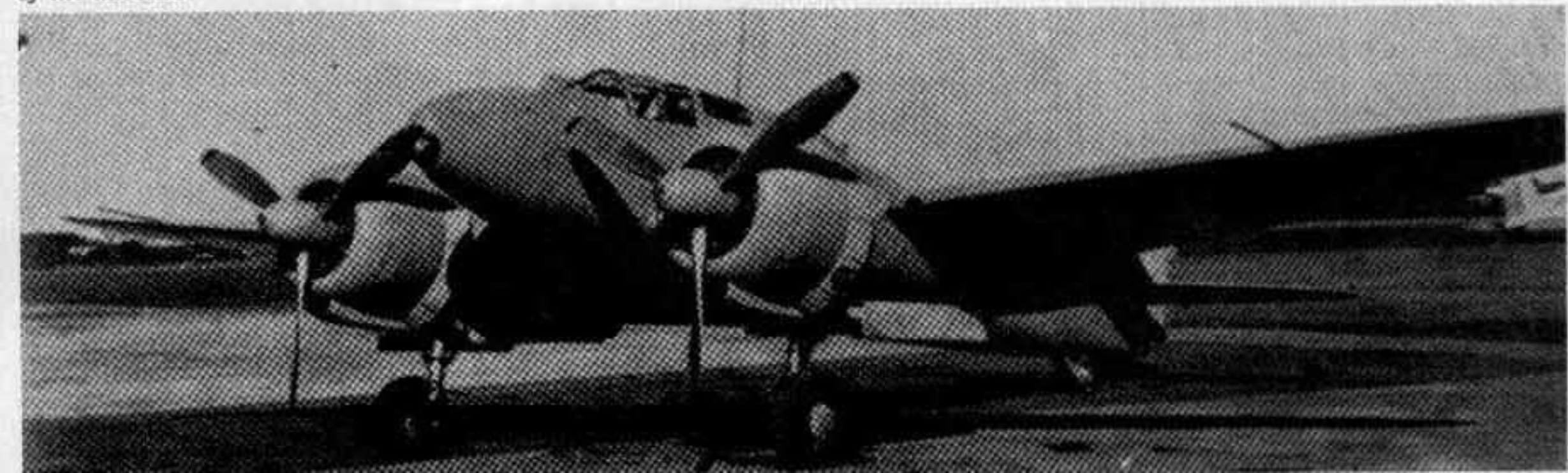
An improved Type 1 Ki-45 prototype with Ha-25 powerplants. Note the supercharger intake on the wing leading edge just outboard of the nacelles.
