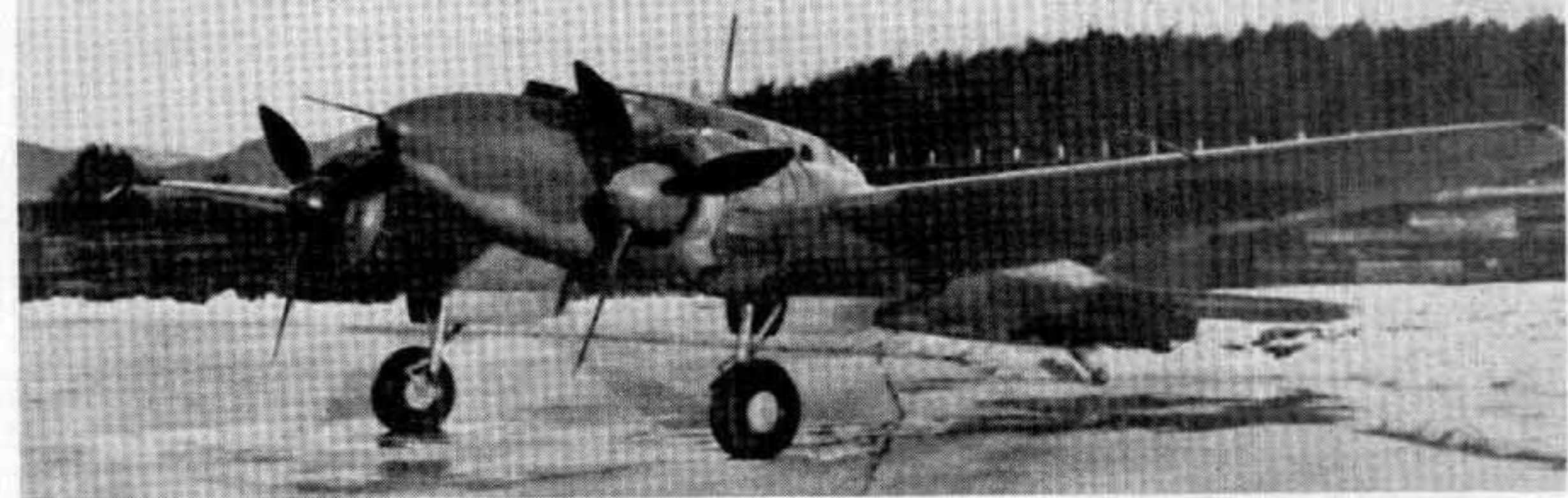
Second prototype, with closer-fitting cowlings and spinners added. The exhaust collector ring around the cowling leading edge characterises Ha-20b-powered aircraft.
