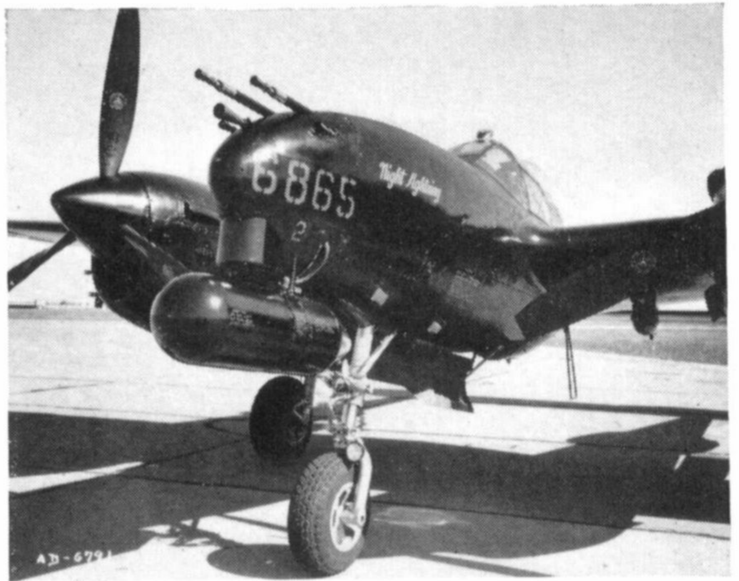
"Night Lightning" (44-26865) the first P-38M night fighter, modified from the P-38L-LO variant. Note A.S.H. radar "bomb" housing. (Photo: Lockheed)
