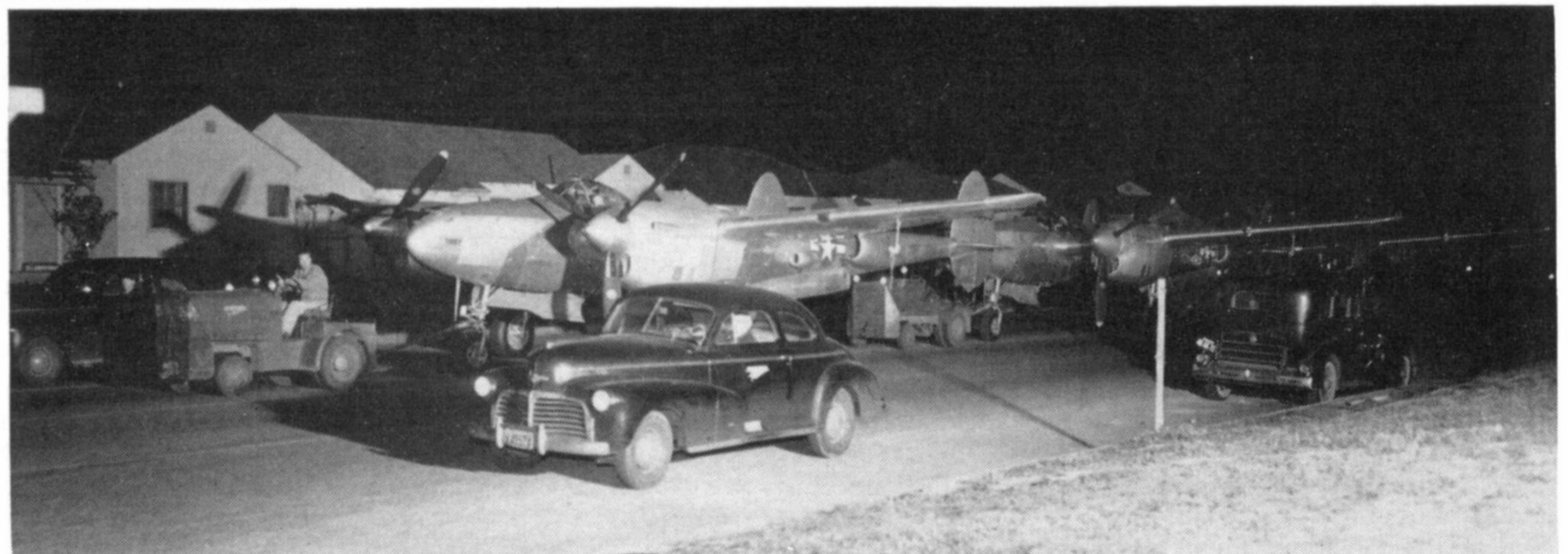
The unusual stage of P-38 production—an L-5-LO variant takes its night drive through the streets of Burbank, California, to the Lockheed Air Terminal. (Photo: Lockheed)
