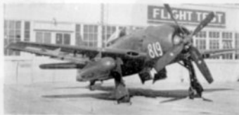
Left: One of the two prototypes for the radar-equipped F8F-1N, BuNo.94819 is seen here during evaluation at N.A.T.C. in the autumn of 1945, with a Grumman prototype radar nacelle installed. (Photo: U.S.N.). Right: BuNo.94873 at N.A.T.C. in April 1946, during flight development programme of the larger vertical tail which was needed to give adequate stability when the centreline tank was installed. Note rudder chord extension and absence of dorsal fin. (Photo: U.S.N.)
