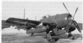
BuNo 90438, the second "production" Bearcat, shown at Bethpage in February 1945 during G.A.E.C. evaluation of various external store configurations. Shown here, upper to lower, are: 150 gal. centre line tank and two 1,000 lb. bombs; 150 gal. centreline tank and two 100 gal. wing tanks; 150 gal. centreline tank and two Mk. 1 twin .50 gun pods; two 11.75 inch Tiny Tim rockets. (Photos: Grumman)
