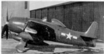
BuNo 90438, the second "production" Bearcat, shown at Bethpage in February 1945 during G.A.E.C. evaluation of various external store configurations. Shown here, upper to lower, are: 150 gal. centre line tank and two 1,000 lb. bombs; 150 gal. centreline tank and two 100 gal. wing tanks; 150 gal. centreline tank and two Mk. 1 twin .50 gun pods; two 11.75 inch Tiny Tim rockets. (Photos: Grumman)
