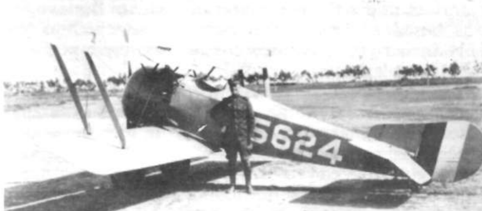
U.S. Navy HD-2 convert A5624 at North Island, late summer 1919. Note retention of early HD-2 enlarged rudder and generator mounted on lower port wing root.
