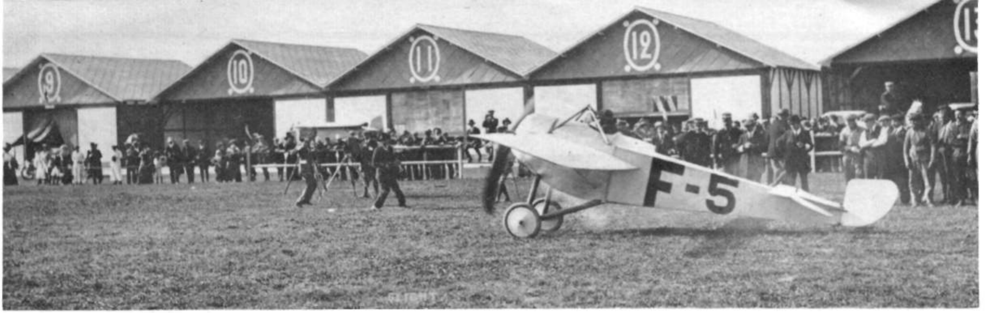
The Ponnier-Pagny Gordon Bennett racing monoplane of 1913, flown by Emile Védrynes at a speed of 197.5 km./hr (123.5 m.p.h.) (Photo: via Flight International)
