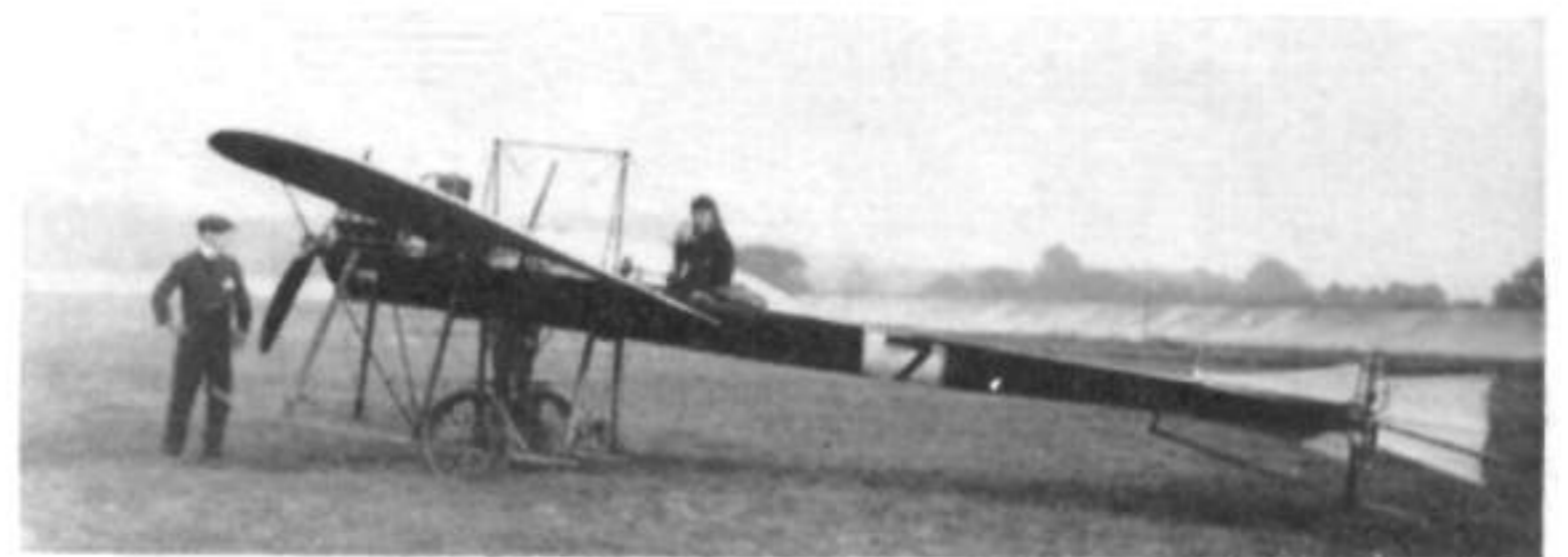
The graceful Hanriot monoplane of 1910 is here exemplified by Mr. A. C. Thomas's aircraft, possibly the only British-owned Hanriot of this type. It had a 35-h.p. E.N.V. engine and was photographed at Brooklands in October 1910, with E. Keith Davis in the cockpit. (Photo: Flight International)
