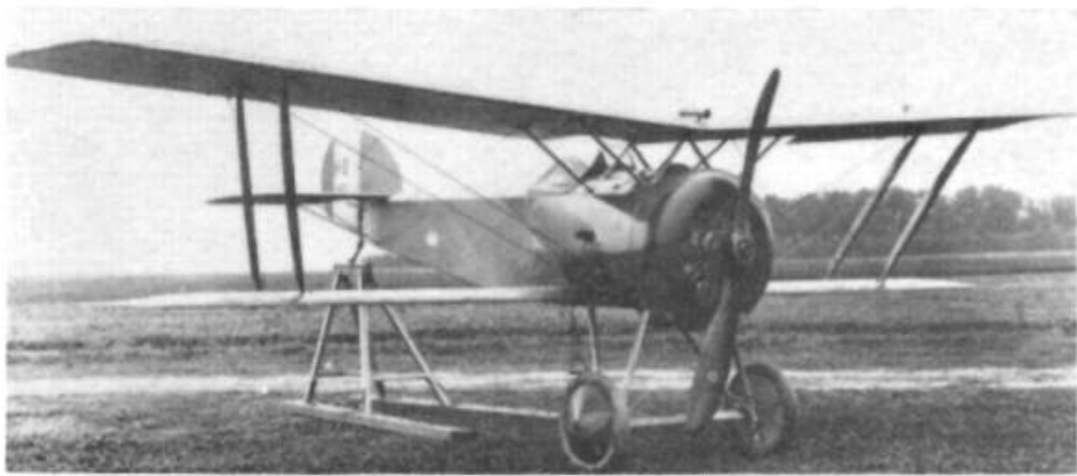
HD-1 No. 61 apparently in Belgian camouflage but with 130 h.p. Clerget engine and modified fin and horn-balanced rudder. (Photo: Imperial War Museum Q66274)
