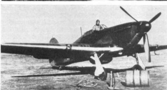
The Belgian Hurricane I's based at Schaffen at the time of the German invasion of May 1940 were almost certainly all British-built, though two licence-built aircraft are known to have been completed. These photographs are interesting in showing individual exhaust stubs (six per side) on some aircraft, but scarcely visible under the wings are the individual aircraft numbers (e.g. H under starboard wing and 22 under port, in five-foot deep characters). It is not known for certain whether the thistle emblem was carried by the 2 ème Escadrille in combat.
