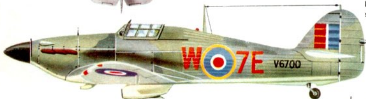
Hurricane I, P2992, of No 527 (Calibration) Sqdn., Hornchurch, 1943. Used for gun calibration, Thames forts, and Type I radar at Stoke Holy Cross, Orby and High Street. Doped with high-reflectivity paint. Rotal prop.
