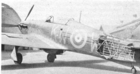
The ability of the Hurricane to withstand severe battle damage is well illustrated by this picture of a 615 (County of Surrey) Squadron aircraft which landed at Kenley after being hit in the rear fuselage by cannon shells and in the wing by machine gun fire. (Photo: F. K. Mason collection)
