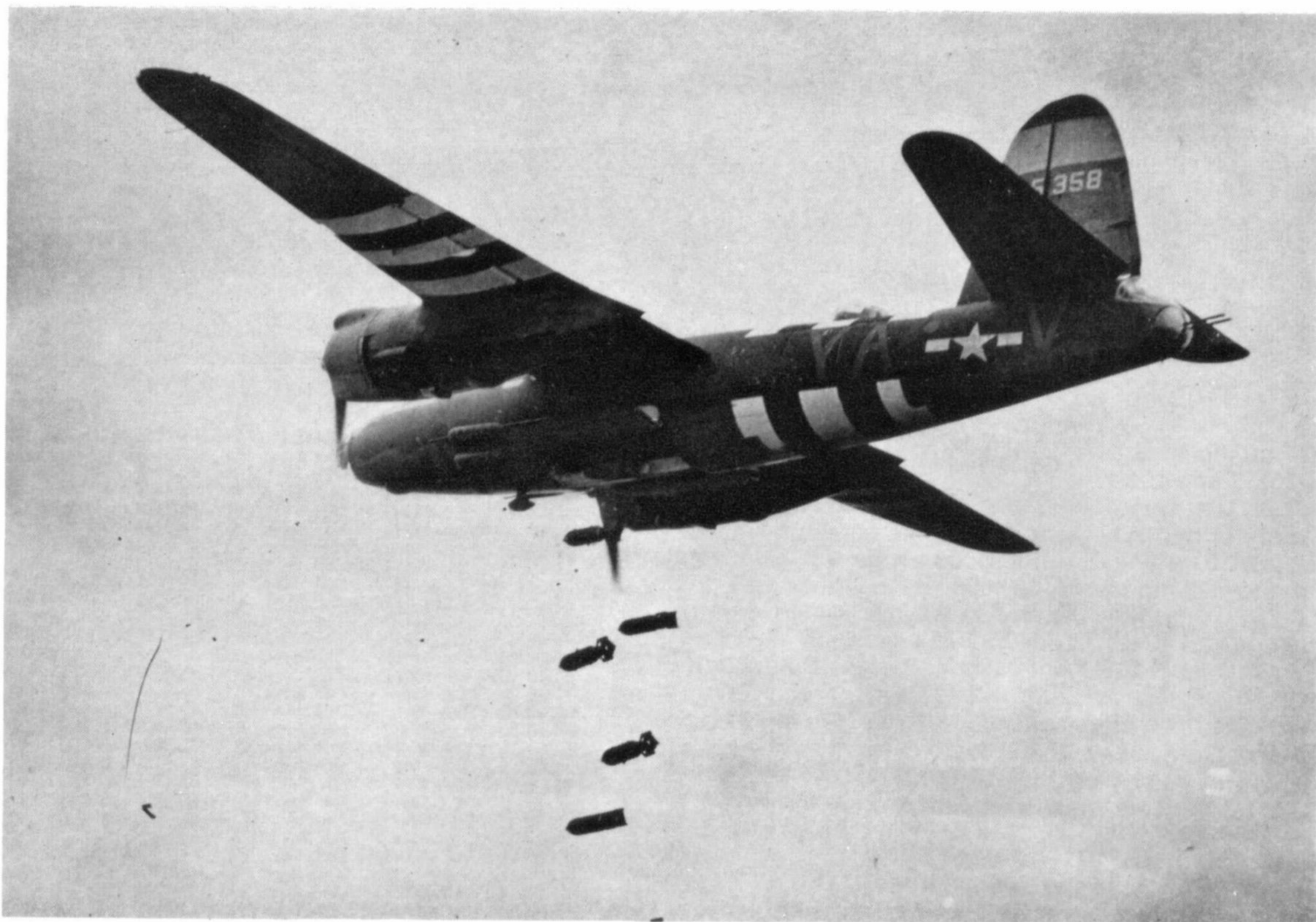
Note the folded bomb-doors of this B-26C-25, YA-V of the 555th Bomb. Sqdn., 386th Bomb. Grp. Normal bomb loads for 9th Air Force missions comprised eight 500 lb. or sixteen 250 lb. weapons; maximum short-range load was 5,200 lbs.
