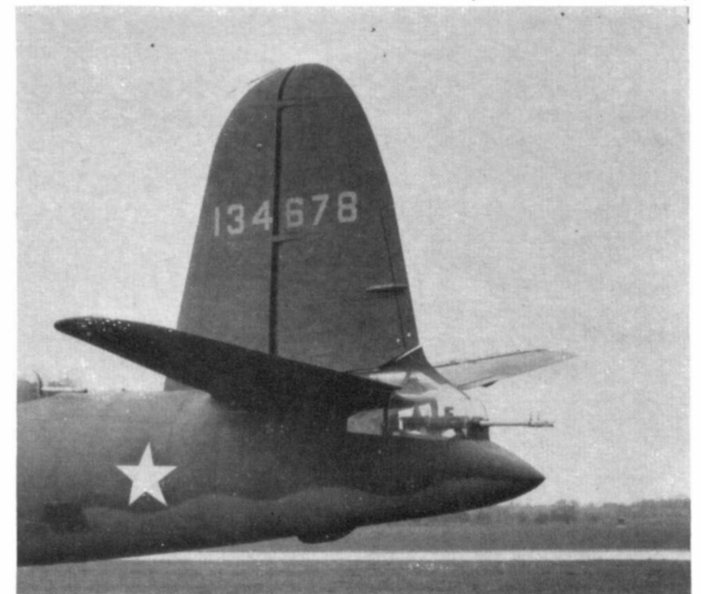
Twin .50 calibre tail guns of a B-26C-5-MO.
