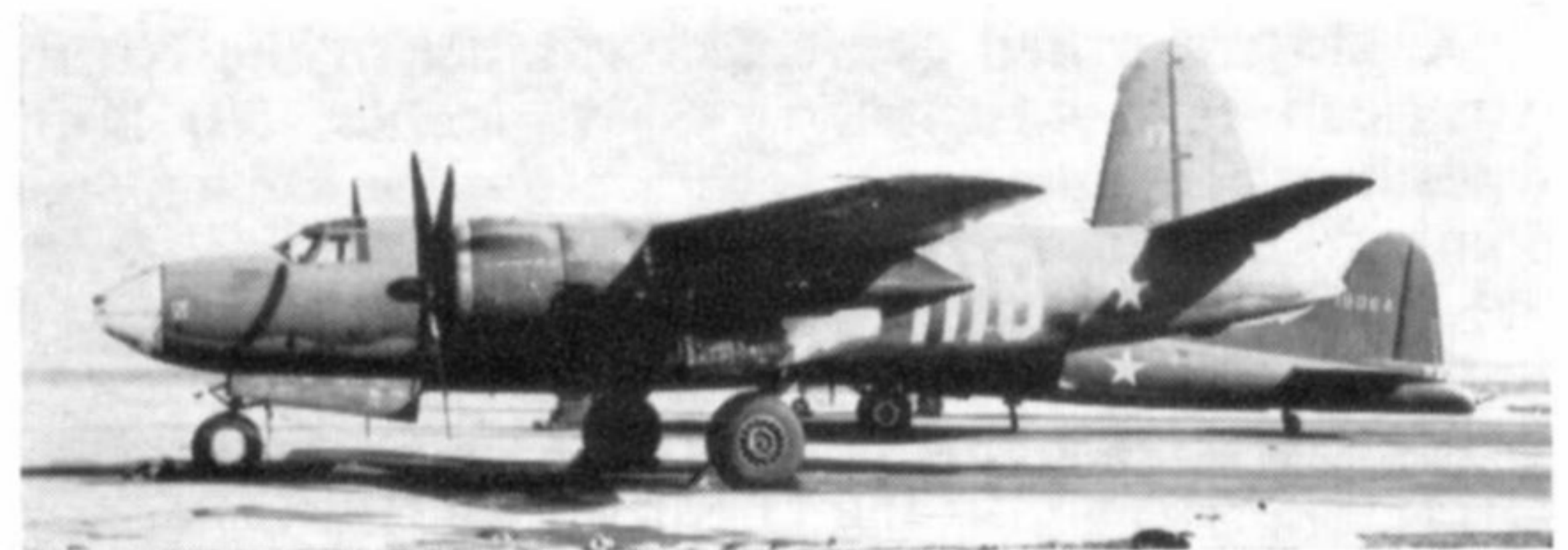
109 machines powered by the R-2800-39 Wasp were delivered as the B-26A-1. (Photo: Peter M. Bowers Collection)
