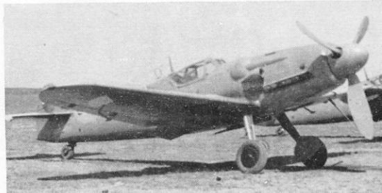
Jumo-engined Avia C.210 of the Czechoslovakian Air Force; note that the original Galland hood is still used. (Photo: Zdenek Titz)
