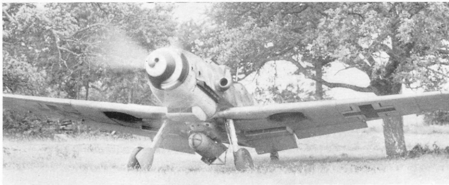
The Gustav runs up in its wooded dispersal point; this sequence was photographed in Russia during the summer battles of 1943. This illustration demonstrates effectively many of the characteristics of the Bf 109G series, including the narrow-track undercarriage, the streamlined air intake on the port side of the cowling, the shallow underwing radiators; and the popular spiral spinner motif, carried both as decoration and as an attempt to put air-gunnery off their aim.
