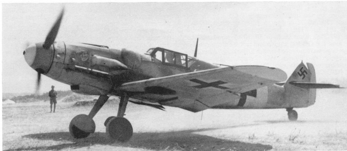
A Bf 109G-1 Trop. of I/JG 51 "Molders" on the South Russian Front. The penetrating dust which characterised Russian airfields in summer forced the installation of sand filters on aircraft in this theatre. Note the Geschwader insignia on the cowling.
