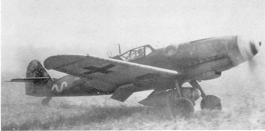
A late-model Bf 109G, probably a G-14, displays the tall tail and the clear-view Galland hood of the later variants. Cockpit canopy framing was severely reduced, and the armour plate behind the pilot's head replaced by a frame of bullet-proof glass. Note that although this photograph could not have been taken earlier than 1944, the early-style III Gruppe marking is still carried.
