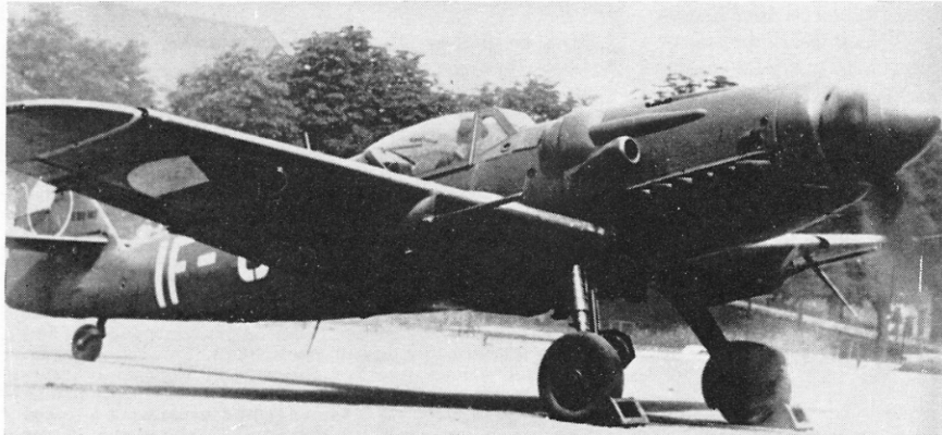
Mezec ( Mule ) was the name by which the Avia C.210 was known to Czechoslovak pilots; its handling characteristics were said to be vicious. Note that this aircraft has a new blown canopy. (Photo: Zdenek Titz)
