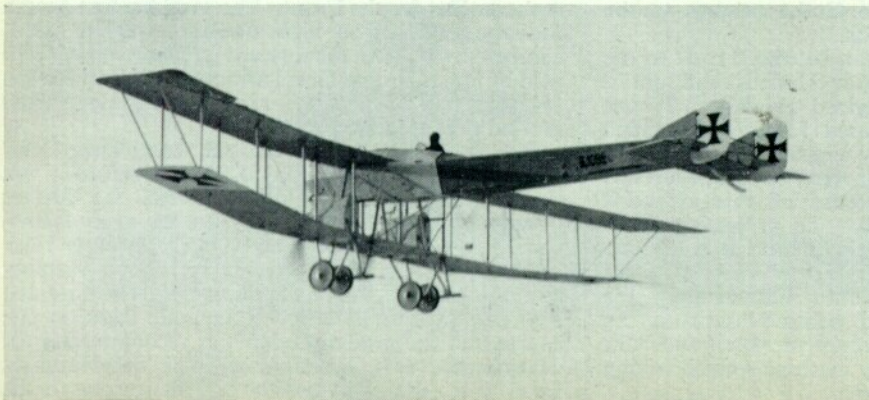
The B.1092/14 at Feld Flieger Abteilung 28 ; the cowlings have been removed for better cooling and new radiators installed. Note the "FU" monogram on the nose. This was the first German twin-engined bomber of the war. (Photo: Egon Krüger)
