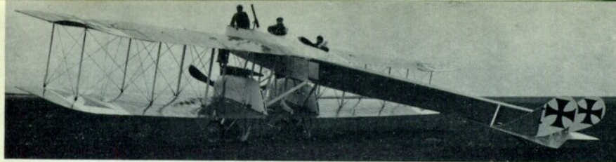
The Gotha G.I prototype note that the outer diagonal strut has been eliminated. Ursinus is in the centre cockpit, and the pilot in the rear position holds a "lucky" pig.
