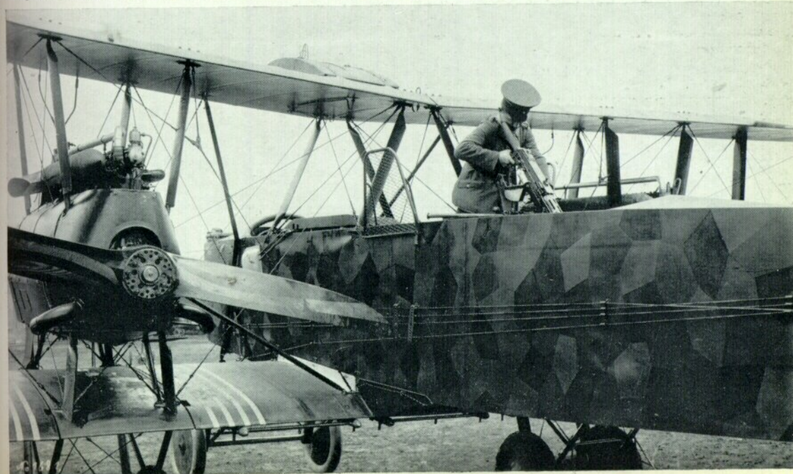
Left: The bomb rack for a single Carbonit bomb under the wing of a Gotha G.I. (Photo: W. Puglisi) Right: Gotha taken over by the Netherlands air service, seen here in Dutch markings in the L.V.A. workshops. The fin serial is 'LA 50'. (Photo: G. H. Kamphuis)
