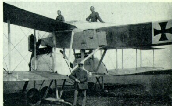
Gotha G.I, showing springs on undercarriage to ease landing shock when tail touched down. Ursinus trademark just visible on panel below cockpit.
