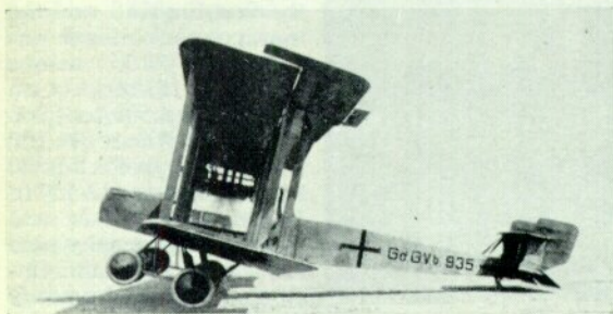
Below left: Gotha G.V modified to test simplified undercarriage structure. (Photo: von Röm)
