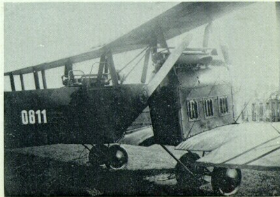
Gotha G.IV (LVG) 08.11, supplied to Austria in 1918, powered by 230 h p. Hiero engines. Note additional centre-section strut. (Photo: P. Bowers)
