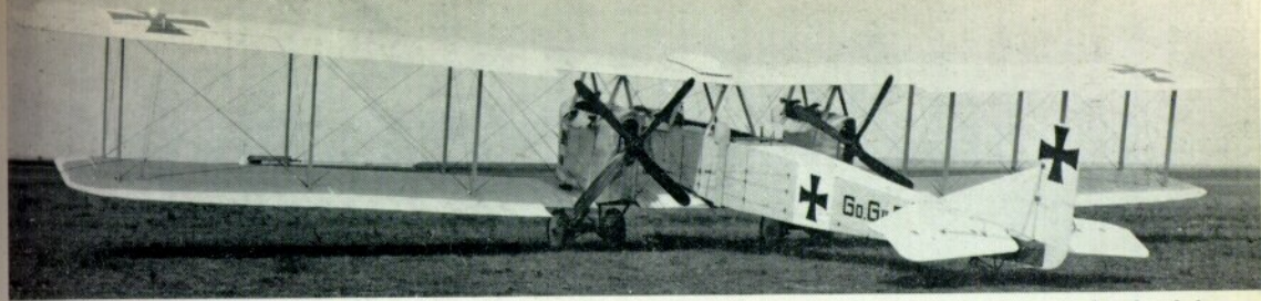
Gotha G.II 204/16 production version here fitted with four-bladed propellers. The paddle-shaped guards on each side of the rear cockpit protected the gunner from debris kicked up by the wheels and flung inboard by the propeller, and also prevented the gunner from accidentally leaning into the aircrew arc. The aircraft is covered with unbleached fabric, note contrast with white field of the crosses.
