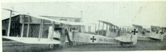
Gotha G.II's 203/16, 205/16 and 200/16 lined up in front of the Gotha factory. The massive two-bladed propeller was characteristic of the Mercedes D.IV geared engine.
