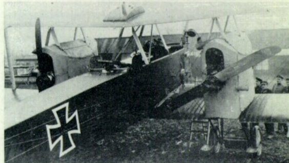
Left: Interested pilots of Jasta 4 examine Gotha G.III 397/16 at Marchais in May 1917. The slim fuselage and Cellon windows on the side of the front cockpit are here evident. Right: G.III 397/16; the passageway on the right side of the fuselage connects the front and rear cockpit; the rear gun is mounted on a lateral slide rail; and mudguards on the wheels prevent stones being thrown into the propeller arc. (Photos: W. Puglisi)
