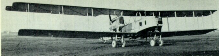
Below left: Gotha G.V modified to test simplified undercarriage structure. (Photo: von Röm)
