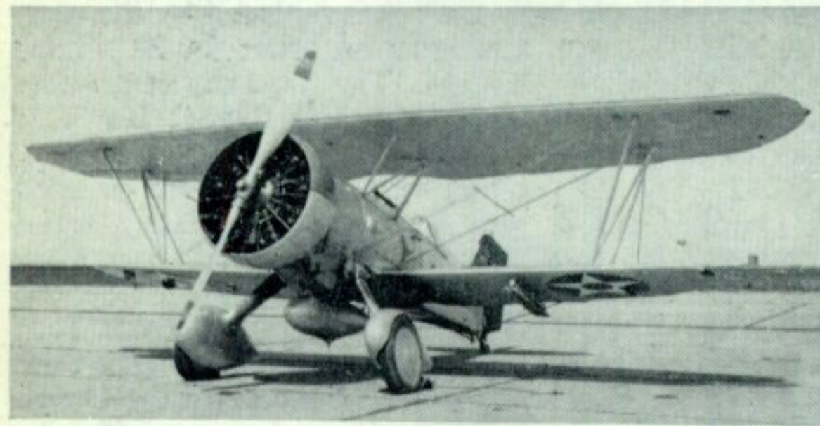
Left: The F11C-2's were redesignated BFC-2 in 1934. Note wing bomb racks and bomb-like auxiliary fuel tank on this aircraft. (Photo: E. M. Sommerich Collection). Right: Compare cockpit and aft fuselage details of BCF-2 with F11C-2. Squadron VF-1B was redesignated and became VB-2, still with red tail and the high hat insignia. (Photo: John C. Mitchell)
