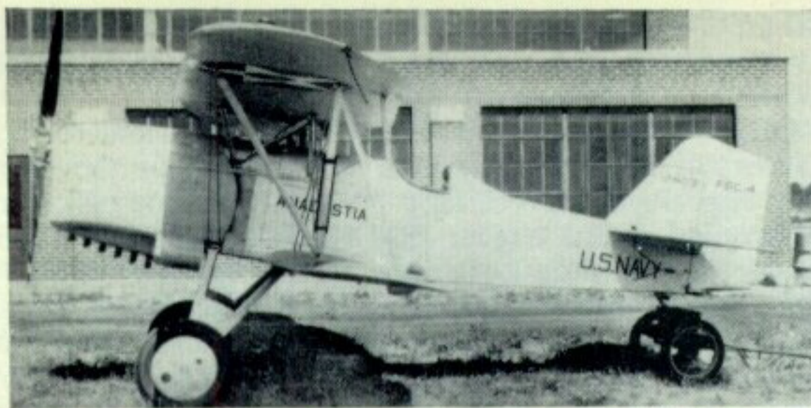
Left: The XF7C-1 was F6C-4, A-7403, fitted with an inverted air-cooled Ranger V-12 engine. (Photo: N.A.C.A.). Right: The 1932 version of the Hawk was sufficiently different to justify a new model number. This is XF11C-1 Navy Serial No. 9219. (Photo: U.S. Navy)
