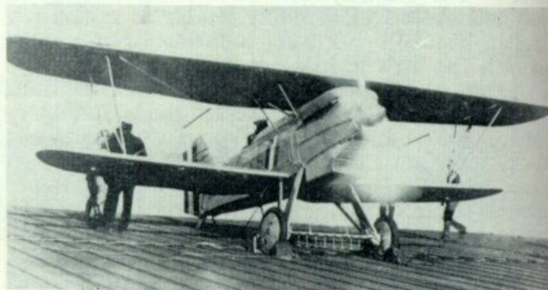
Left: The 7th F6C-1, A-6974, converted to F6C-2, a replacement leader of VF-2. Note new undercarriage and fuselage bomb rack. Right: F6F-2 A-6973 aboard U.S.S. Langley. Note undercarriage spreader bar and guide hooks. (Photo: U.S. Navy)
