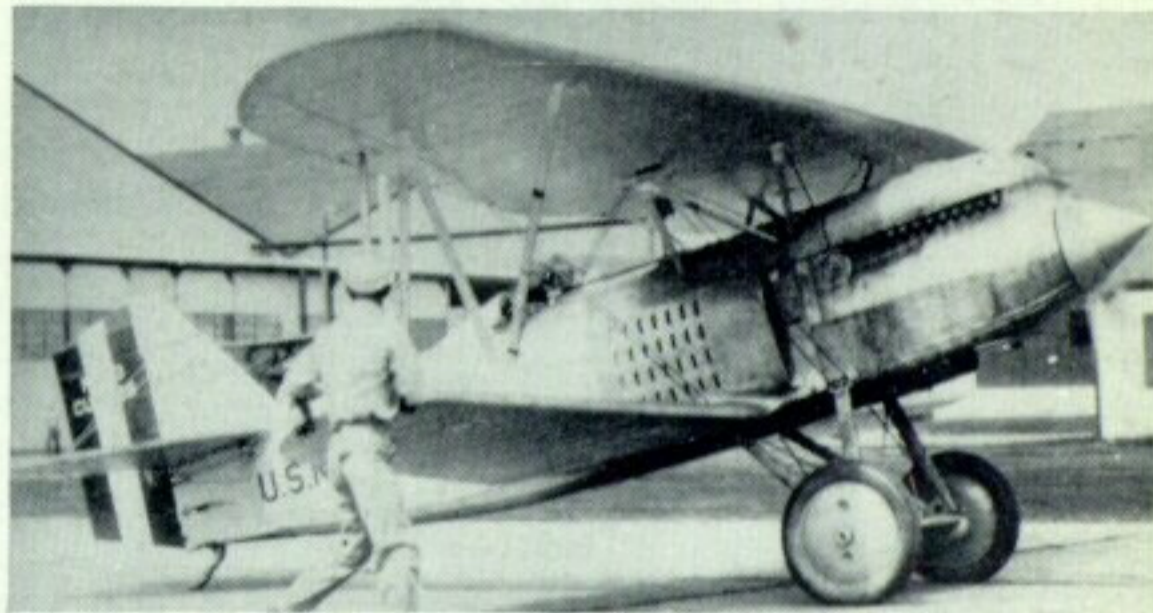
F6C-3 A-7114 modified for racing with radiator inside fuselage, low-drag undercarriage, and rear fuselage and belly rounded out with superstructure. (Photo: U.S. Navy)
