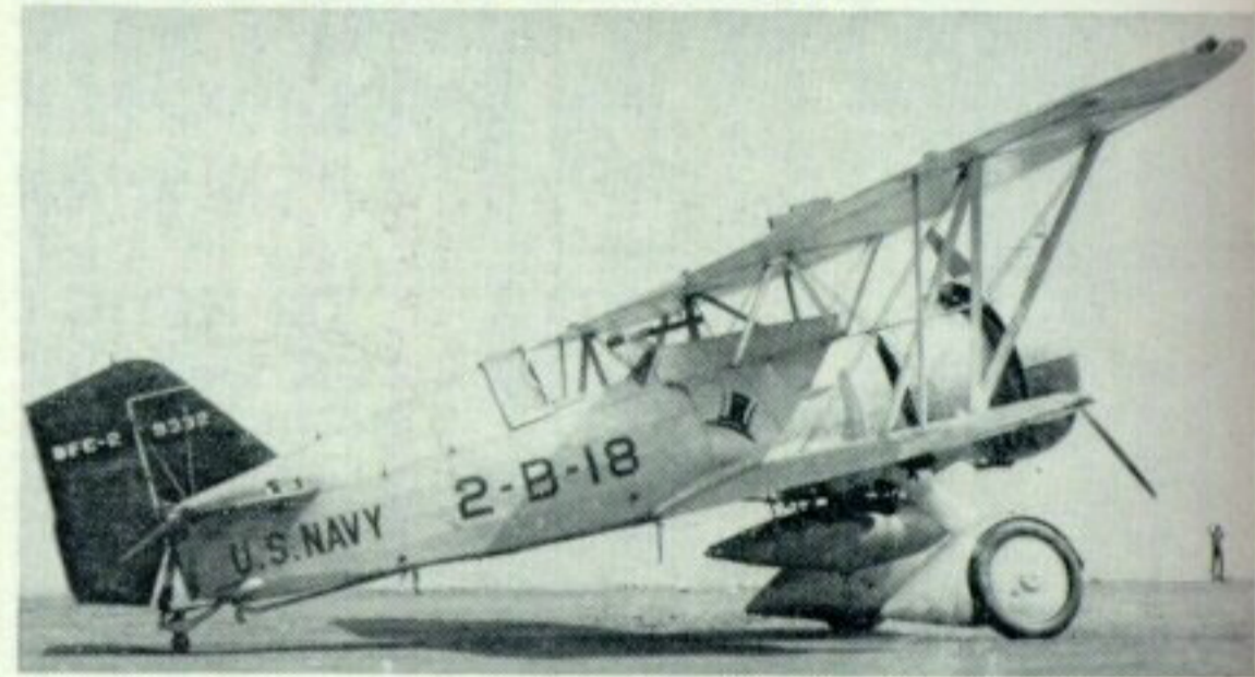
Left: The F11C-2's were redesignated BFC-2 in 1934. Note wing bomb racks and bomb-like auxiliary fuel tank on this aircraft. (Photo: E. M. Sommerich Collection). Right: Compare cockpit and aft fuselage details of BCF-2 with F11C-2. Squadron VF-1B was redesignated and became VB-2, still with red tail and the high hat insignia. (Photo: John C. Mitchell)
