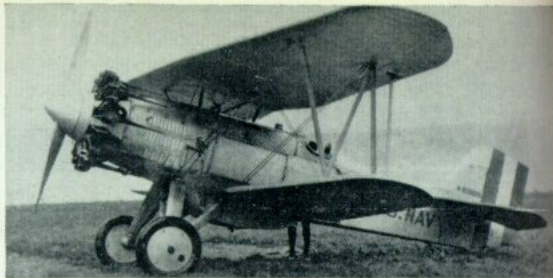
The first F6C-1, A-6968, after installation of P & W "Wasp" radial engine and redesignation as F6C-4. Note spinner, bayonet exhaust stacks, and large belly tank. (Photo: Arthur E. Price)
