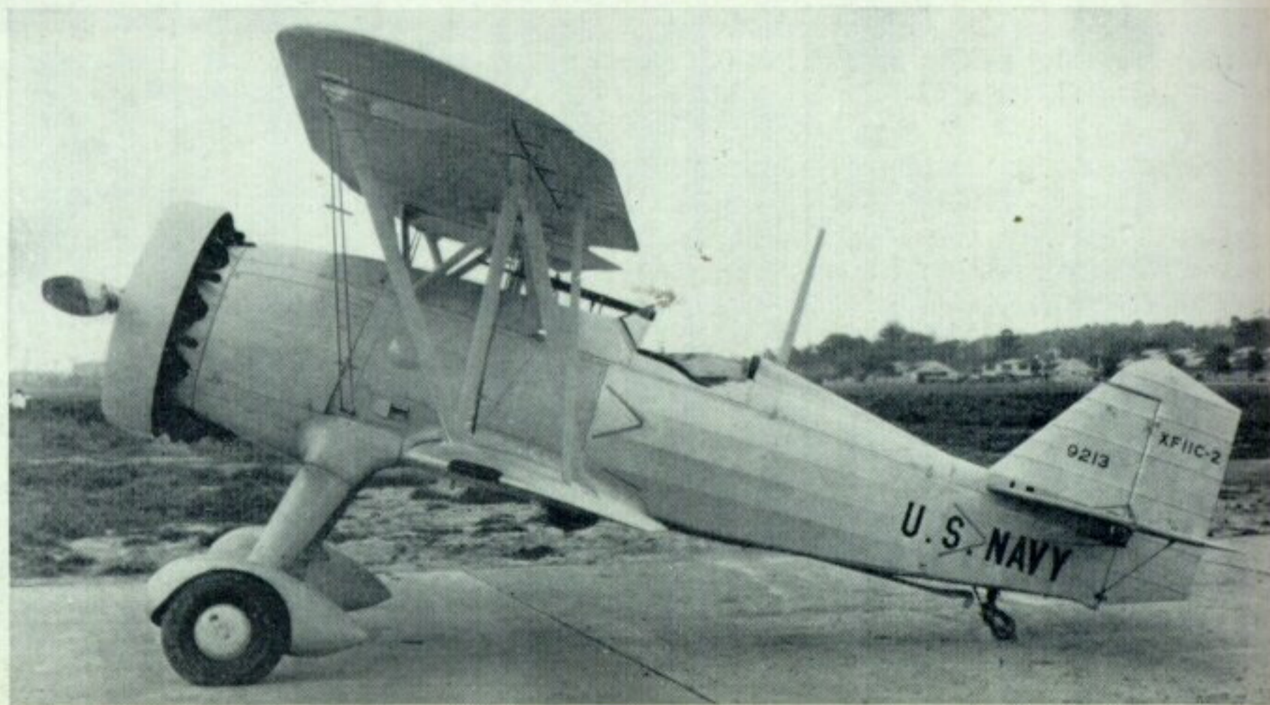
Although carrying a later designation but earlier serial number, 9213, the XF11C-2 was an older airplane than the XF11C-1. Note longer undercarriage legs.
