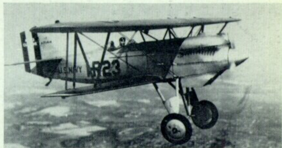
F6C-3 A-7144 restored to near-standard configuration with -4 undercarriage, circa 1930. Only the rounded rear fuselage contours remain from its racing days. (Photo: U.S. Navy)
