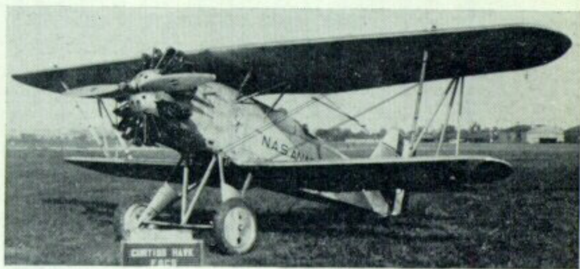
After becoming F6C-4 by engine change, the first F6C-1, A-6968, became the XF6C-5 when a P & W "Hornet" engine and production F6C-4 undercarriage were installed in 1927. (Photo: U.S. Navy)
