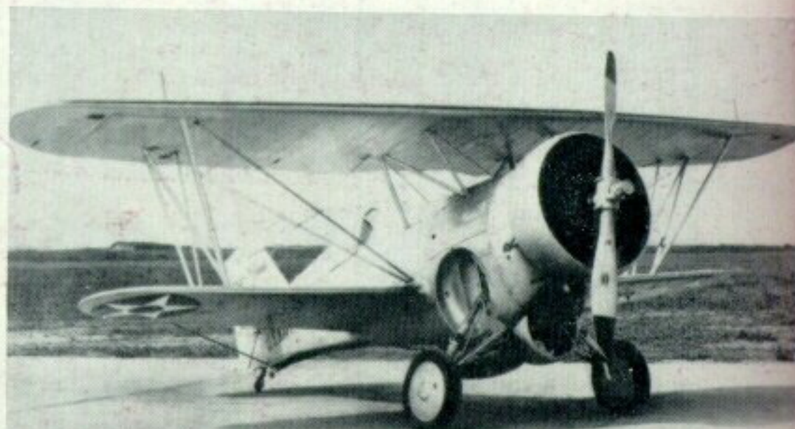
The XF11C-3 with controllable propeller and modified fuselage after redesignation as XBF2C-1. (Photo: U.S. Navy)
