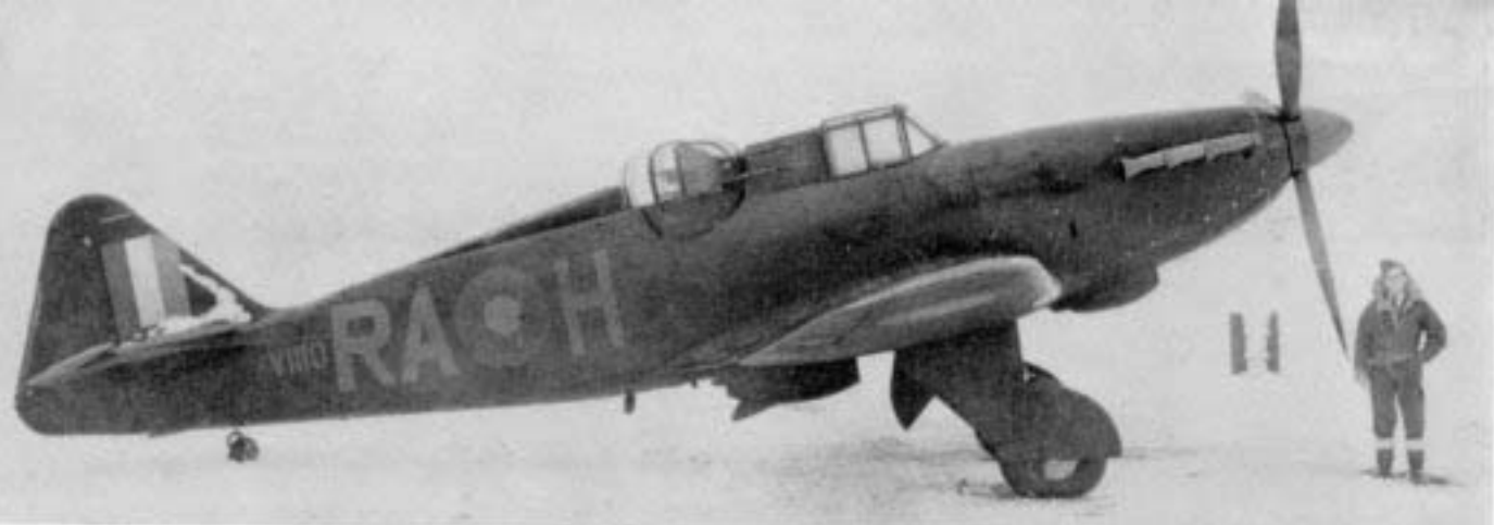
V1110, RA-H of No. 410 (R.C.A.F.) Squadron, photographed in January 1942. The machine is finished in RDM2 super-matt black overall, with red-blue roundels in all positions. This aircraft was later converted to T.T. Mk. III configuration.
