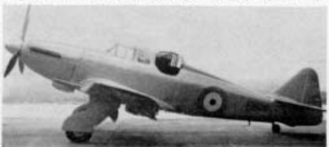
Left: The second prototype, K8620, with telescopic radio masts, modified undercarriage cover plates, and a rear-view window added on each side of the canopy. Right: The only Defiant competitor to fly, the Hawker Hotspur. (Photo: Imp. War Mus. HU 2171)
