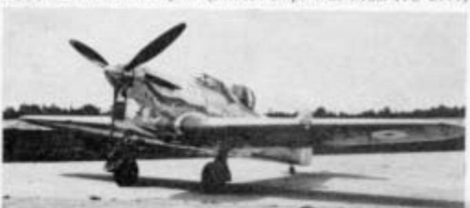
Left: The second prototype, K8620, with telescopic radio masts, modified undercarriage cover plates, and a rear-view window added on each side of the canopy. Right: The only Defiant competitor to fly, the Hawker Hotspur. (Photo: Imp. War Mus. HU 2171)
