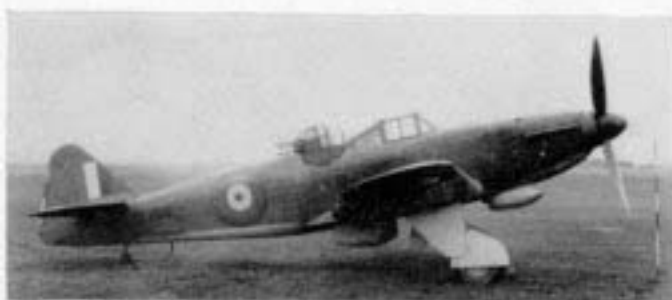
N1551 with the retractable fuselage sections lowered for firing. (Photo: Imp. War Mus. MH 5988)
