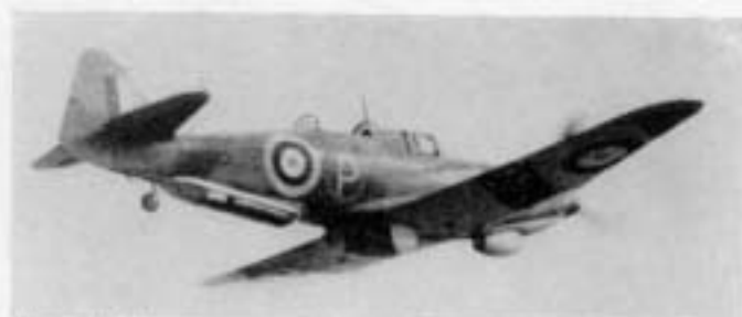
Note the drogue storage box under the rear fuselage of DR863, the T.T. Mk. I prototype.
