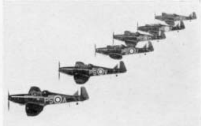
In this formation of Defiants from No. 264 Sqn., three distinct types of fuselage roundel are visible; compare aircraft 'A', aircraft 'Z' and aircraft 'U'. (Photo: Imp. War Mus. CH 888)
