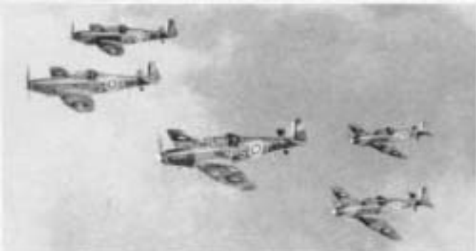
Five 264 Sqn. Defiants in flight, all apparently bearing patches over recent combat damage; note the two camouflage schemes. Aircraft 'A' and 'T' are finished in a scheme which mirrors that of 'X', 'D' and 'V'. (Photo: Imp. War Mus. CH 877)
