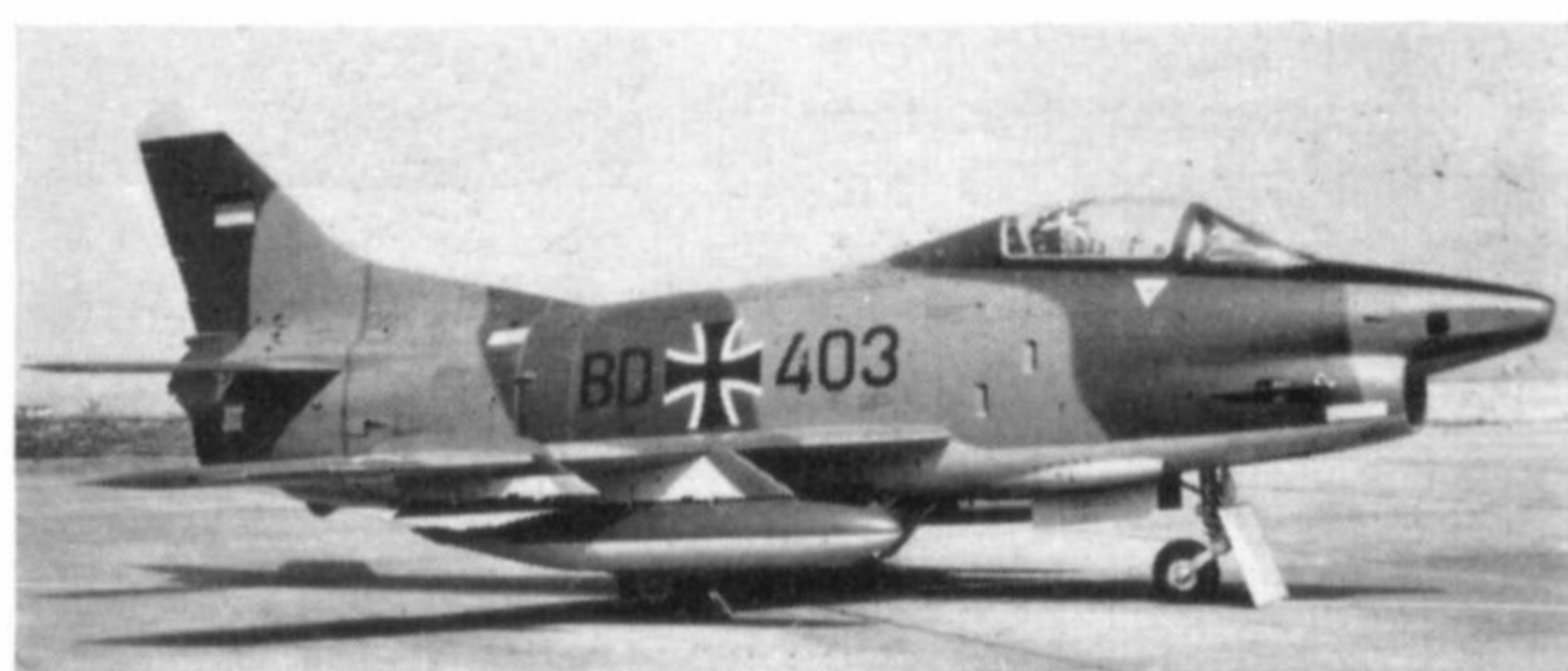
A G.91R-3 of the Luftwaffe's Waffenschule 50; note protruding barrel of 30 mm. cannon, and underwing stores.
