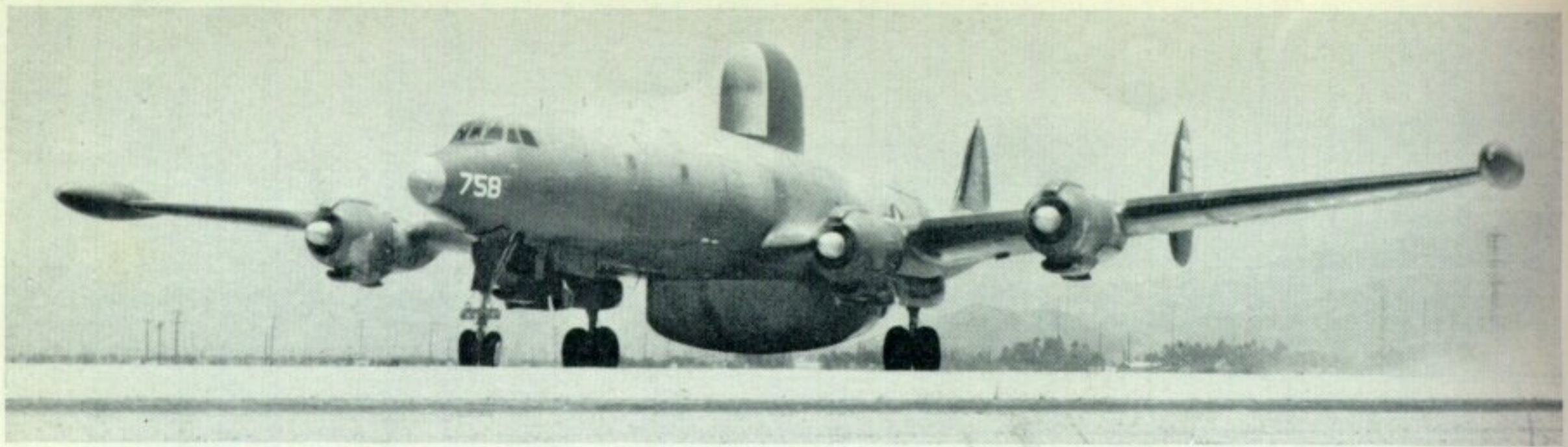
A Pacific Missile Range "Willy Victor" EC-121D takes off from Pt. Mugu on a frequency interference control mission prior to a satellite launching. This study gives an impression of the massive radar bays. (Photo: U.S.N. via Bulban)
