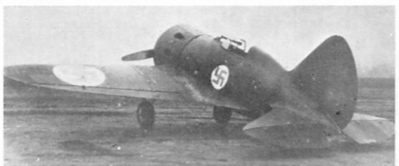
Above and below: IR-101, another machine captured by the Finns, displays the fixed, braced undercarriage sometimes used by training and liaison I-16's. This aircraft appears to be finished in the "Continuation War" scheme of forest green/black-green shadow shading and deep yellow fuselage band.
