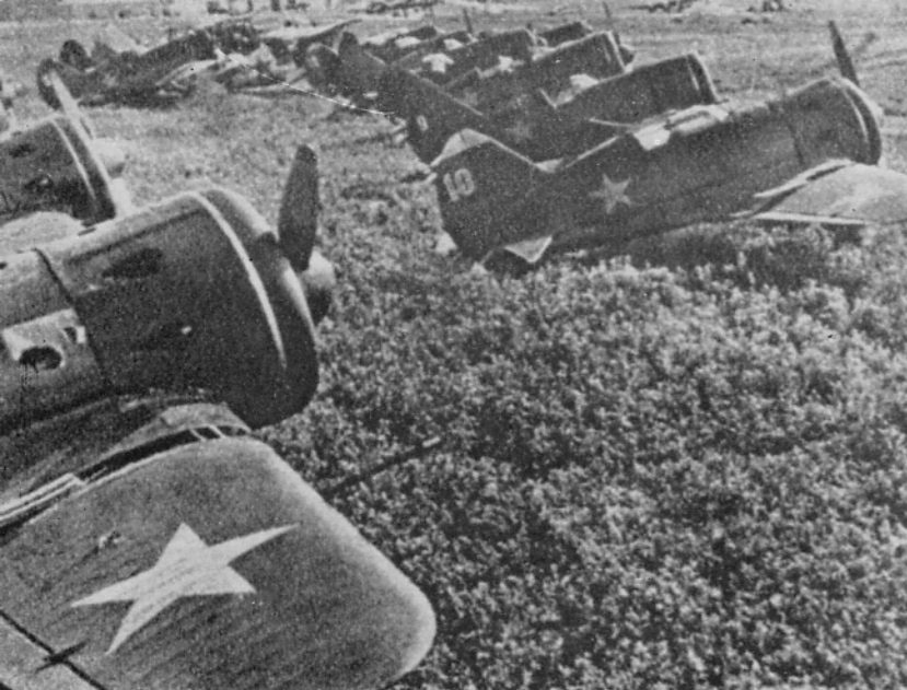
I-16's and I-15's, apparently captured on the ground or abandoned in the face of the German advance. Note battle damage to nearest aircraft; these are Type 10's.
