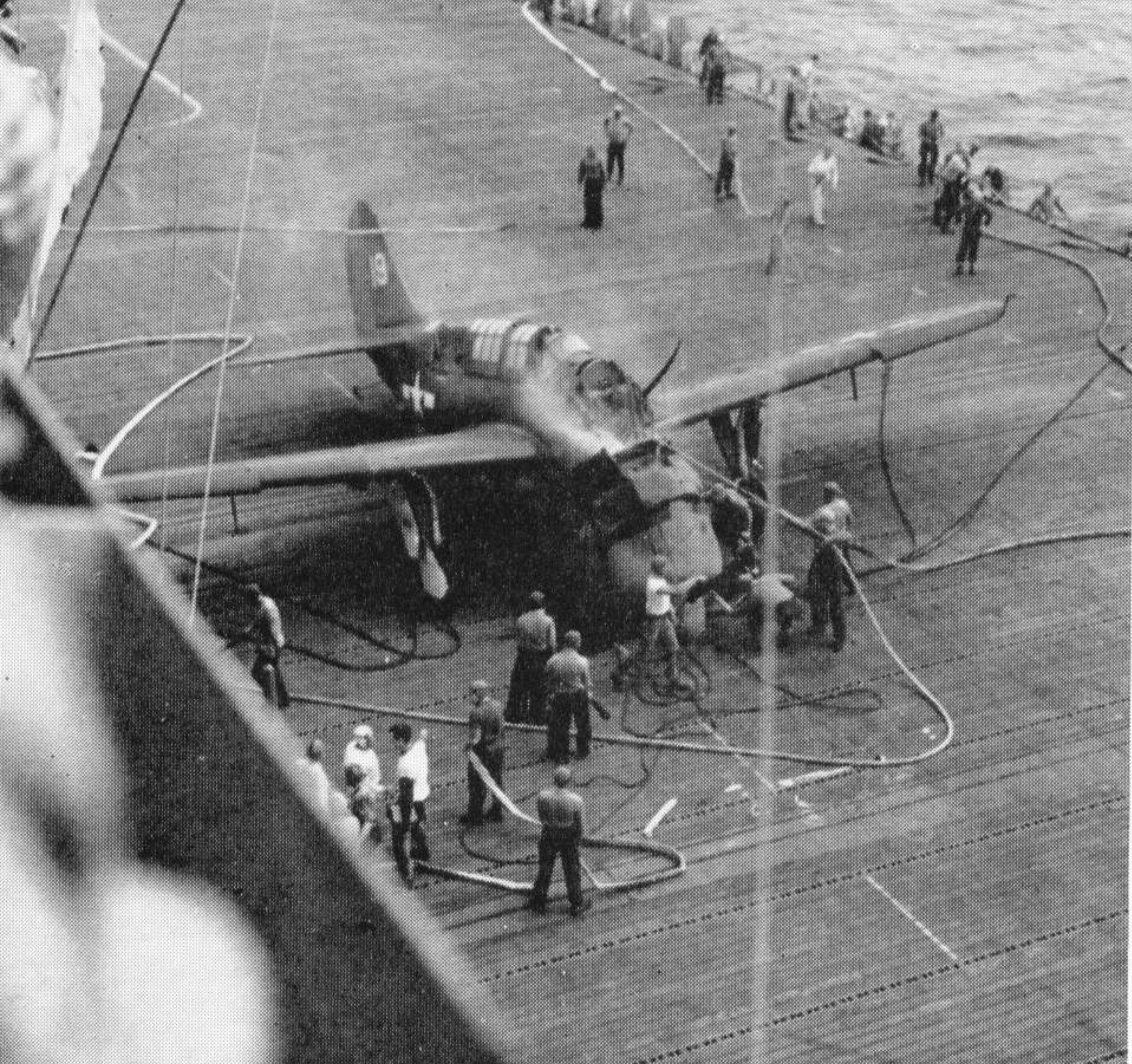
SB2C-1C of VB-15 loses its engine in a barrier crash on the Essex (CV-9) after returning from a mission in the Philippine Sea battles. (Photo: U.S.N./National Archives)
