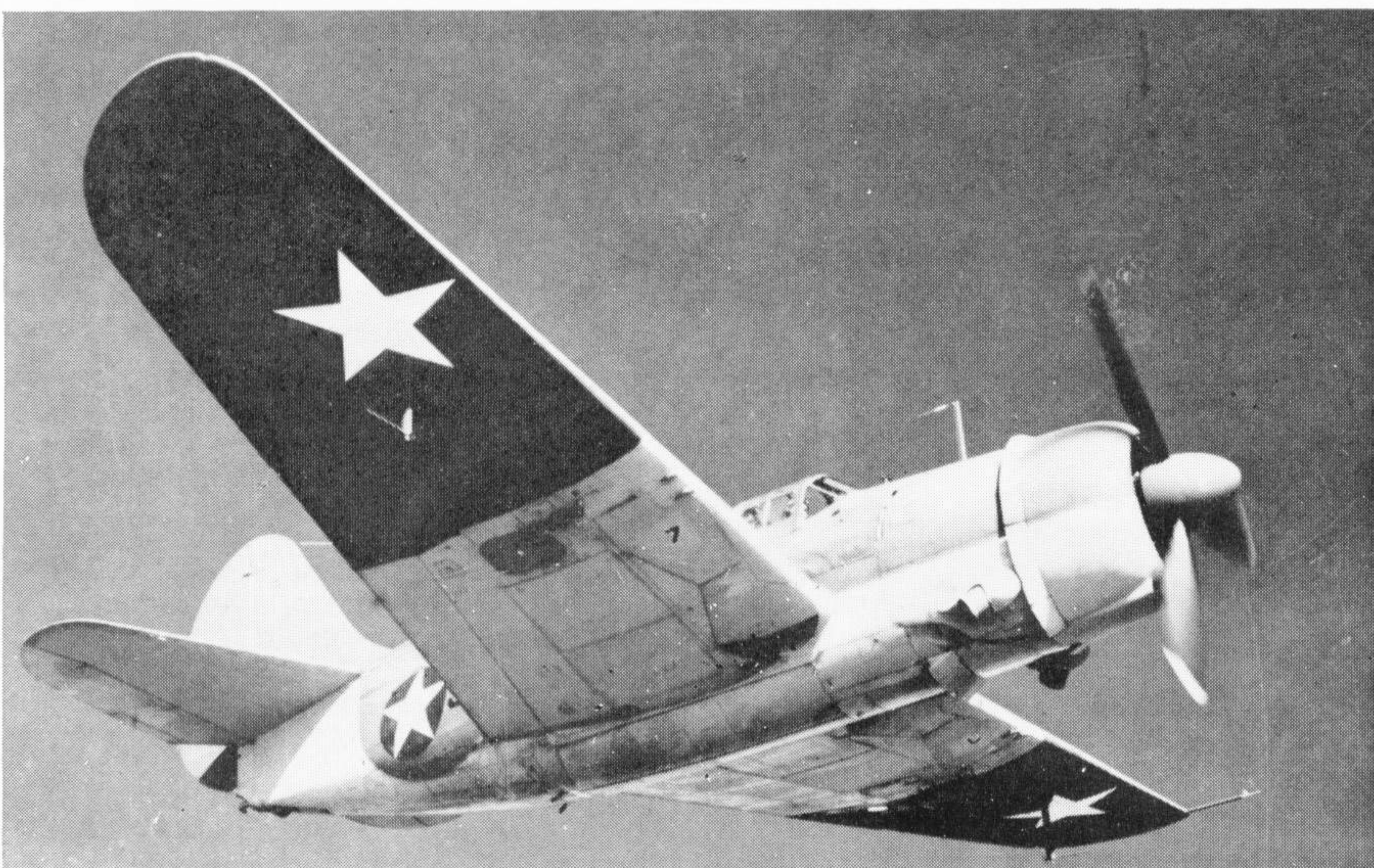
BuNo 00018 shown in flight, shortly after issue to VS-9 at NAS Norfolk, Virginia in November 1942. The company-painted number is visible on the fin; note also retracted tail wheel and ASB Yagi antennae under the wings.
